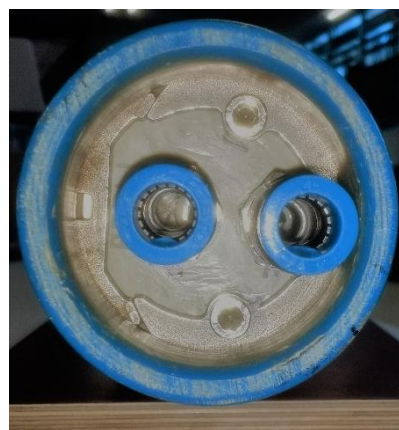
Figure 15. The bearing plate on the permeate-concentrate side of the pressure vessel.
