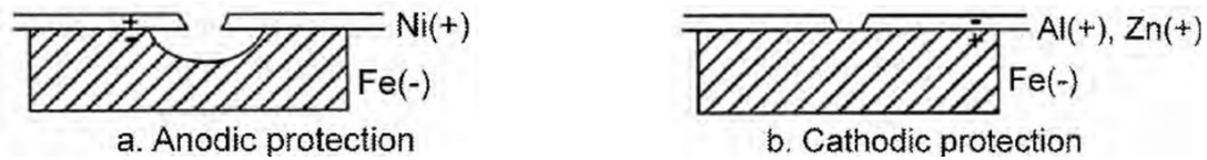
Figure 2.24: (a) Anodic protection with non-sacrificial coating (b) Cathodic protection with sacrificial coating [85]
