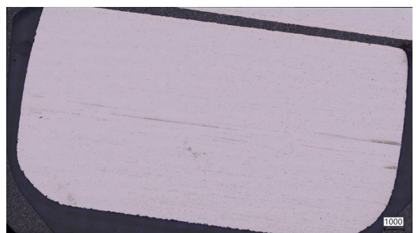
Figure D.6: Stitched micrograph of immersed sample with 250 µm coating
