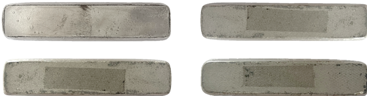
Figure 4.22: Photographs of immersed samples, from left to right: without coating, 250, 375 and 500 \mu\text{m}
