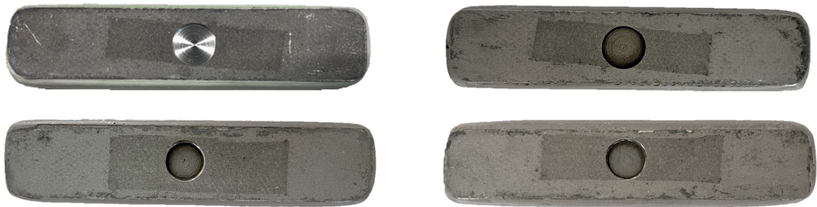
Figure 4.28: Photographs of immersed galvanic corrosion samples, from left to right: 250 μm before immersion, 250, 375 and 500 μm
