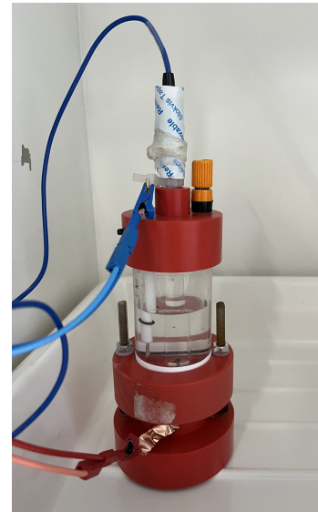
Figure 3.12: Actual electrochemical cell setup
