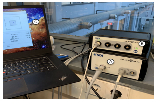
Figure 4.11: (A) Aurora ® System Control Unit; (B) Sensor Interface Unit; (C) the host computer.
