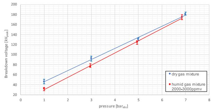
Fig. 10. Breakdown strength of C<sub>4</sub>-FN with different humidities in a uniform electric field against increasing operating pressures.
