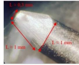
Fig. 1. Dimensions of the tungsten needle.
