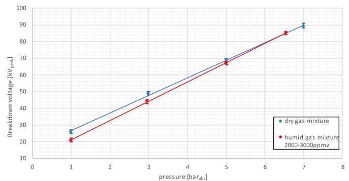
Fig. 11. Breakdown strength of C<sub>4</sub>-FN with different humidities in a quasi-uniform electric field against increasing operating pressures.
