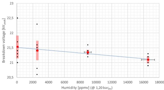
Fig. 9.  $U_{50}$  of C<sub>4</sub>-FN in a nonuniform electric field.
