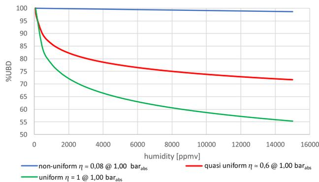
Fig. 17. Rough comparison between the relative ac breakdown strength of the three examined electric field configurations.
