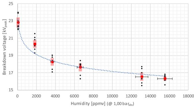
Fig. 8.  $U_{50}$  of C<sub>4</sub>-FN in a quasi-uniform electric field.
