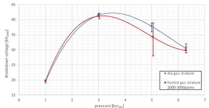
Fig. 12. Breakdown strength of C<sub>4</sub>-FN with different humidities in a nonuniform electric field against increasing operating pressures.
