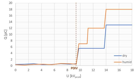
Fig. 13. Measured average charge at different voltages.  $Q$  [pC] is the averaged charge according to the IEC60270.
