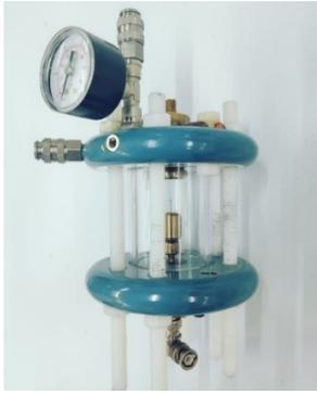
Fig. 3. Photograph of the test cell to examine the PD behavior of corona. The test cell is PD free up to 40 kV<sub>peak</sub> and is of the same size as Fig. 2(b).
