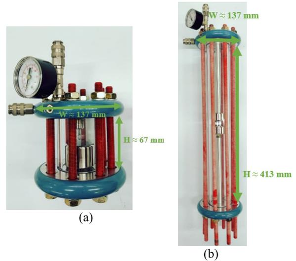
Fig. 2. Photograph of the two test cells used during this research. (a) Small test cell with a total length of ca. 12 cm. (b) Large test cell with a total length of ca. 47 cm. Radius of blue top and bottom electrode is 12 mm.
