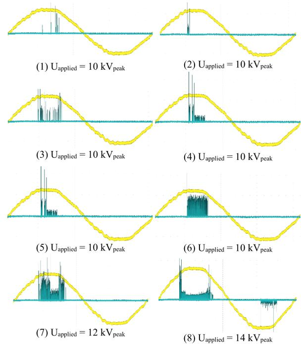
Fig. 14. Eight screenshots (interval of 60 s) of the oscilloscope PRPD pattern in dry C<sub>4</sub>-FN. Yellow = applied voltage. Blue = corona PDs.
