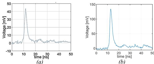
Fig. 16. (a) Waveform of a corona PD in dry C<sub>4</sub>-FN. (b) Waveform of a corona PD in humid C<sub>4</sub>-FN.
