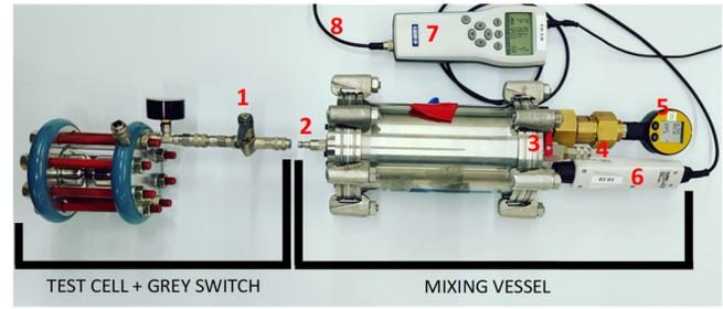
Fig. 4. Test setup used to create a humid C<sub>4</sub>-FN gas mixture. 1 = removable gray switch; 2 = male DILO outlet of the mixing vessel; 3 = red switch to give more control over the inlet of the mixing vessel; 4 = female DILO inlet of the mixing vessel; 5 = digital pressure sensor (up to two decimals); 6 = humidity probe DMP74B; 7 = handheld dewpoint meter DM70; and 8 = data connection between probe and meter.
