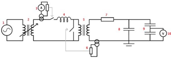
Fig. 5. Test setup for examining the ac breakdown behavior of the  $C_4$ -FN gas mixture. 1 = fixed power source 19 kVA and 50 Hz; 2 = variac; 3 = overcurrent protection; 4 = step up transformer; 5 = 50-k $\Omega$  current limiting resistor; 6 = ac/dc voltage probe; 7 = multimeter; 8 = test cell; 9 = 50- $\Omega$  coaxial cable; 10 = overvoltage protection; and 11 = oscilloscope.
