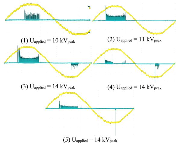
Fig. 15. Five screenshots (interval of 60 s) of the PRPD pattern in humid C<sub>4</sub>-FN. Yellow = applied voltage. Blue = corona PDs.
