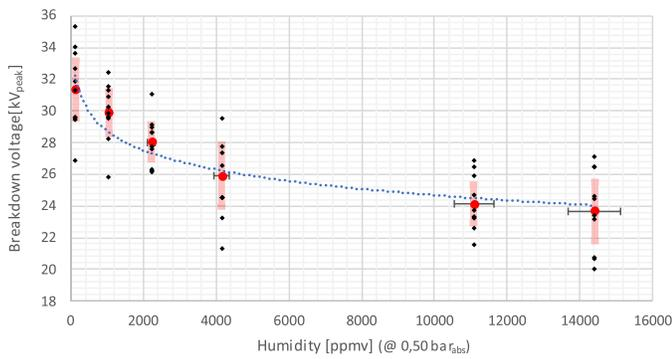
Fig. 7.  $U_{50}$  of C<sub>4</sub>-FN in a uniform electric field.
