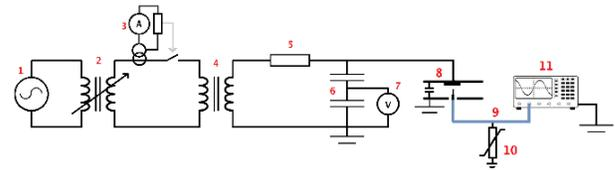
Fig. 6. Test setup for examining the corona PD behavior in the  $C_4$ -FN gas mixture. 1 = power socket; 2 = variac; 3 = overcurrent protection; 4 = step up transformer; 5 = 50-k $\Omega$  current limiting resistor; 6 = ac/dc voltage probe; 7 = multimeter; 8 = test cell; 9 = 50- $\Omega$  coaxial cable; 10 = overvoltage protection; and 11 = oscilloscope.
