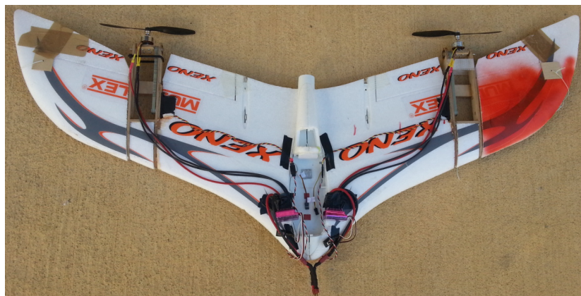
Figure 7. Xeno UNI form Multiplex with two customised tilt rotors.
