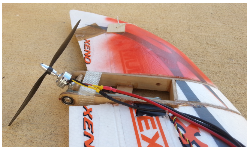
Figure 8. Tilt rotor mechanical structure.
