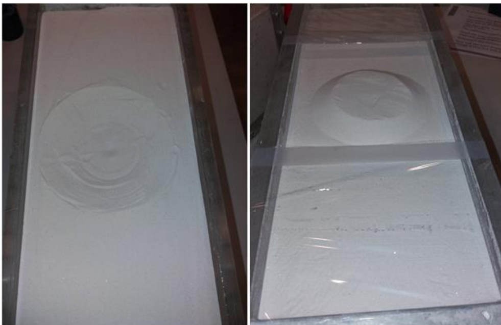
Figure 3.4 Samples prepared for the centrifuge tests, with scour formation (left) and with scour protection (right).
