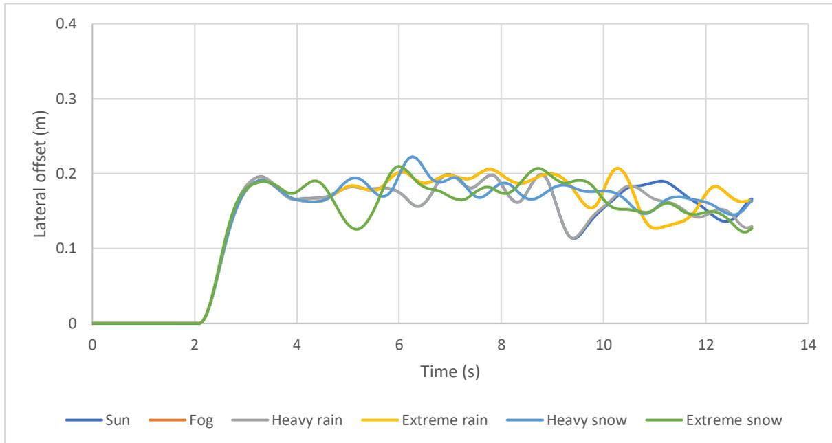
Figure 38: Lateral offset variation for different weather conditions at 2.6 m lane width, 750 m radius and 100 km/h
