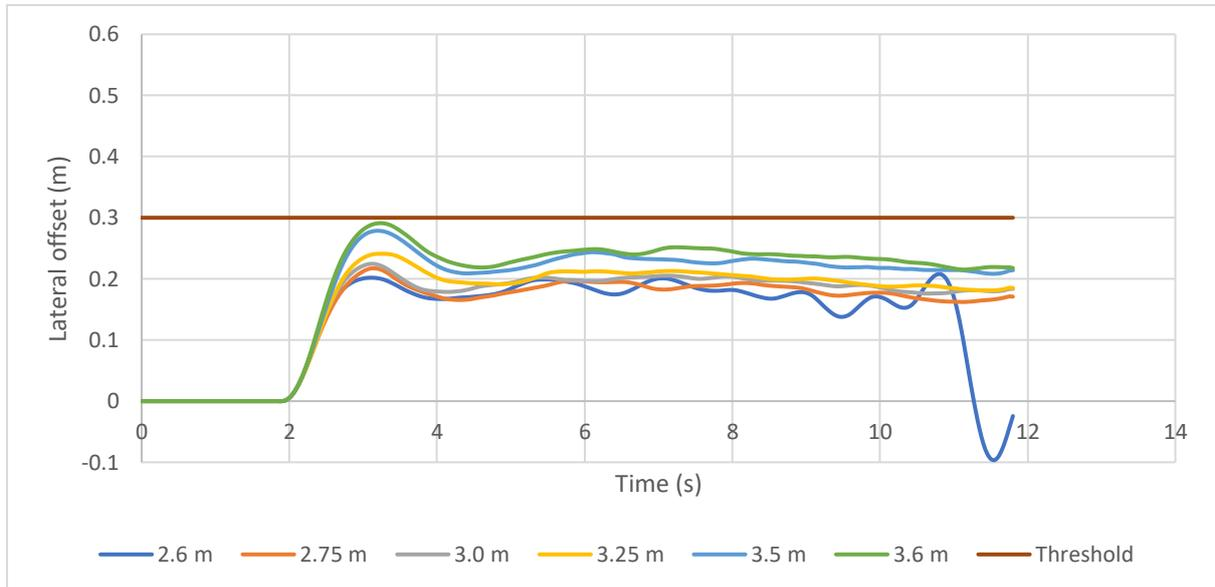
Figure 66: Lateral offset variations for test cases with 900 m radius and speed of 110 km/h
