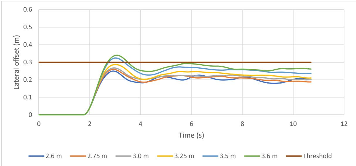
Figure 67: Lateral offset variations for test cases with 900 m radius and speed of 120 km/h
