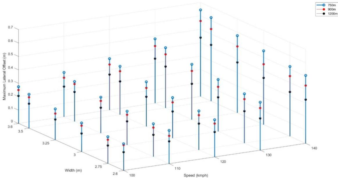
Figure 49: Maximum lateral offset variations of test cases without precipitation
