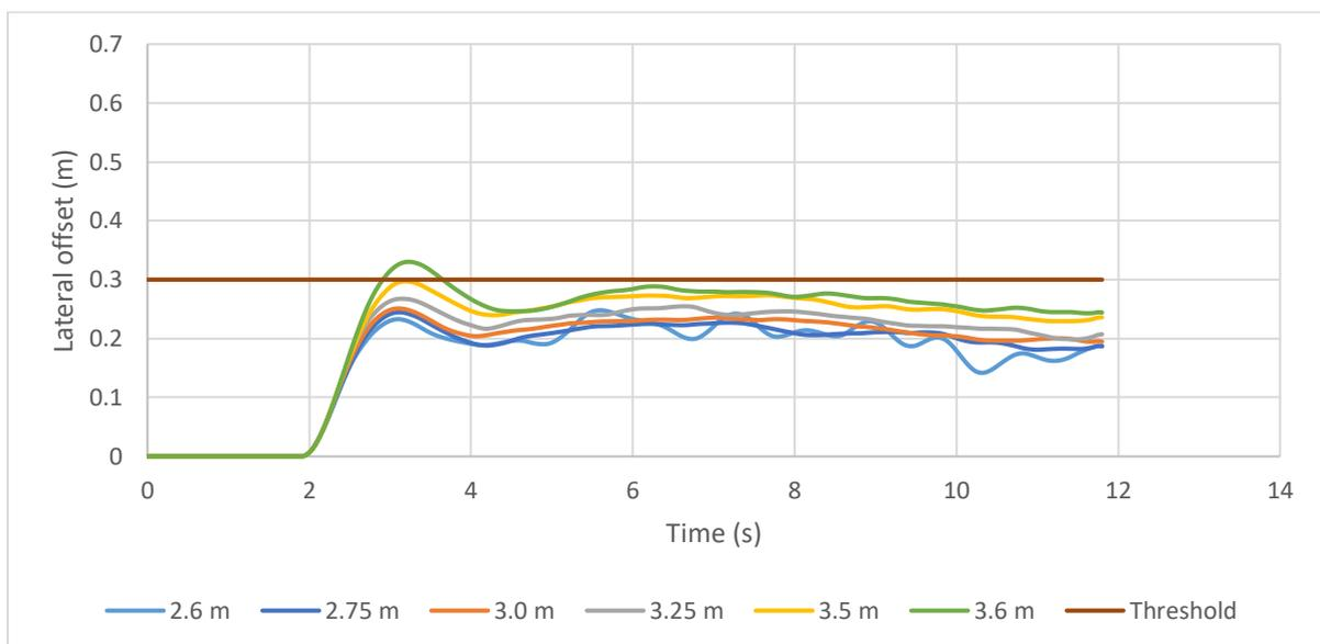
Figure 61: Lateral offset variations for test cases with 750 m radius and speed of 110 km/h
