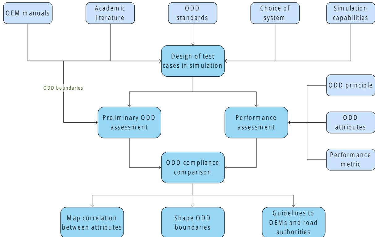
Figure 55: Conceptual framework to test the ODD boundary of ADAS in simulation
