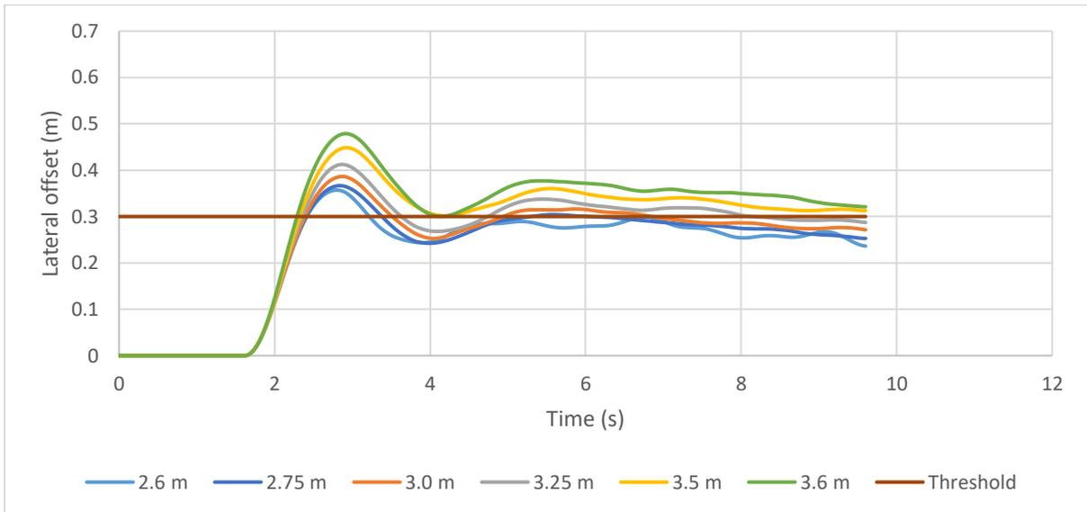
Figure 63: Lateral offset variations for test cases with 750 m radius and speed of 130 km/h
