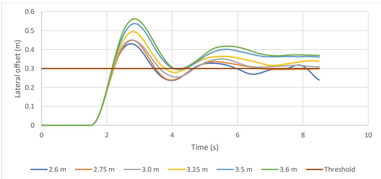
Figure 69: Lateral offset variations for test cases with 900 m radius and speed of 140 km/h
