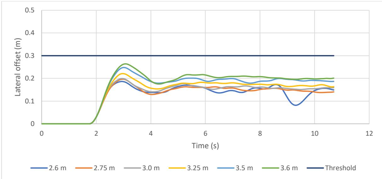
Figure 72: Lateral offset variations for test cases with 1200 m radius and speed of 120 km/h
