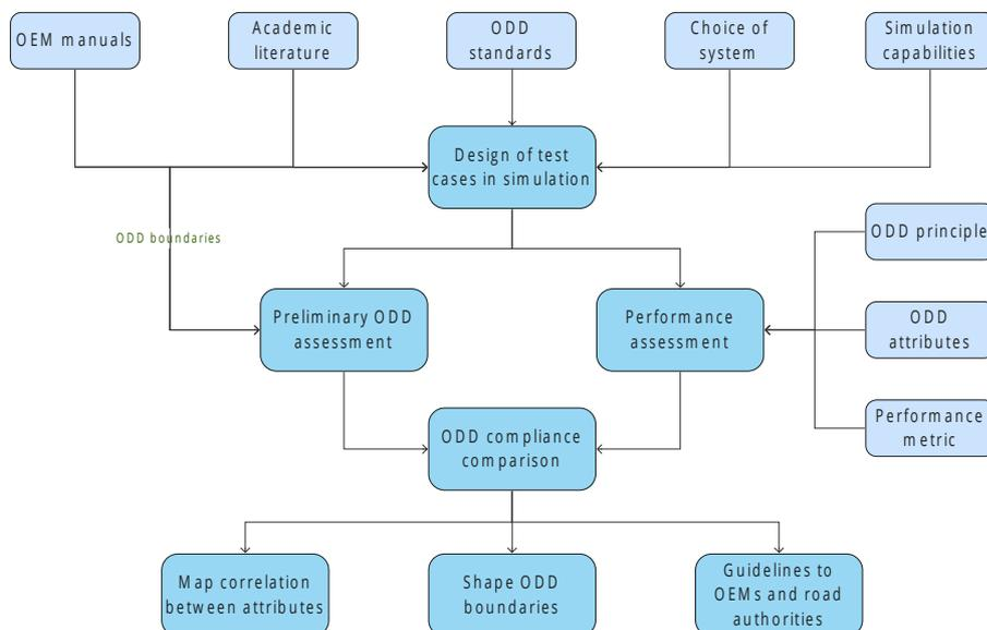
Figure C: Proposed framework to assess the ODD of an ADAS feature in simulation
