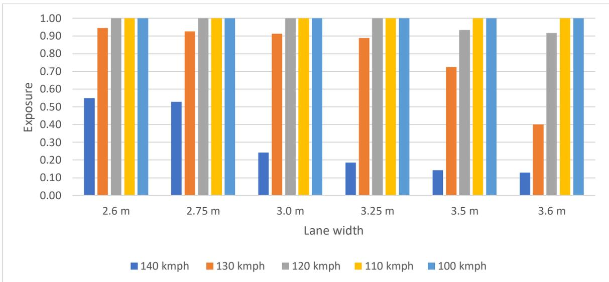
Figure 27: Exposure data comparison between different lane widths and speeds for test cases of 900 m radius curve
