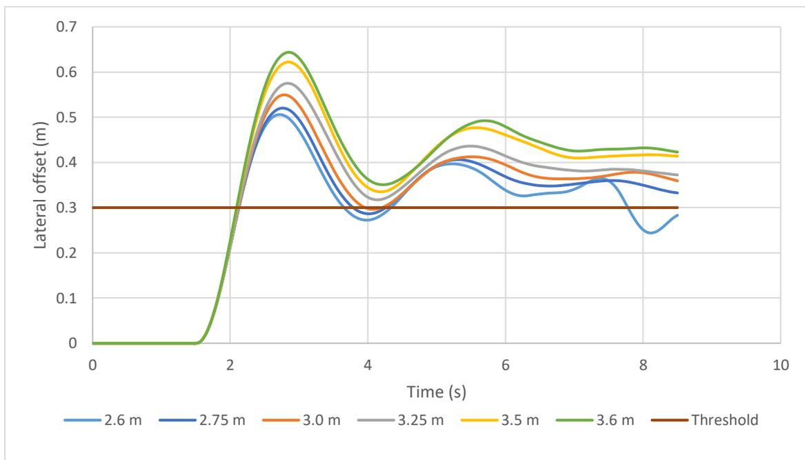
Figure 19: Lateral offset variation for different lane widths in 140 km/h and 750 m radius condition
