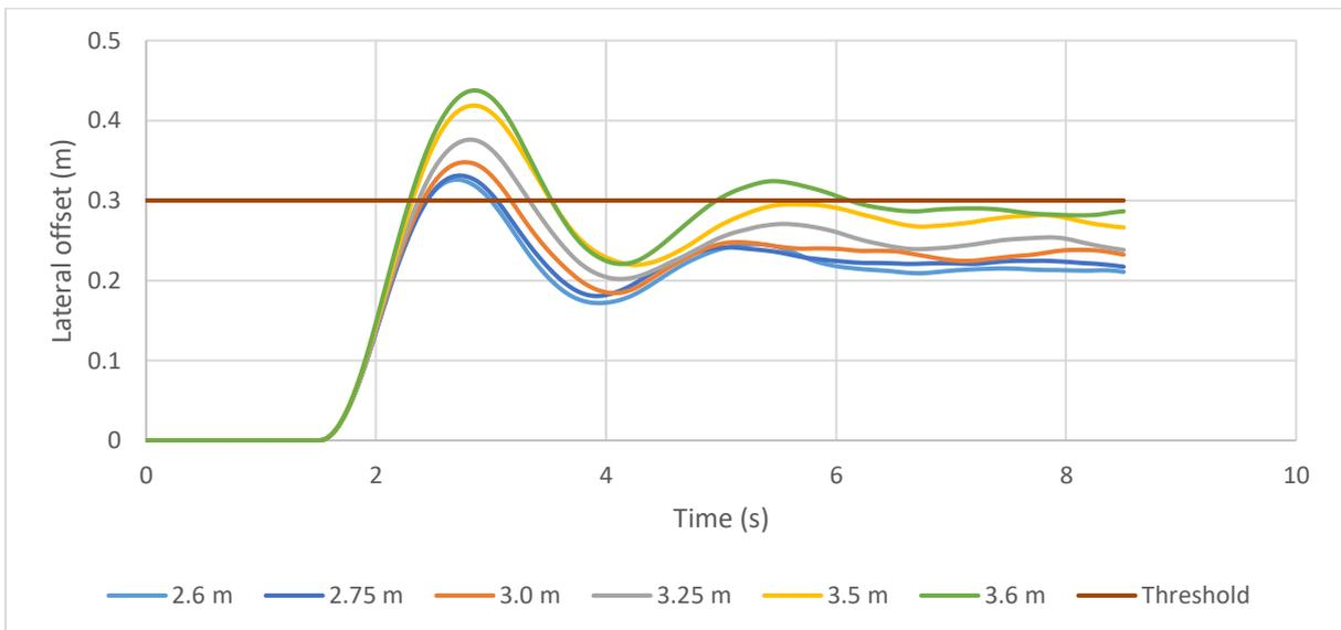
Figure 74: Lateral offset variations for test cases with 1200 m radius and speed of 140 km/h
