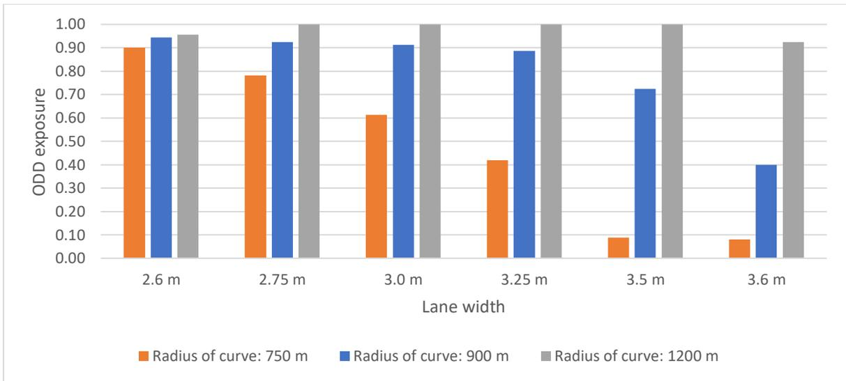
Figure 32: Exposure data comparison between different lane widths and radii for test cases of 130 km/h
