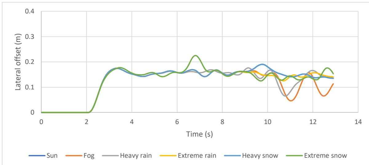
Figure 34: Lateral offset variation for different weather conditions at 2.6 m lane width, 900 m radius and 100 km/h
