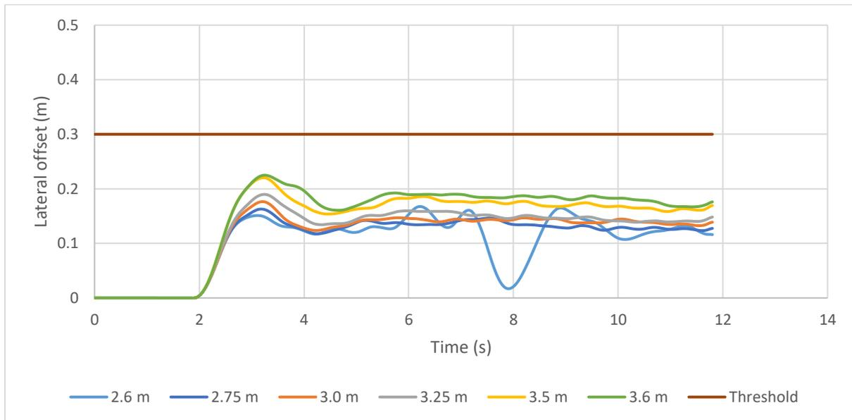
Figure 71: Lateral offset variations for test cases with 1200 m radius and speed of 110 km/h
