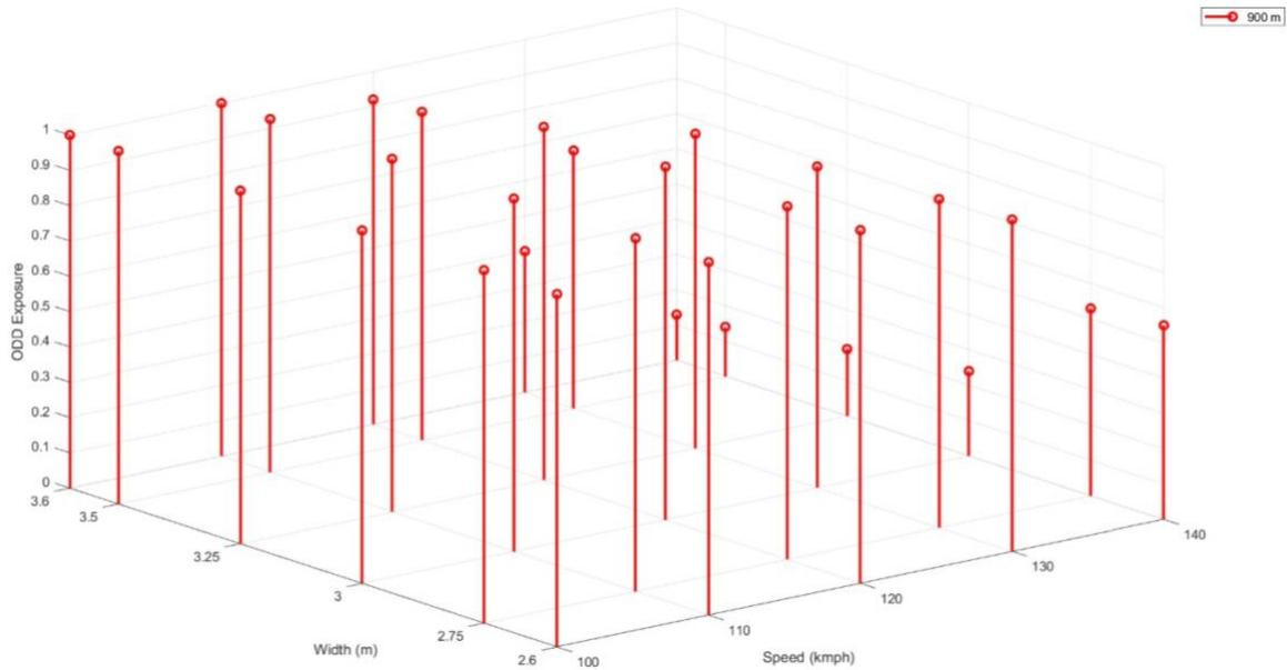
Figure 52: Exposure variations of all the test cases of radius 900 m without precipitation
