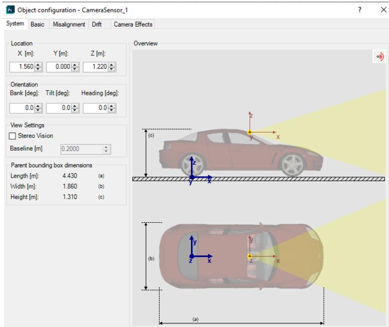
Figure 13: Camera sensor position on the test vehicle
