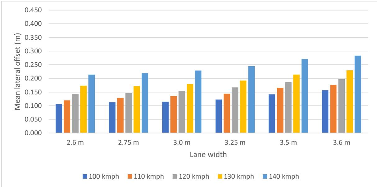
Figure 22: Mean lateral offset variations for 1200 m radius curve
