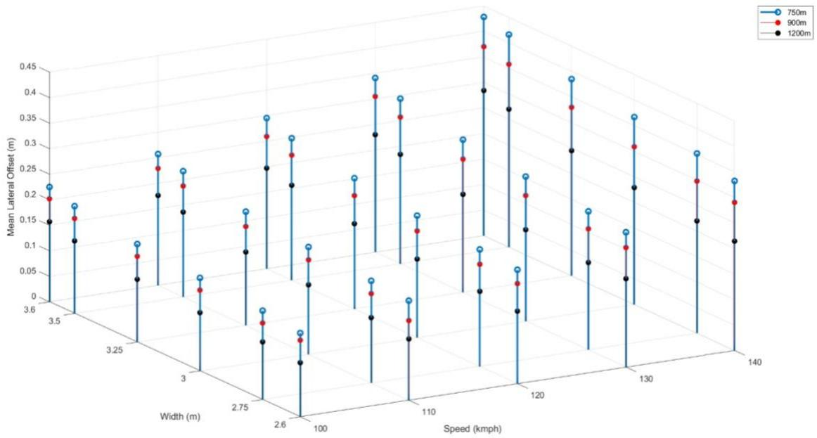
Figure 50: Mean lateral offset variations of test cases without precipitation
