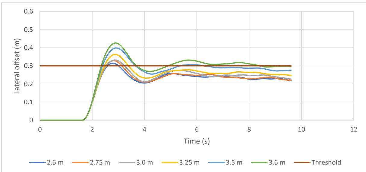
Figure 68: Lateral offset variations for test cases with 900 m radius and speed of 130 km/h
