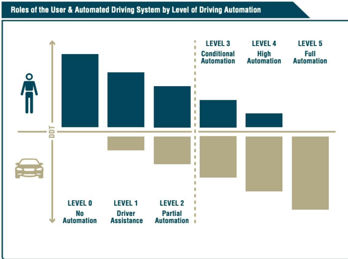
Figure 4: Roles of driver and system in SAE levels
