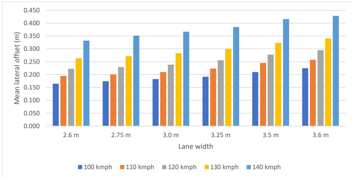
Figure 20: Mean lateral offset variations for 750 m radius curve
