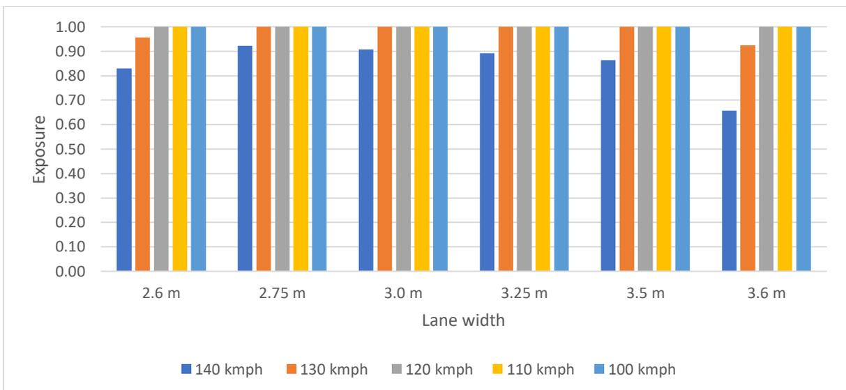
Figure 28: Exposure data comparison between different lane widths and speeds for test cases of 1200 m radius curve
