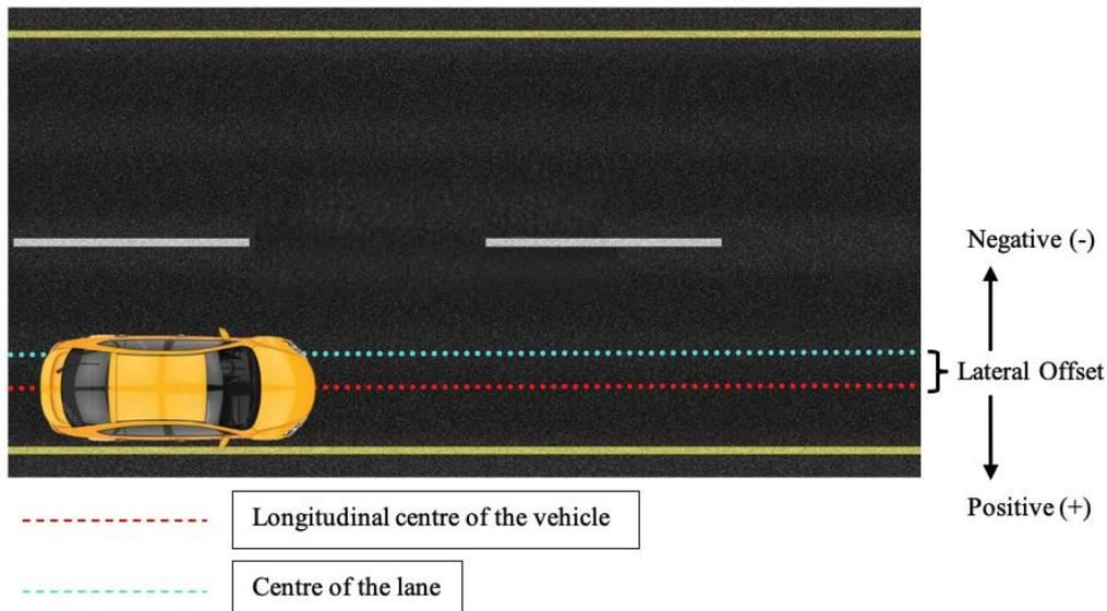
Figure 12: Measurement of lateral offset
