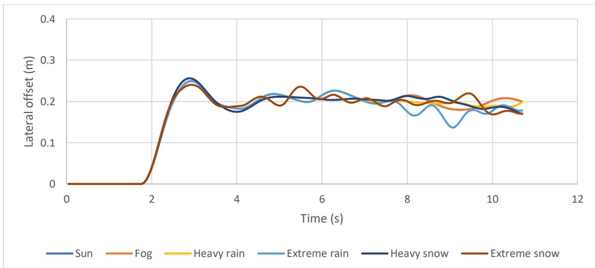
Figure 35: Lateral offset variation for different weather conditions at 2.6 m lane width, 900 m radius and 120 km/h
