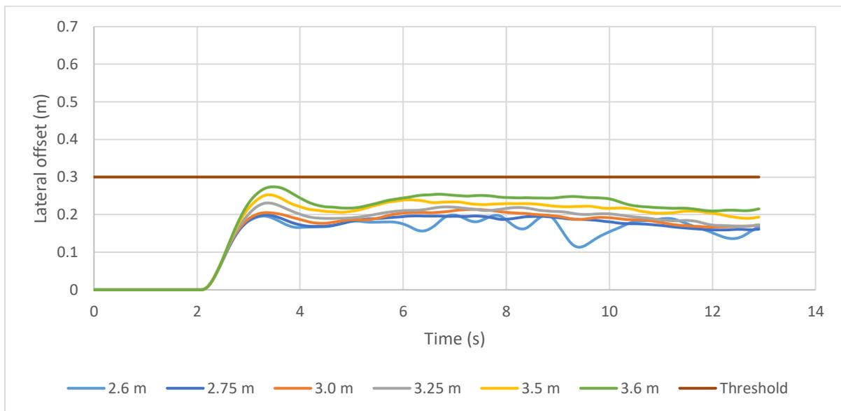
Figure 60: Lateral offset variations for test cases with 750 m radius and speed of 100 km/h
