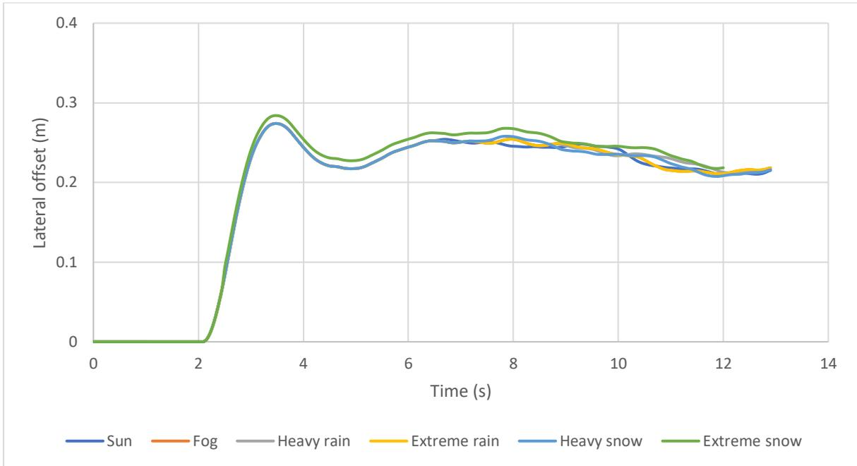
Figure 40: Lateral offset variation for different weather conditions at 3.6 m lane width, 750 m radius and 100 km/h
