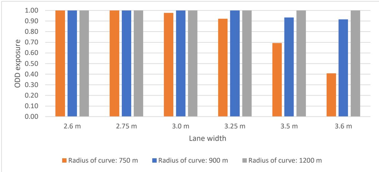
Figure 31: Exposure data comparison between different lane widths and radii for test cases of 120 km/h
