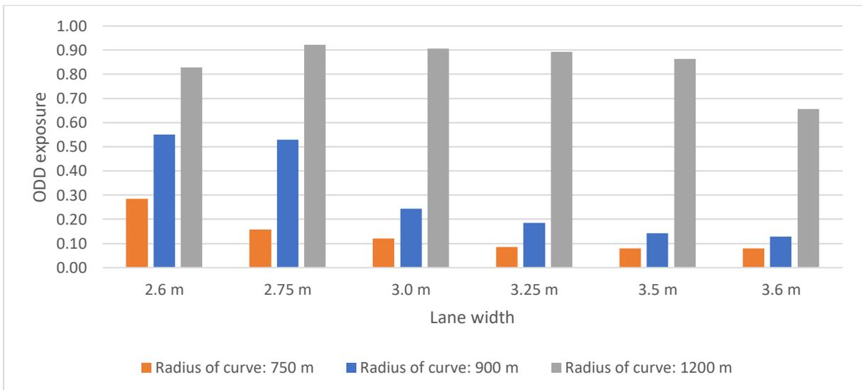
Figure 33: Exposure data comparison between different lane widths and radii for test cases of 140 km/h
