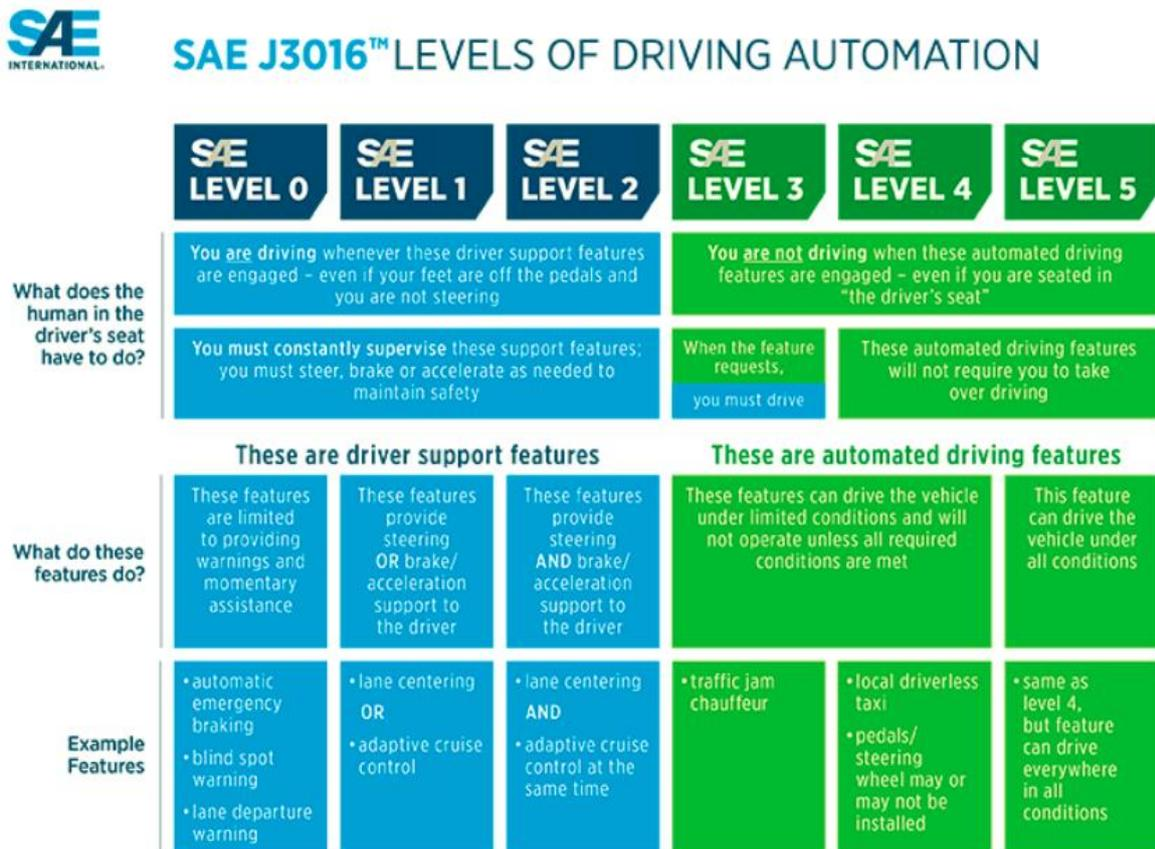
Figure 3: SAE levels of driving automation and functions
