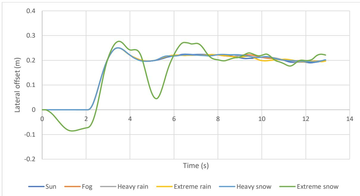
Figure 36: Lateral offset variation for different weather conditions at 3.6 m lane width, 900 m radius and 100 km/h
