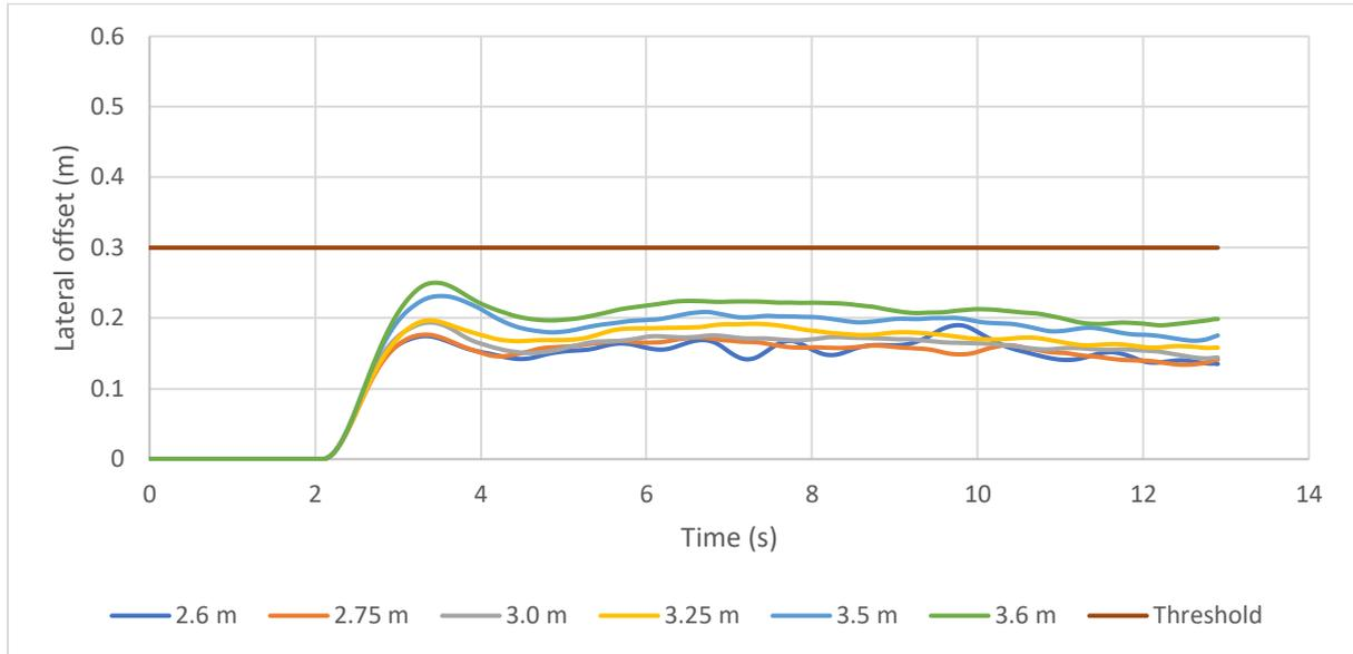
Figure 65: Lateral offset variations for test cases with 900 m radius and speed of 100 km/h
