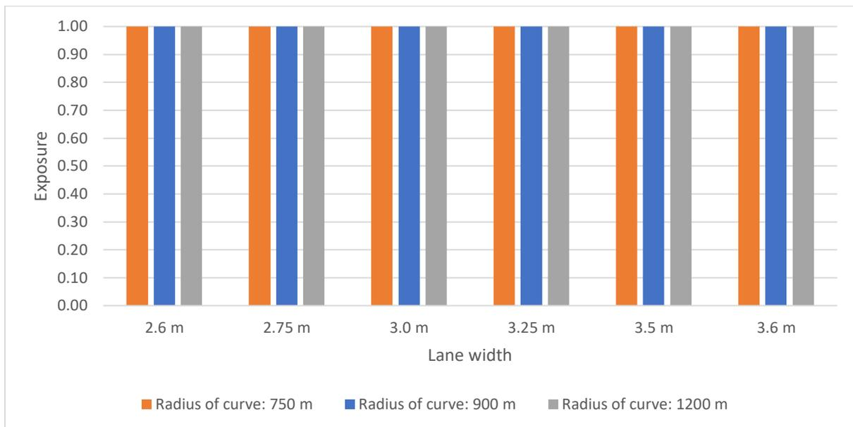
Figure 29: Exposure data comparison between different lane widths and radii for test cases of 100 km/h
