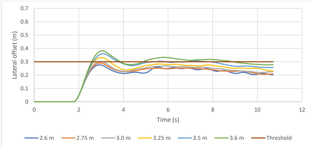
Figure 62: Lateral offset variations for test cases with 750 m radius and speed of 120 km/h
