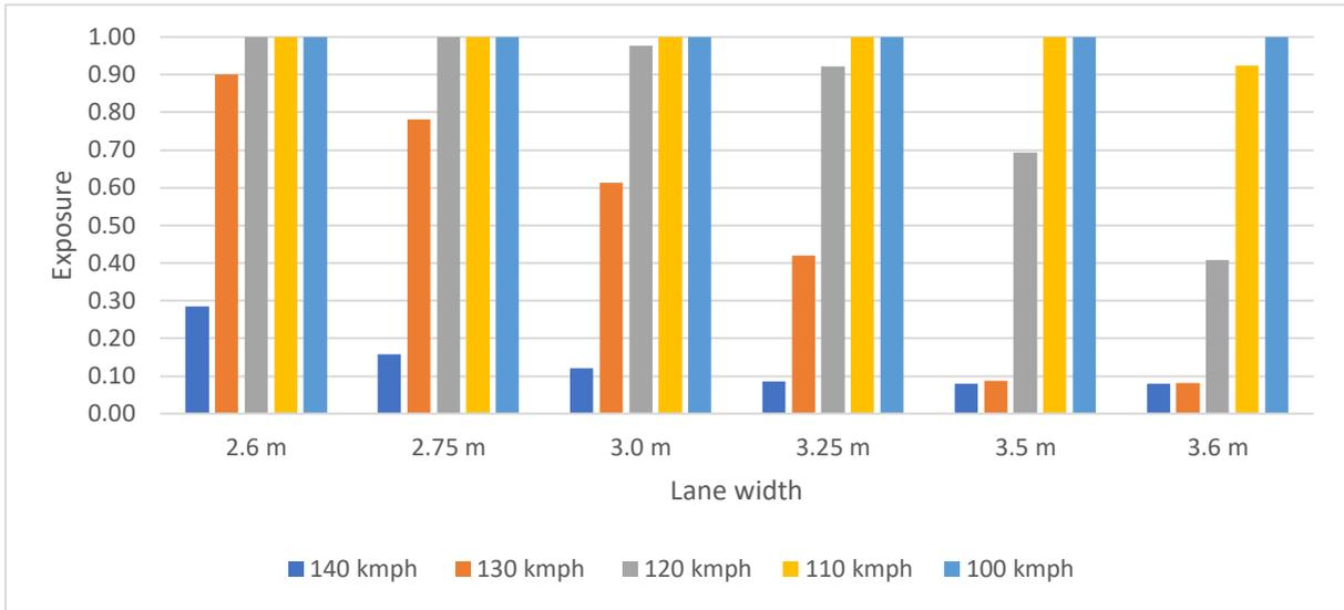
Figure 26: Exposure data comparison between different lane widths and speeds for test cases of 750 m radius curve
