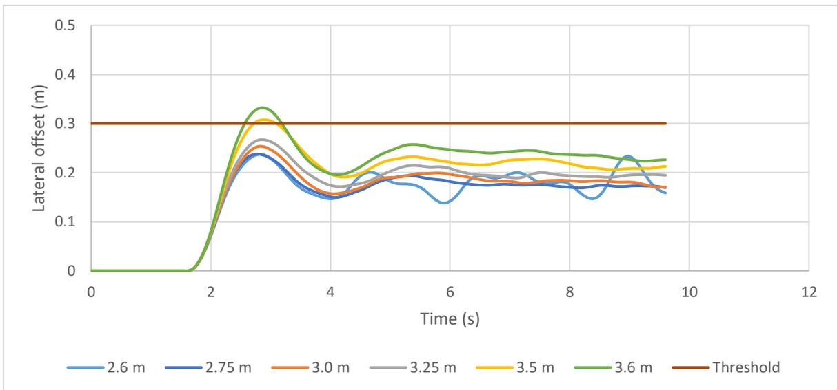
Figure 73: Lateral offset variations for test cases with 1200 m radius and speed of 130 km/h
