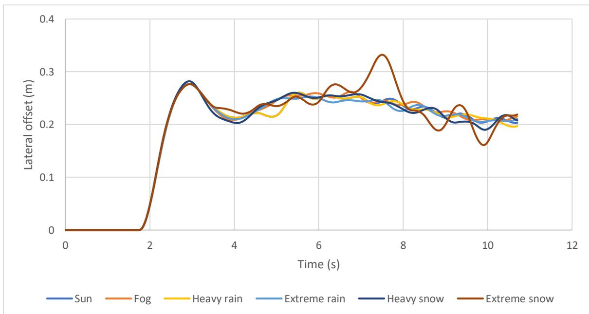
Figure 39: Lateral offset variation for different weather conditions at 2.6 m lane width, 750 m radius and 120 km/h
