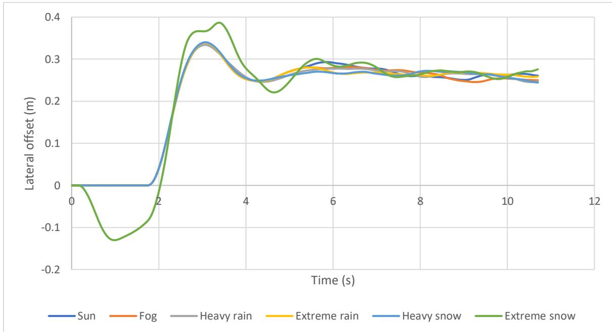
Figure 37: Lateral offset variation for different weather conditions at 3.6 m lane width, 900 m radius and 120 km/h
