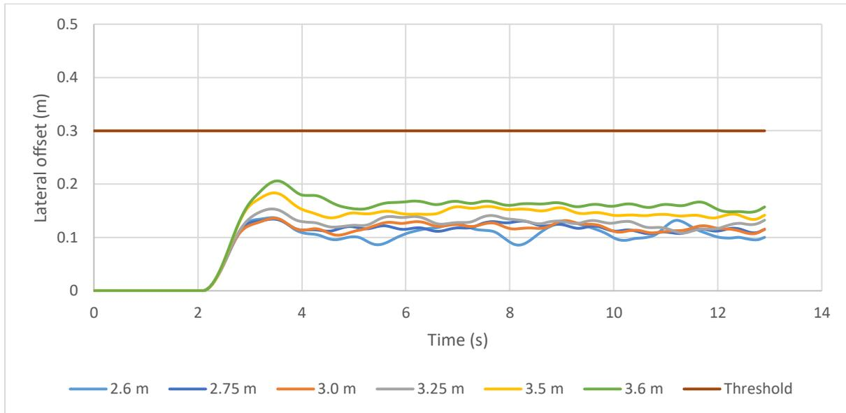
Figure 70: Lateral offset variations for test cases with 1200 m radius and speed of 100 km/h
