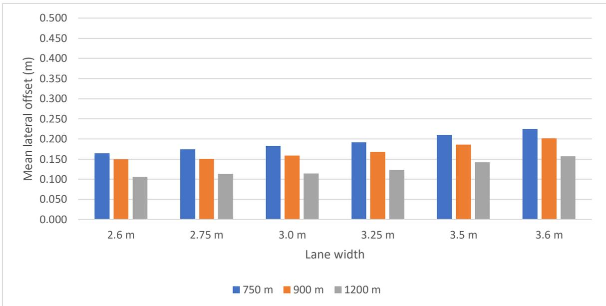
Figure 23: Mean lateral offset variation for 100 km/h
