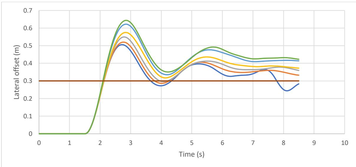
Figure 64: Lateral offset variations for test cases with 750 m radius and speed of 140 km/h
