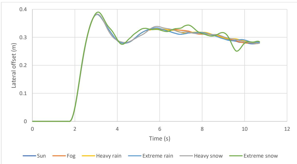
Figure 41: Lateral offset variation for different weather conditions at 3.6 m lane width, 750 m radius and 120 km/h
