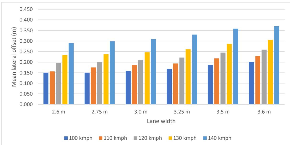
Figure 21: Mean lateral offset variations for 900 m radius curve
