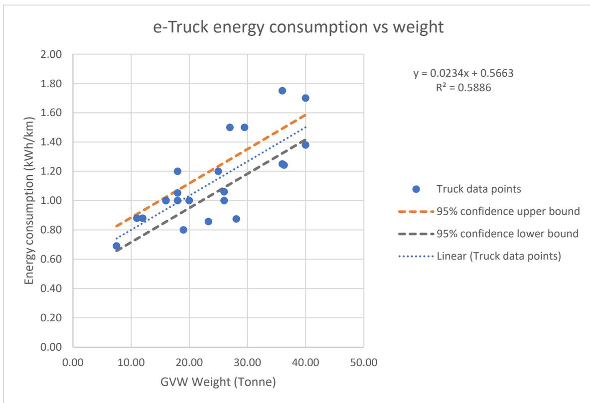
Figure 19: Relation between e-Truck energy consumption and weight
