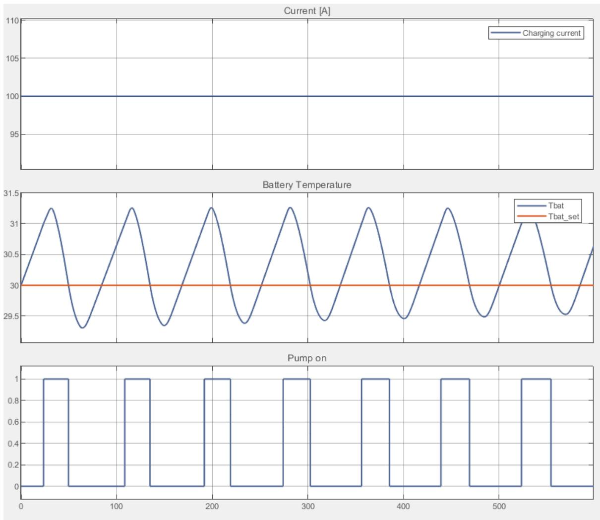
Figure 18: MATLAB Simulink BTMS results
