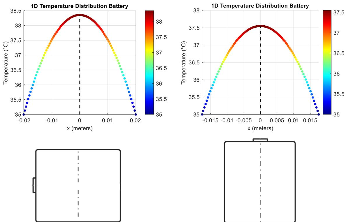
Figure 14: 1-dimensional in-plane conductive heat transfer through battery cell's (a) long dimension and (b) short dimension
