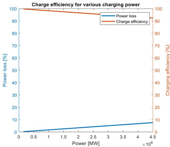
Figure 13: Power loss due to resistive heating at various charging rates
