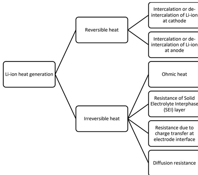
Figure 2: Heat generation classifications in Li-ion batteries. Adapted from (Choudhari, et al., 2020)
