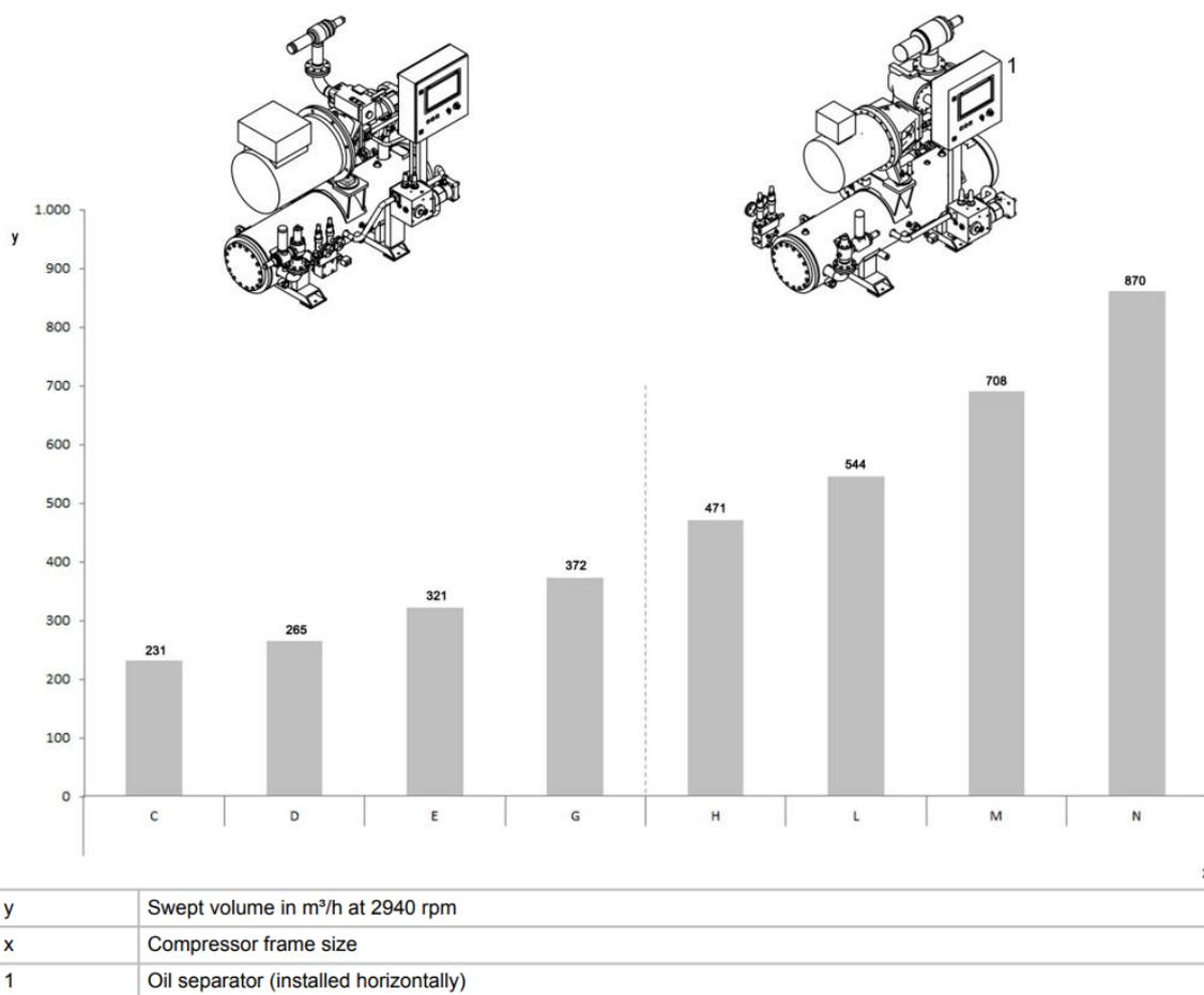
Figure 28: Variations of GEA ammonia compressor and their volumetric flow rate (GEA, 2021)
