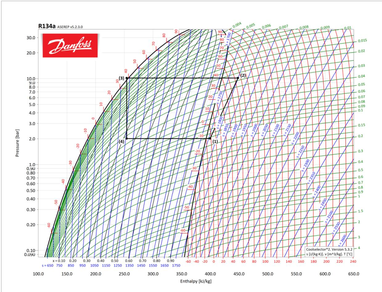
Figure 25: Log-ph diagram of R134a
