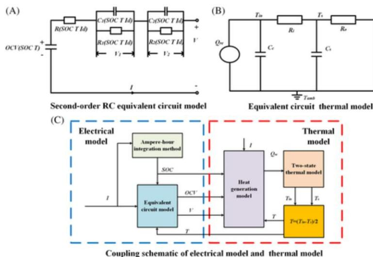
Figure 5: Schematic of (A) equivalent circuit model, (B) thermal model, (C) electro-thermal model. Adapted from (Chen, Hu, Cao, et al. 2020)
