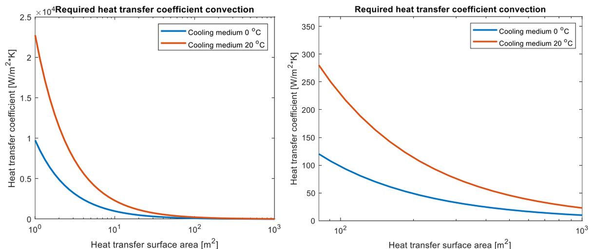
Figure 16: Required heat transfer coefficient for various surface area quantities at a battery surface temperature of 35 °C
