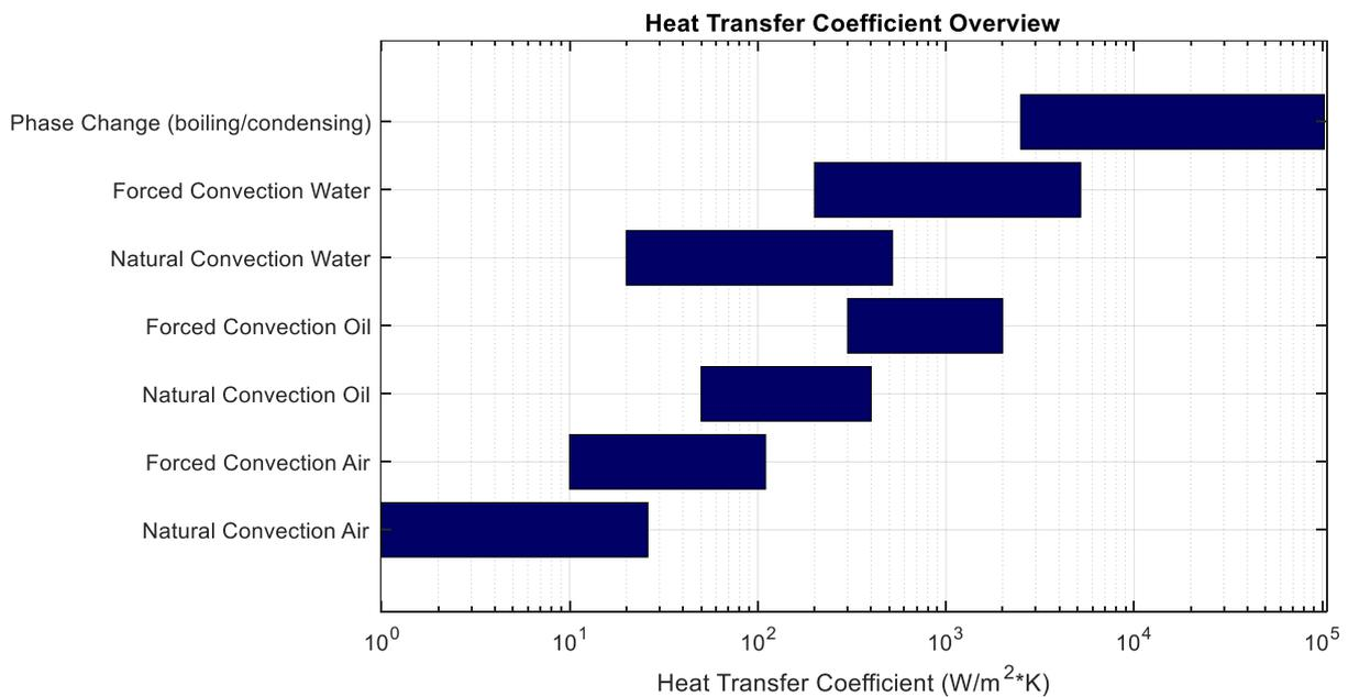
Figure 9: Overview of cooling strategy heat transfer coefficient for convection (Aamir, et al., 2016) (Sridhar, 2013) (Vargas, et al., 2018) (Moran, et al., 2012)
