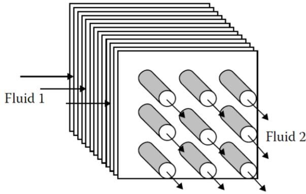
Figure 10: Crossflow heat exchanger (B. Noshirvani University of Technology, 2023)
