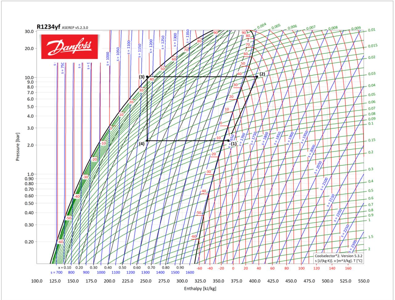
Figure 26: Log-ph diagram of R1234yf
