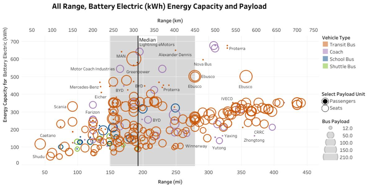
Figure 8: Electric bus data (CALSTART, 2023)
