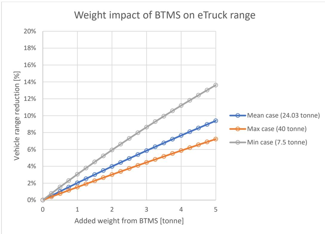
Figure 20: Relation between e-Truck added weight and driving range reduction
