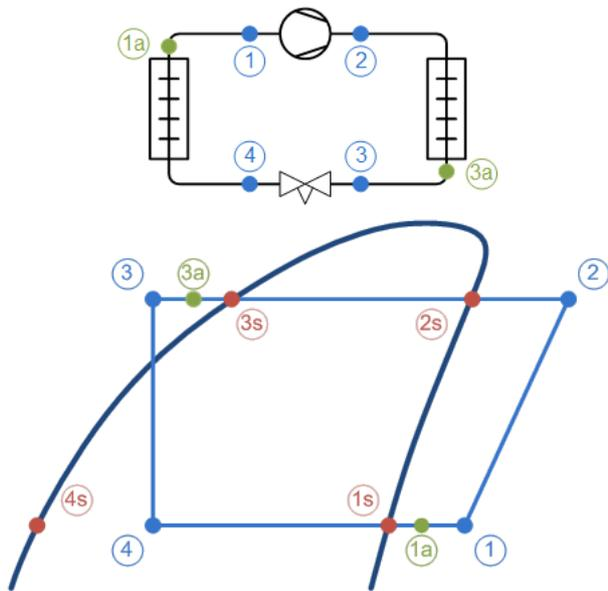
Figure 17: Schematic representation of the vapor-compression cycle (Danfoss, 2023)
