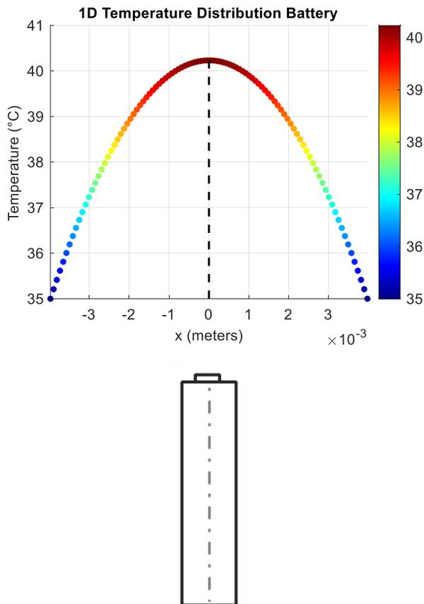
Figure 15: 1-dimensional cross-plane conductive heat transfer through battery cell
