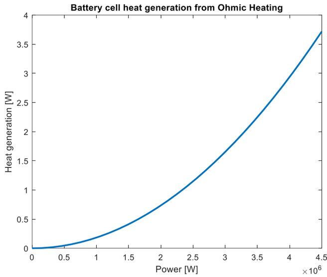
Figure 12: Battery cell heat generation from Ohmic Heating at various charging rates
