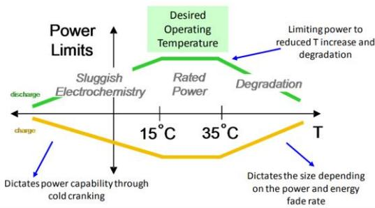
Figure 1: Battery optimal temperature range and power limits. Adapted from (Pesaran, et al., 2013)
