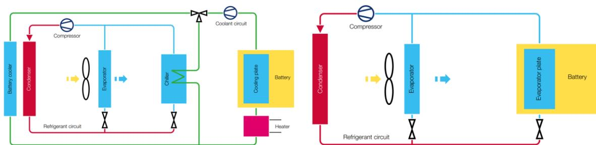
Figure 4: Battery thermal management by dual-circuit (left) and refrigerant-based single-circuit (right). Adapted from (Wang, et al., 2016) and (Mahle Behr, 2021)
