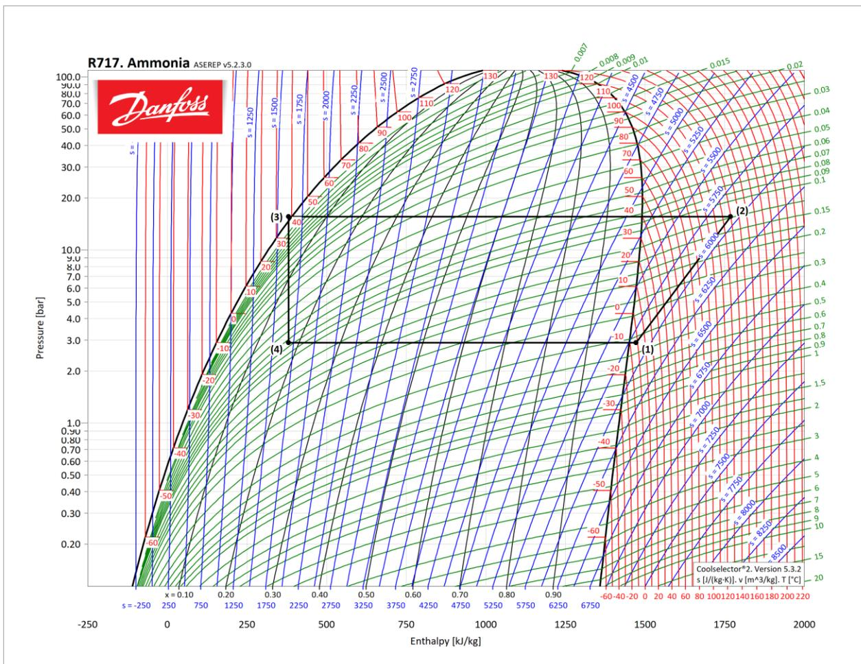
Figure 24: Log-ph diagram of R717
