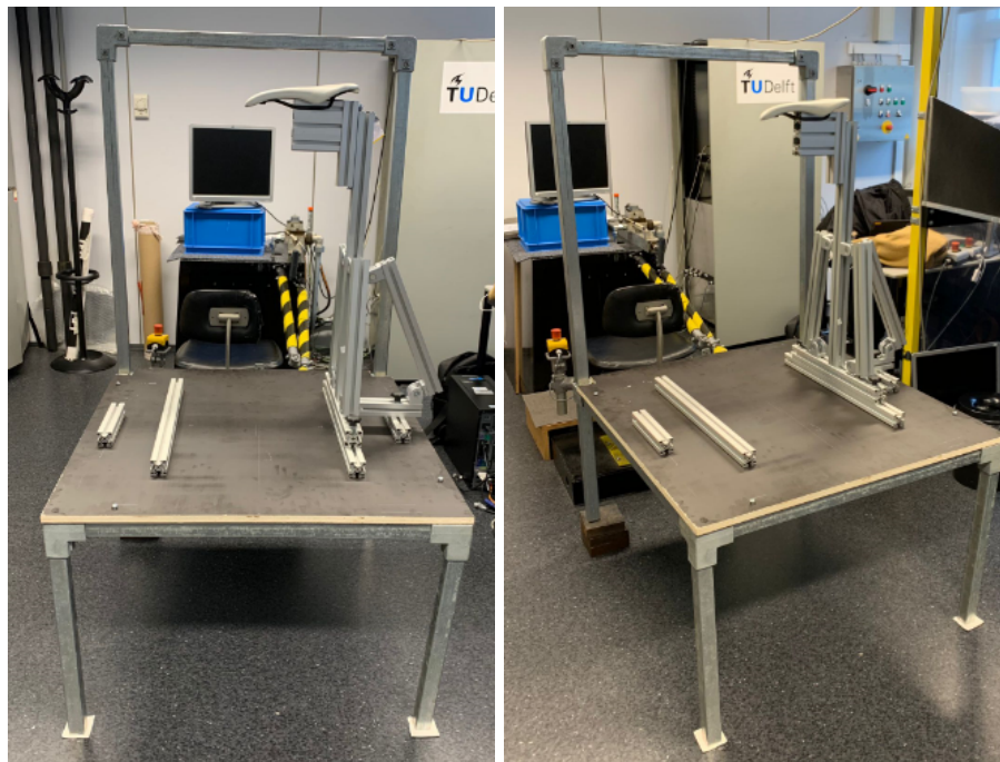
Figure 4: The experimental set-up shown in the lab in front of the Proprio. It is not positioned correctly here, due to the presence of the seat from the old set-up, obstructing its proper placement.
