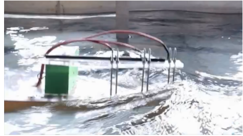
(b) Before slamming: water exceeds deck level
