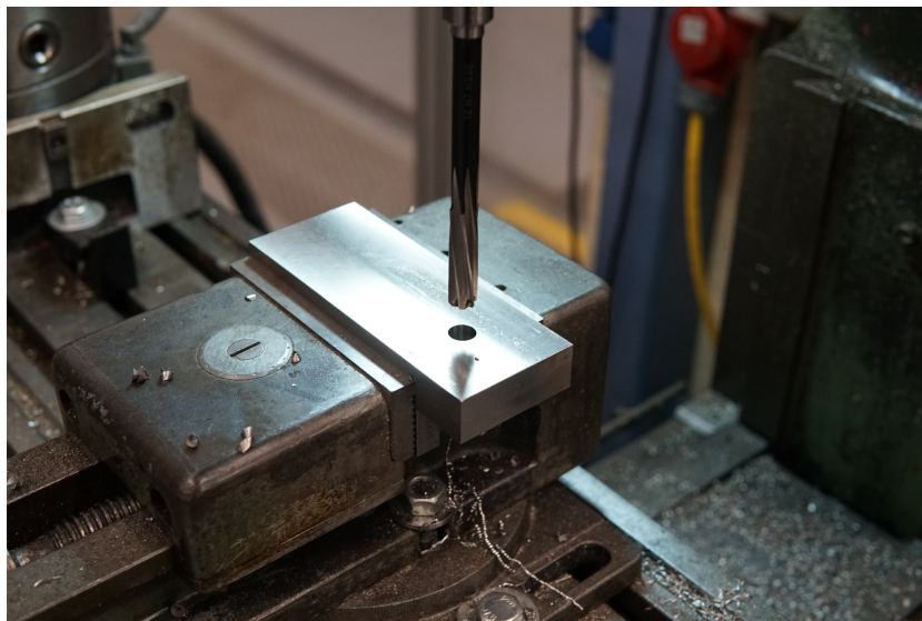
Figure E.1: Machining the bore that interfaces with both the oxygen injector and the resonator.
