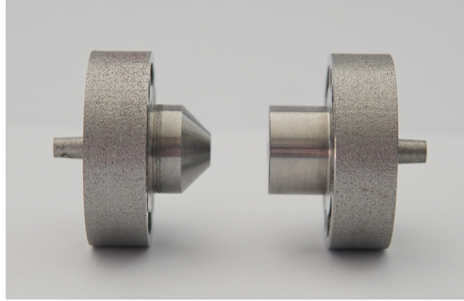
Figure 5.4: Comparison between the conical (left) and cylindrical resonator (right).
