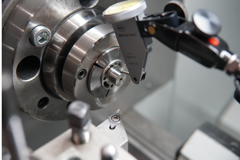
Figure E.2: Measuring concentricity between the cavity inlet and the interface between the resonator and combustion chamber using a small dial indicator.
