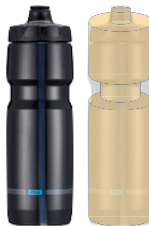
FIGURE 7. Illustration of model-based prediction as described in [7]. In this example a bottle is modeled via 4 cylinders.
