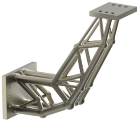
Figure 2.15: A satellite antenna bracket designed with the truss optimisation tool (from He et al. [51])
