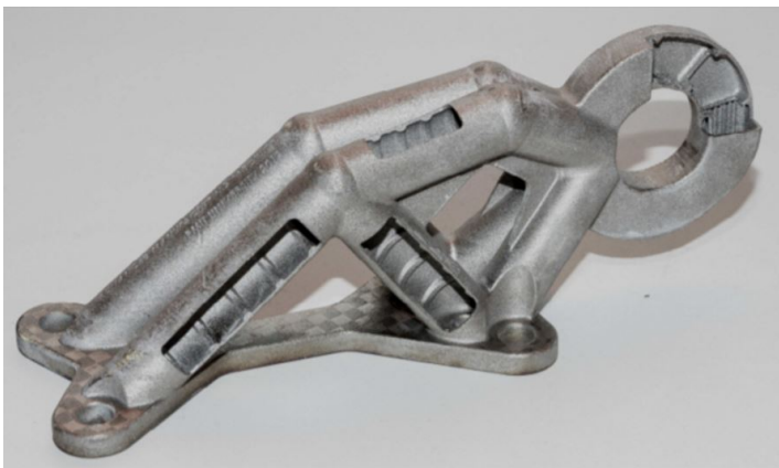
Figure 2.11: Multilevel designed bracket (from Brandt et al. [25])
