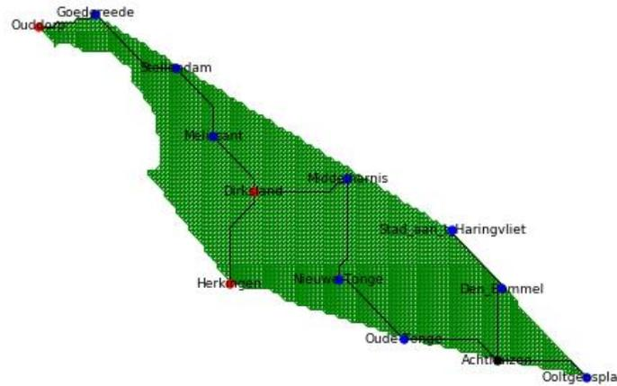
Figure 37 Initial solution for the electricity network in Goeree-Overflakkee.
