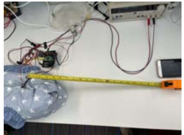
Figure F.9: The test setup for measuring the sound intensity of the pumps, with the pumps being inside the two pouches.
