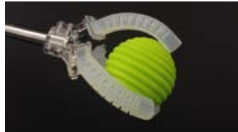
Figure 1.2: A small silicon-rubber based soft robot. By inflation of the robot, the flexible material expands and causes deformation, leading to movement. Source: Ryan Truby/Harvard SEAS.
