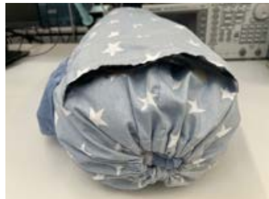
Figure A.7: The outer pouch contains a pocket for the Velostat sheet, with velcro to keep the sheet in place.
