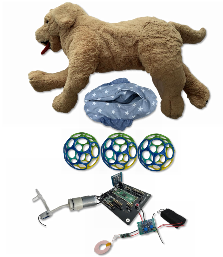
Figure A.1: Assembly overview of the Teddy. Looking from top to bottom you can see the teddy, the pouch, the mounting/integration balls, and the PCB, the batteries, and the pumps.
