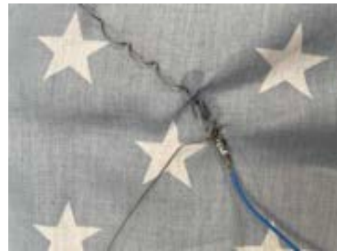
Figure F.3: Close up of the way the wire and conductive thread are integrated to make contact with the Velostat.
