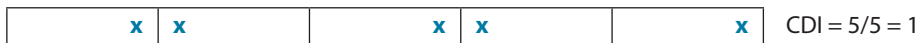
Figure 2-10 | Two sample distributions of five spacecraft along one dimension of interest. 'x' indicates spacecraft
