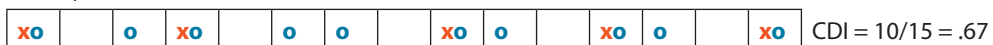
Figure 2-11 | Two sample distributions of five spacecraft along one dimension of interest. 'x' indicates actual spacecraft and ten dummy spacecrafts are introduced and denoted by 'o'
