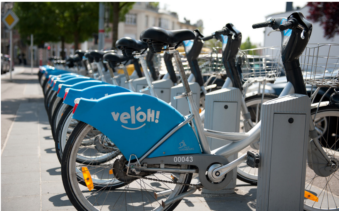
Figure 2.3 Veloh! bicycles in the city of Luxembourg. These docked bicycles can be used with a subscription. A card is presented at the locking pole, verifies the user and deducts a certain amount of money when the bicycle is returned to any docking station in the city. According to Shaheen e.a. one of the latest developments in the second generation.
