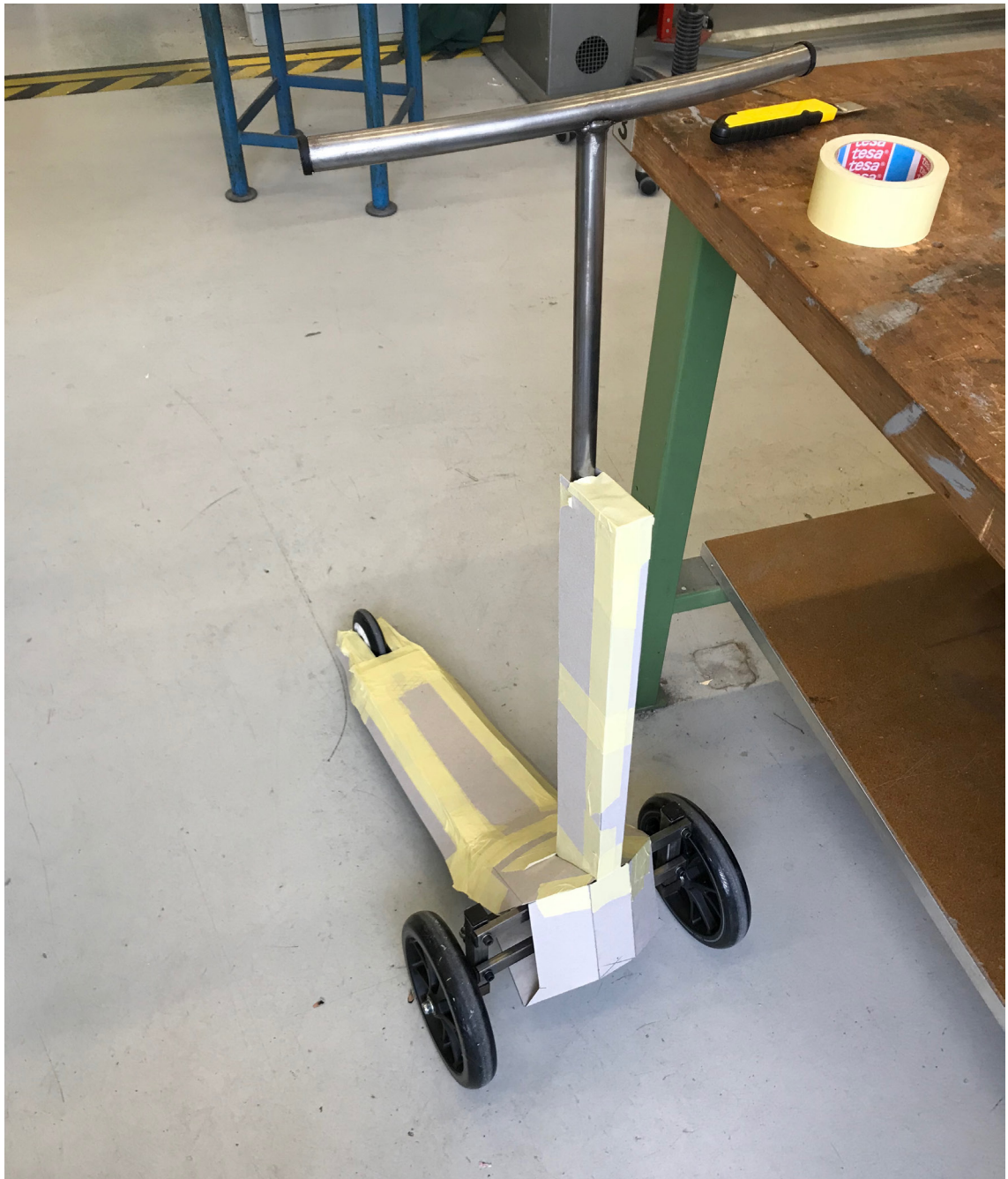
Figure 4.3 Cardboard exploration of a tubular frame with covering panels
