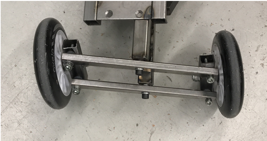
Figure 3.4 A parallelogram configuration that translates a leaning motion into both a tilting and steering action
