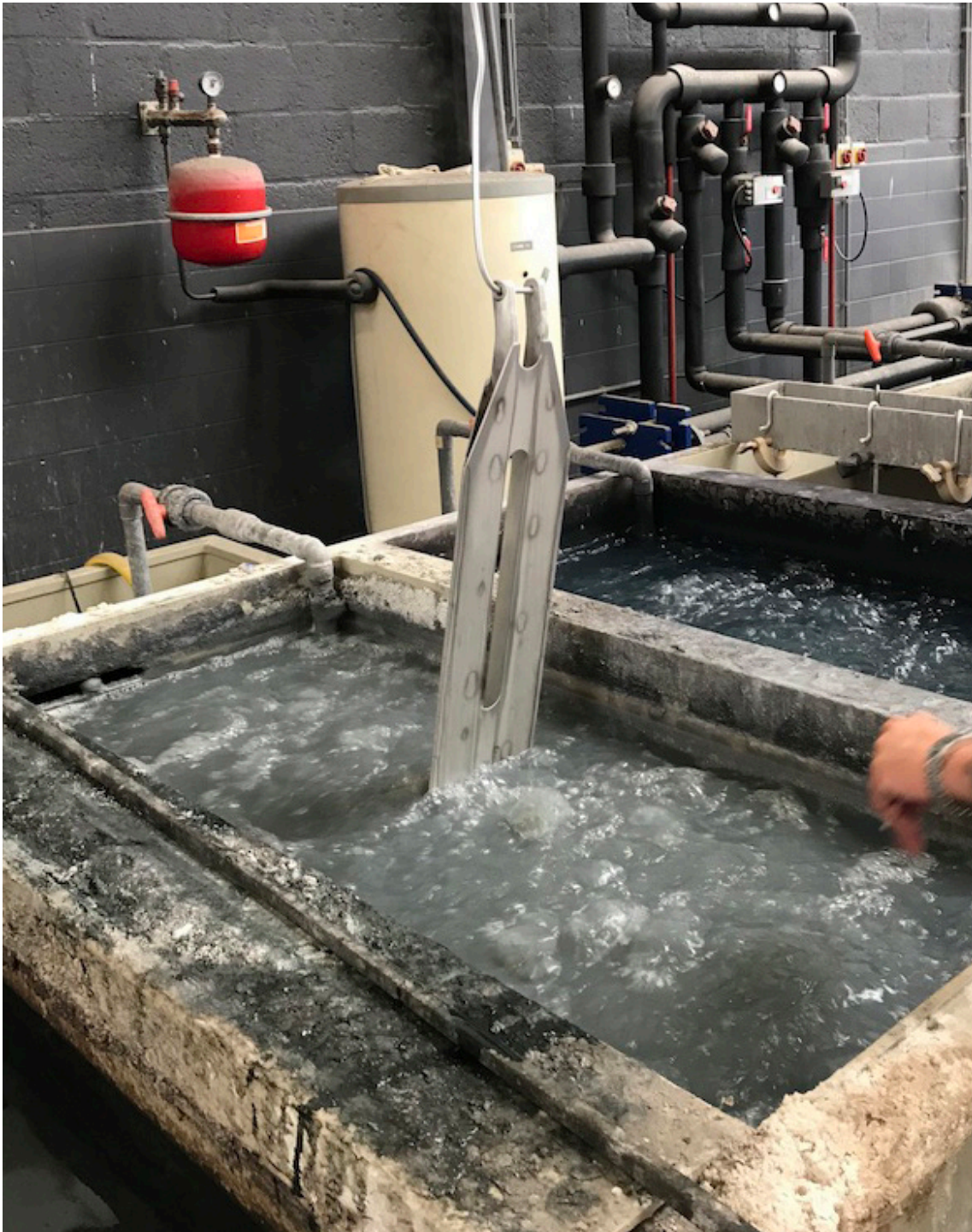
Figure 4.13 The deionizing process highlights all the welded spots and seams. The bath contains an alkaline dissolved in water and kept at 60°C. Once an aluminium object is placed in the bath the chemical reaction between aluminium/aluminium oxide removes a thin layer of the surface, either deionizing it or preparing the surface for anodizing.
