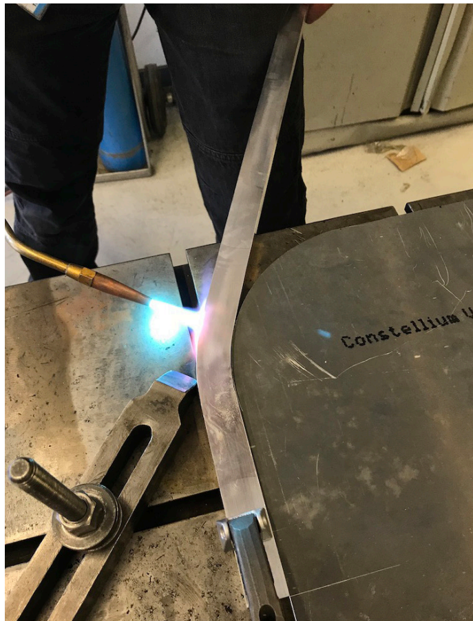
Figure 4.7 (top) Prototyping and simulating the extruded aluminium footboard
