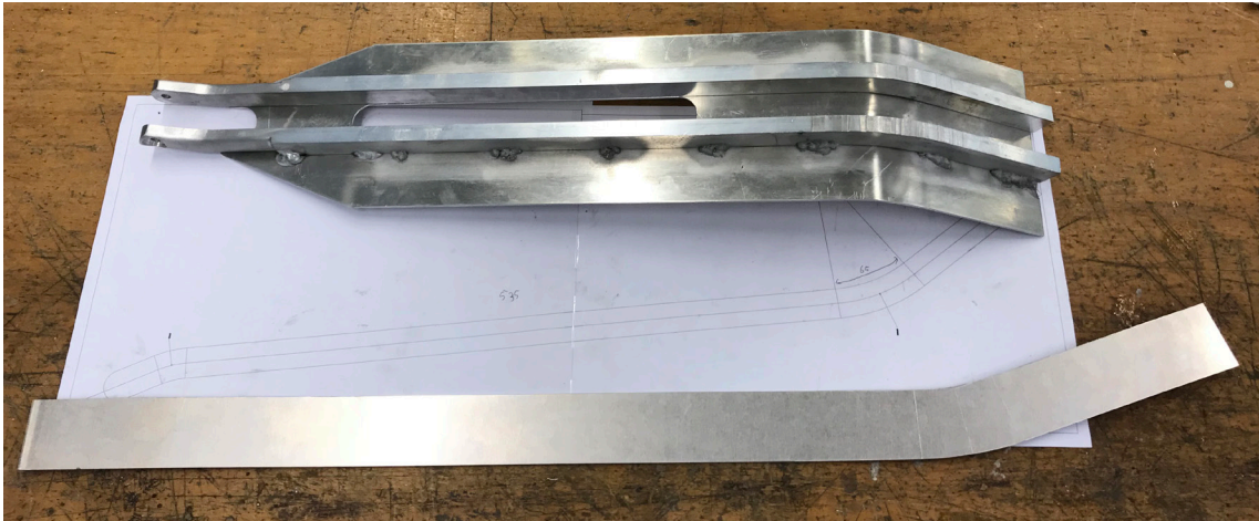
Figure 4.7 (top) Prototyping and simulating the extruded aluminium footboard
