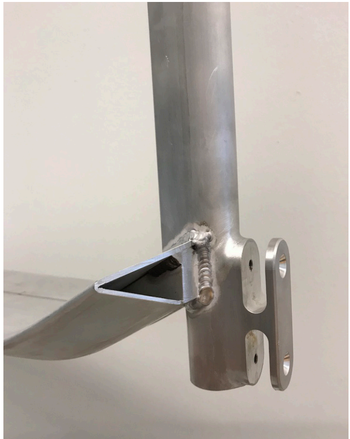
Figure 4.9 (top) TIG welding sheet aluminium to simulate the extruded profile
