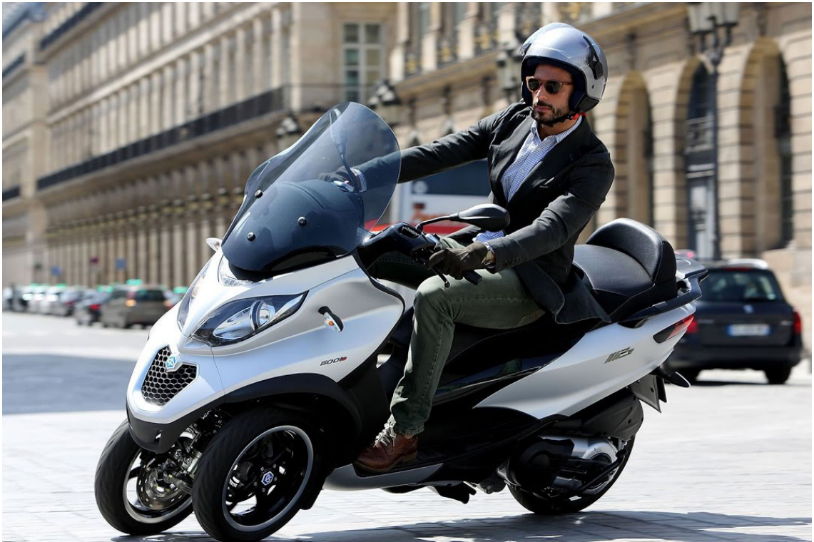
Figure 2.16 (top) A Piaggio MP3. The front steering assembly allows the Piaggio to both steer and tilt. A single parallelogram performs the tilting action. The suspension is provided directly on the wheels
