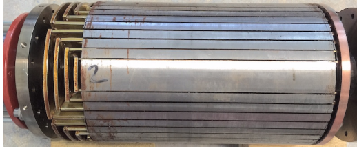
Fig. 2. Nested-loop rotor constructions
