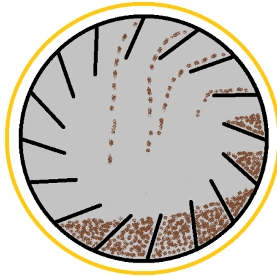
Figure 3.1: Standard aggregate heater design. The coil is shown as a gold ring around the drum. The flights pick up the aggregate and drop it once they reach the top. The aggregate curtains out over the middle of the drum.
