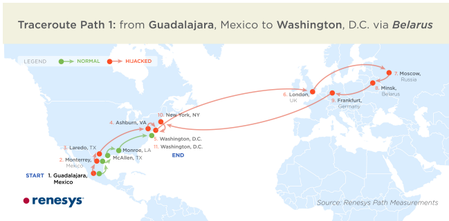
Fig. 3. The normal path and diverted path of Internet traffic during the Belarussian traffic diversion, retrieved via dyn.com [1].
