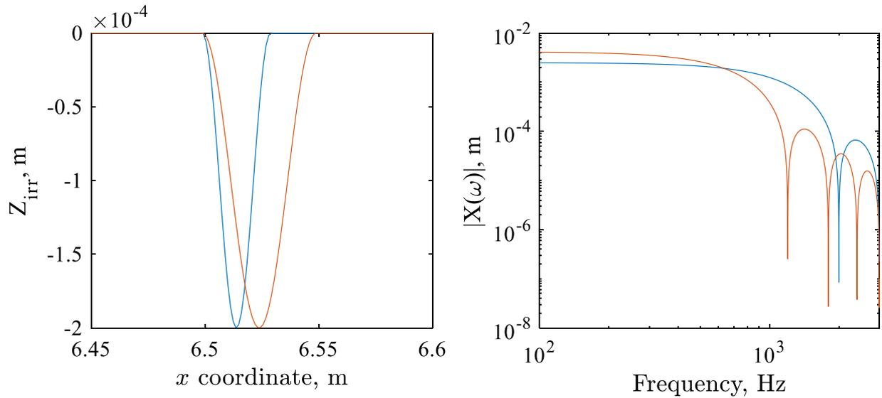
Fig. 12. Geometries of two typical rail surface defects in the space and frequency domain (a)  $Z_{irr}(x)$  (b) Magnitude of the Fourier coefficient  $X(\omega)$ . Blue line: length 30mm, depth 0.2 mm; red line: length 50mm, depth 0.2mm. Both defects start at 6.5m which is near the center of a sleeper support at 6.6 m.
