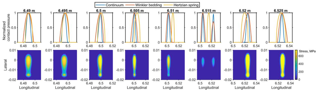
**Fig. 6.** Influence of contact models on the contact solution. First row: contact pressure distribution normalized to its maximum value. The title of each subplot indicates the wheel center position. Second row: contact patch and pressure distribution obtained by the continuum model.
