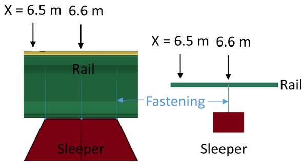
Fig. 7. The two locations for calculating track receptance.
