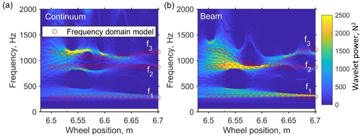
**Fig. 15.** Comparisons between the characteristic frequencies predicted by the time domain and frequency domain models. (a) Continuum model; (b) beam model. The SWPSs are obtained by the time domain models. The red circles indicate a sequence of the *frozen configuration* responses at each wheel position obtained by the frequency domain models.
