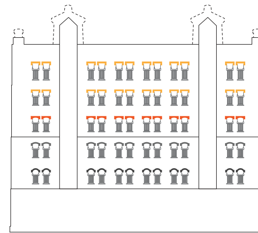
FOUR DIFFERENT TYPES OF WINDOWS THAT REFLECT THE CONSTRUCTION.
