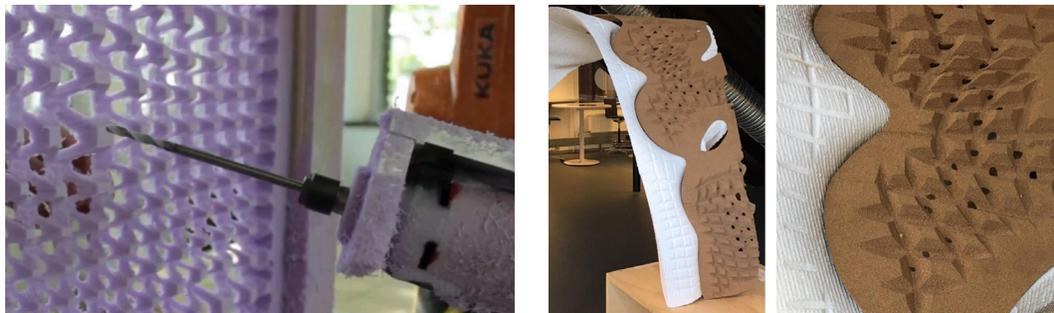
FIGURE 6 Hybrid Assembly, extending material properties to enhance the performance through integration of multiple materials and fabrication methods
