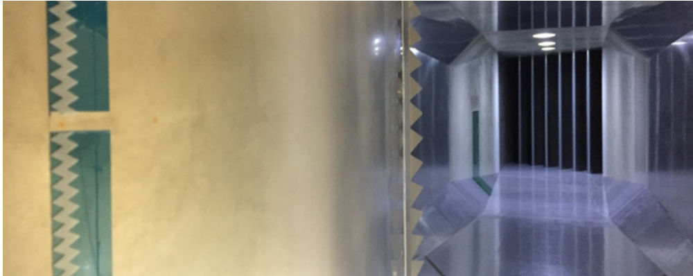
Fig. 7 NWB test set-up with tripping detail.
