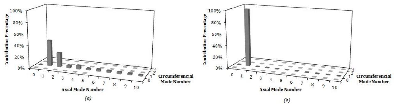
Figure 5.31: Mode contribution under horizontal loading at the first resonance peak at (1.72 Hz):
