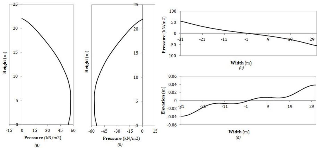
Figure 5.25: Pressure and free surface elevation seismic loading in horizontal direction at **1.97 Hz** for Model A: (a) wall Pressure at  $\theta = 0$  ;(b) wall pressure at  $\theta = \pi$ ; (c) plate pressure; (d) free surface elevation
