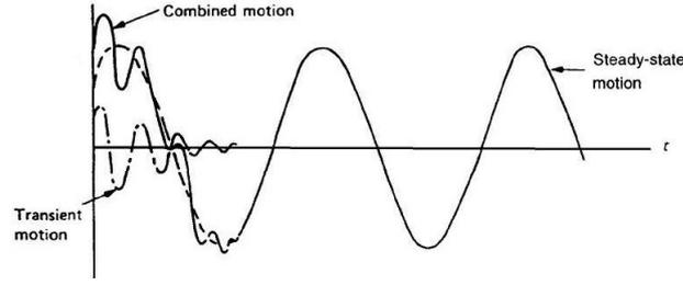
Figure 2.13: The total, steady-state, and transient solution of the system
