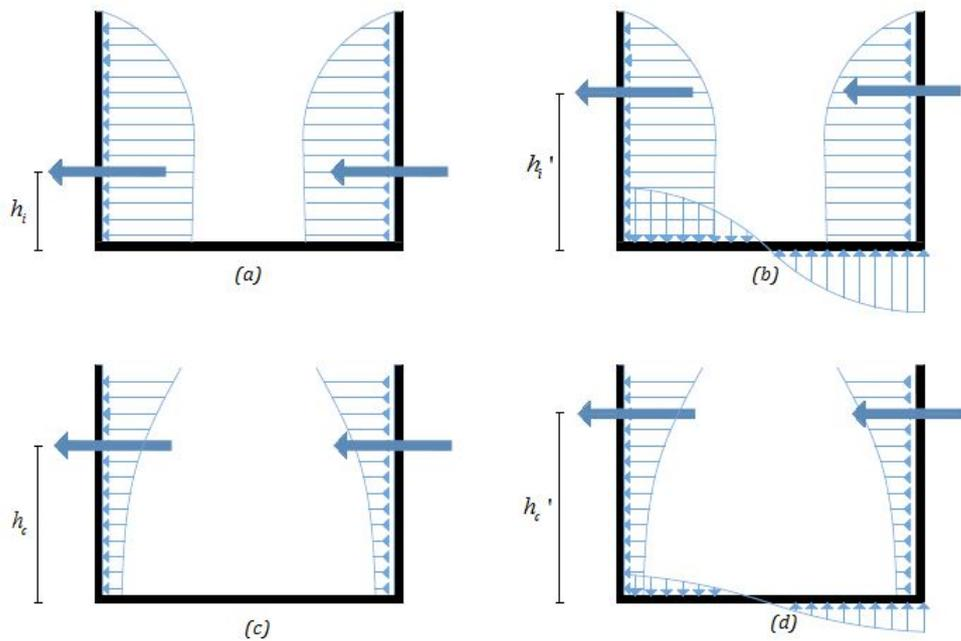
Figure 2.20: The distribution and centroidal heights of impulsive (a,b) and convective (c,d) pressures.
