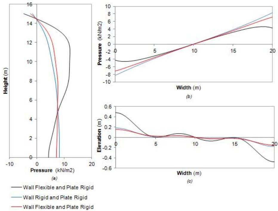
Figure 3.33: Pressure and free surface elevation for different Flexibility Seismic Loading in x Direction at frequency 0.3847 Hz:
