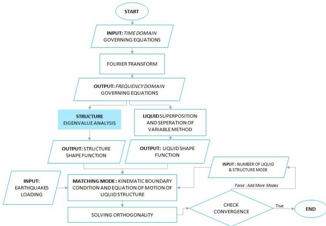
Figure 3.2: The Process Flowchart of the Two-Dimensional Model
