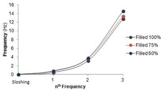
Figure 3.28: Change of frequencies in the different liquid volume for Seismic loading in Z direction
