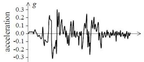
Figure 2.6: Recorded acceleration in accelerogram
