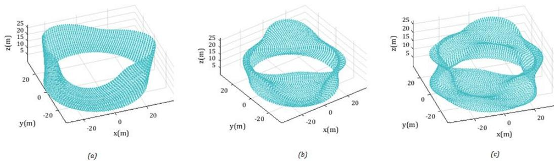
Figure 5.14: Mode shape with *circumferential* mode number( $m$ ) = 3 from Matlab, (a) axis mode number 1 ;(b) axis mode number 2 ;(c) axis mode number 3
