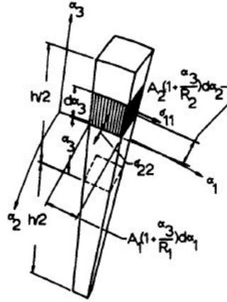
Figure B.5: Cut infinitesimal cross-sectional dimensions
