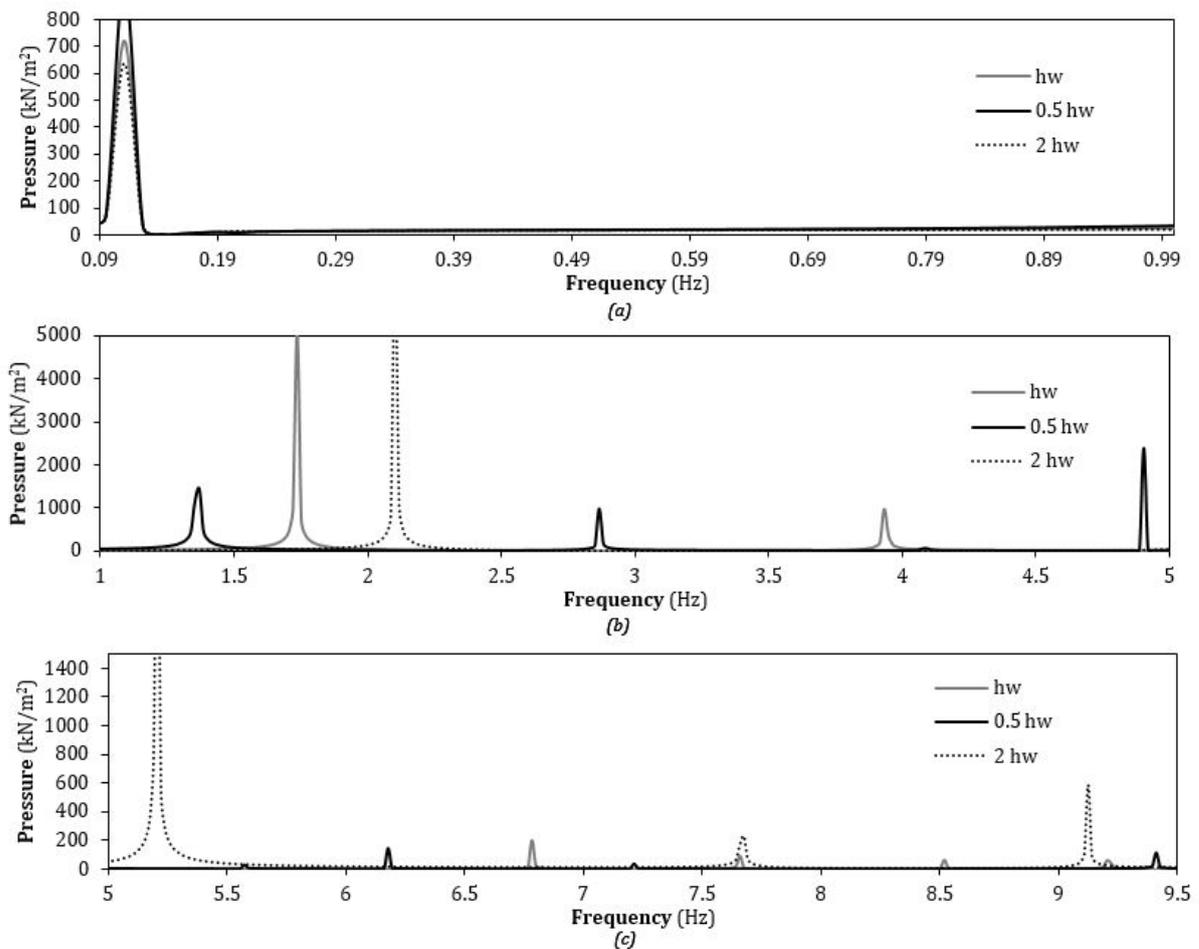
Figure 5.42: Frequency response of pressure for different wall thickness under horizontal loading; (a) low frequency range; (b) medium frequency range; (c) high frequency range
