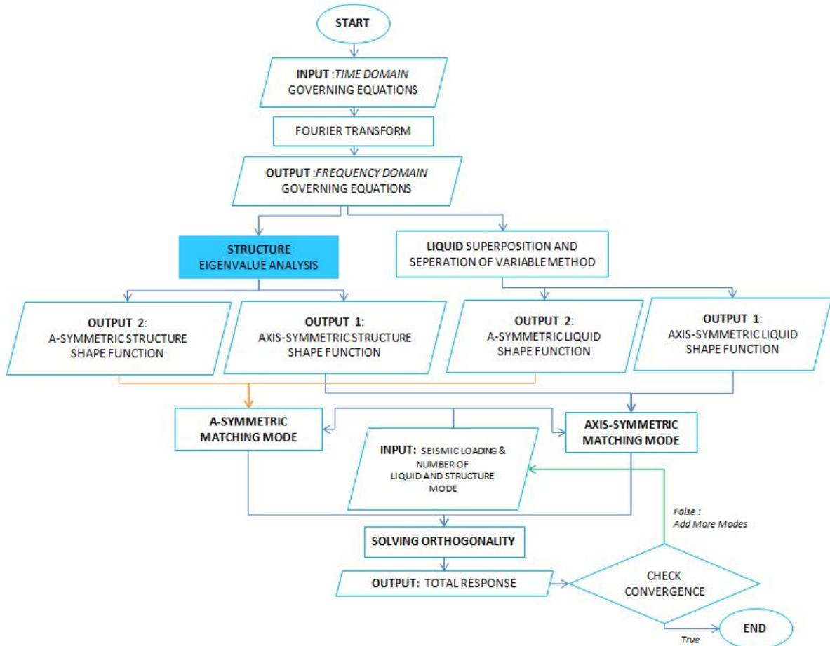
Figure 4.2: The three-dimensional process flowchart
