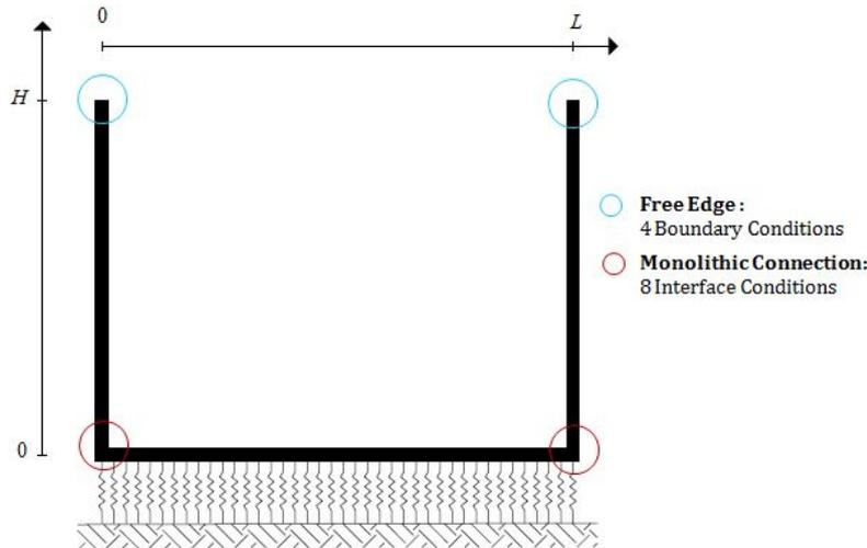
Figure 3.6: Boundary and interface conditions of the structure
