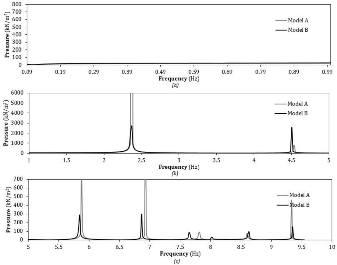
Figure 5.32: Frequency response of Model A and Model B wall pressure in term of pressure under vertical loading: (a) low frequency range; (b) medium frequency range; (c) high frequency range
