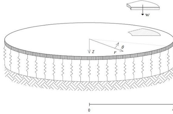
Figure 4.6: Circular plate axis and degree of freedom
