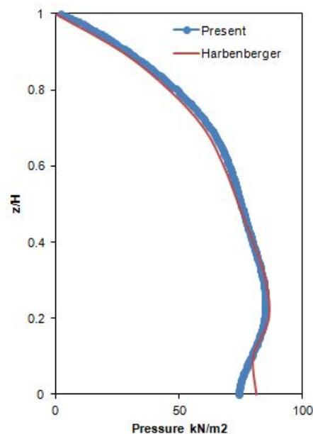
Figure 5.57: Hydrodynamic wall pressure ( $\theta = 0$ ) compare to Habenberger under horizontal loading
