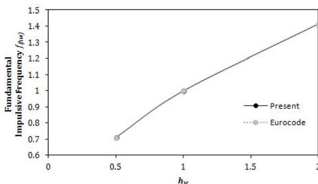
Figure 5.44: Fundamental frequency difference for different wall thickness
