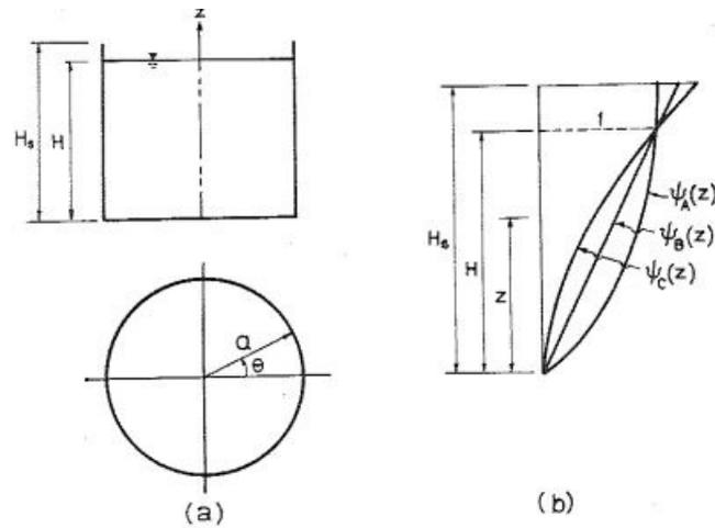
Figure 2.24: The tank system (a) ; example vibration mode shapes (b)
