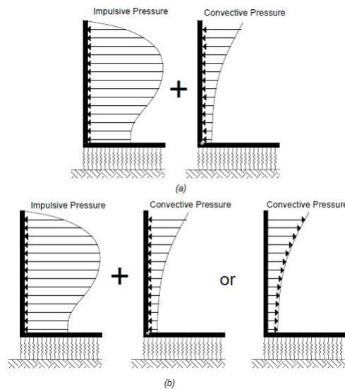
Figure 3.19: Conservative vs actual hydrodynamic pressure: (a) conservative total pressure; (b) actual total pressure
