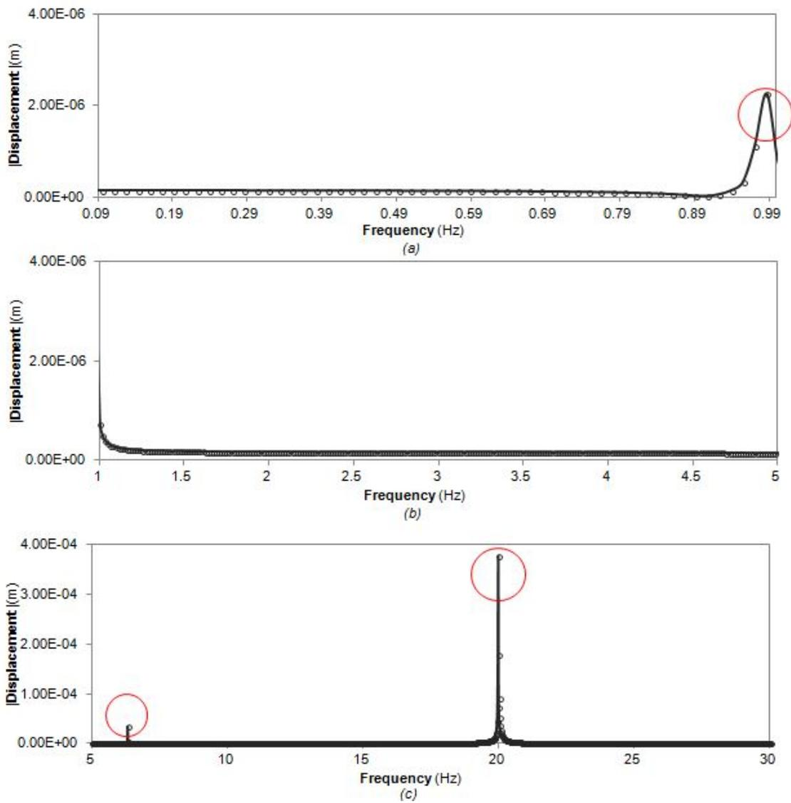
Figure 3.14: Frequency response in term of deformation for empty tank under seismic loading in vertical direction: (a) low frequency range;(b) medium frequency range ;(c) high frequency range
