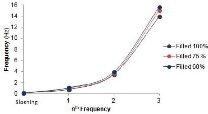
Figure 3.27: Change of frequencies in the different liquid volume for Seismic loading in X direction
