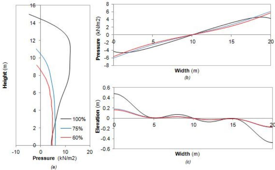
Figure 3.29: Wall Pressure for Liquid Volume Percentage Seismic Loading in x Direction at frequency 0.59 Hz: (a) Wall Pressure (b) Plate Pressure (c) Free Surface Elevation
