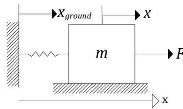
Figure 2.10: The earthquake loading in Single Degree of Freedom
