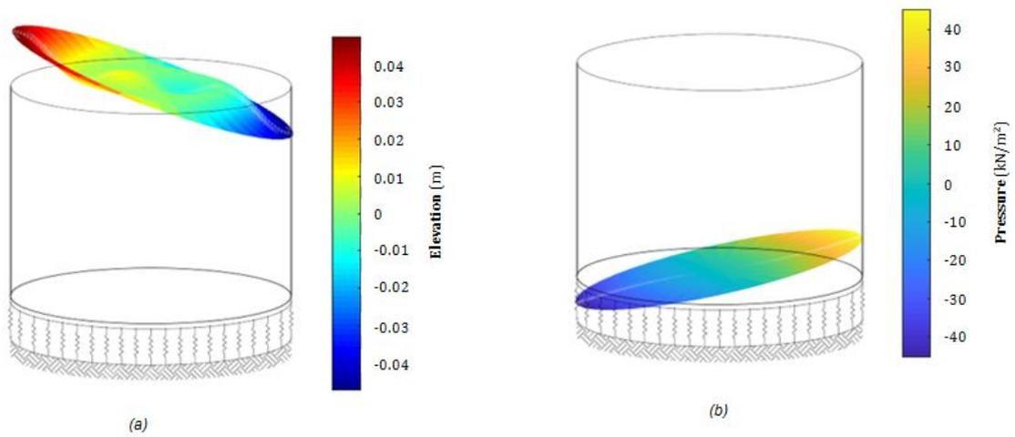
Figure 5.29: Plate pressure and free surface elevation seismic loading in horizontal direction at **1.97 Hz** in 3D cross section for Model B: (a) free surface elevation; (b) plate pressure
