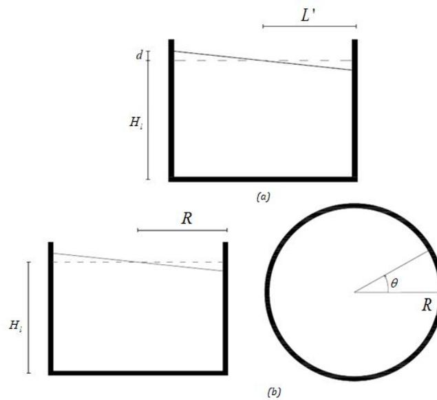
Figure 2.22: (a) The cross section of rectangular tank; (b) The cross section of cylindrical tank. (Source : The dynamic behaviour of Water Tanks, George W, Housner[7])
