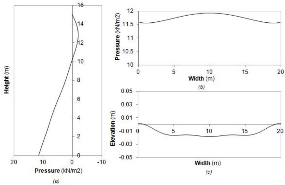
Figure 3.22: Pressure and free surface Elevation seismic loading in z direction at 1.431 Hz:
