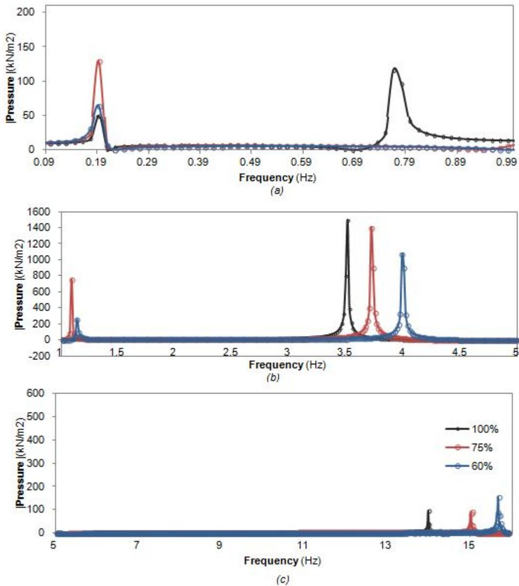
Figure 3.25: Frequency response in term of pressure for different liquid volume under seismic loading in horizontal direction: (a) low frequency range;(b) medium frequency range ;(c) high frequency range
