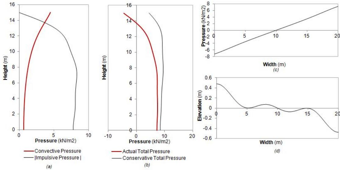
Figure 3.20: Pressure and free surface elevation seismic loading in x direction at 0.318 Hz:
