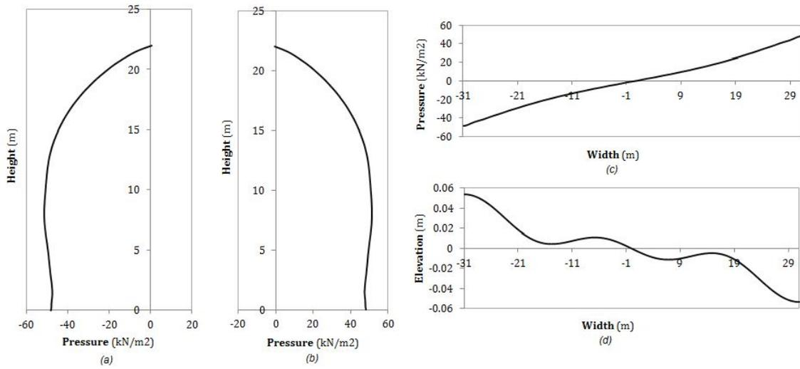
Figure 5.28: Pressure and free surface elevation seismic loading in horizontal direction at **1.97 Hz** for Model B: (a) wall Pressure at  $\theta = 0$ ; (b) wall pressure at  $\theta = \pi$ ; (c) plate pressure; (d) free surface elevation
