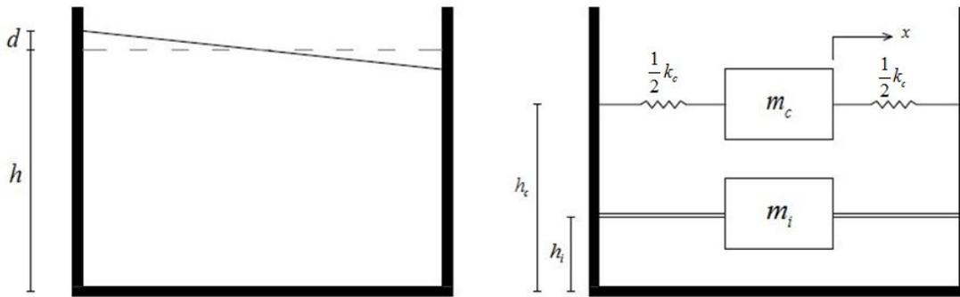
Figure 2.21: Equivalent of a dynamic system of the tank from Housner. The discrete lumped mass can be seen in the right. The impulsive mass ( $m_i$ ) and the compulsive mass ( $m_c$ ) equivalent to the forces that are produced by the water. (Source : The dynamic behaviour of Water Tanks, George W, Housner[7])
