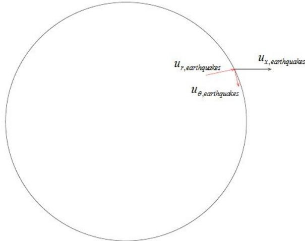
Figure 4.4: The projection of horizontal seismic loading
