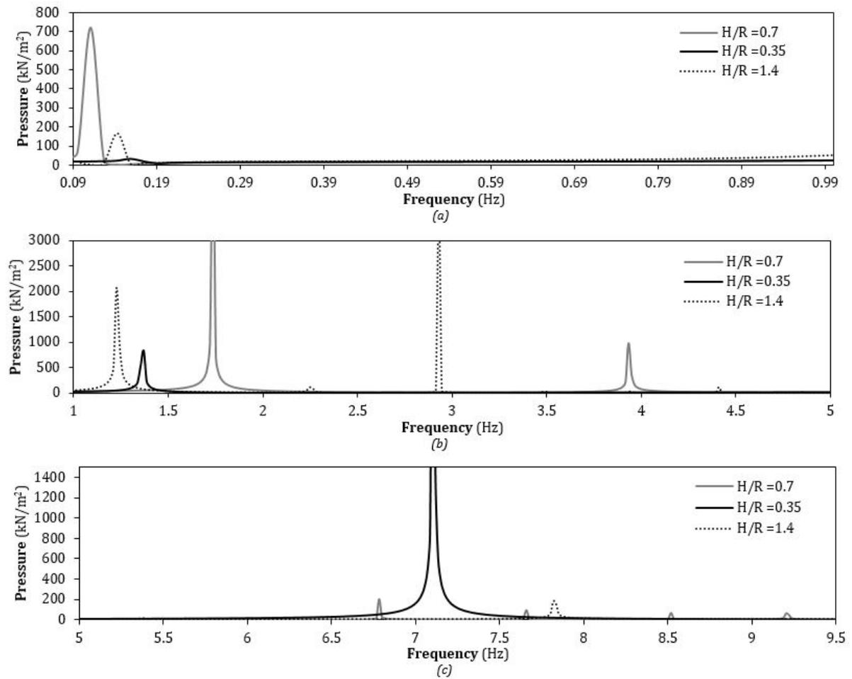
Figure 5.48: Frequency response of pressure for different From Geometry under horizontal loading:(a) low frequency range; (b) medium frequency range; (c) high frequency range
