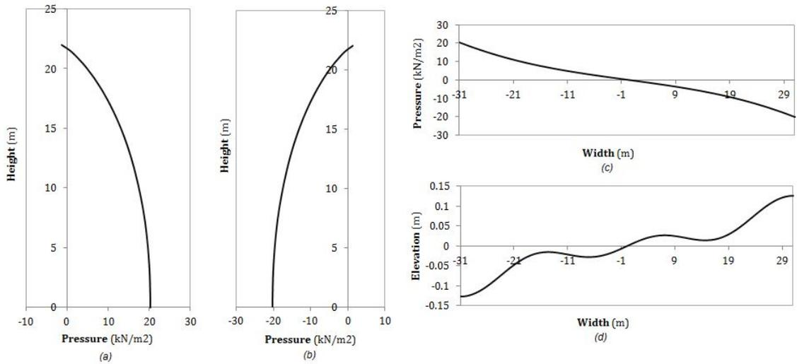
Figure 5.24: Pressure and free surface elevation seismic loading in horizontal direction at **0.700 Hz** for Model A: (a) wall Pressure at  $\theta = 0$  (b) wall Pressure at  $\theta = \pi$  (c) plate pressure (d) free surface elevation
