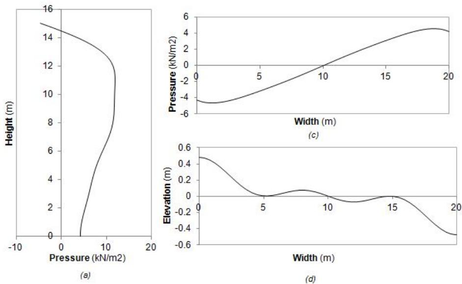
Figure 3.21: Pressure and free surface elevation seismic loading in x direction at 0.955 Hz:
