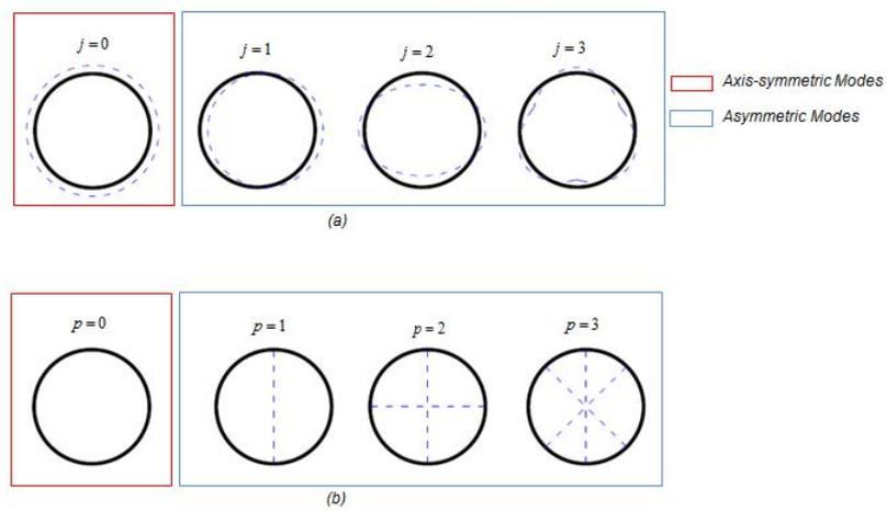
Figure 4.13: Axisymmetric and Asymmetric in both structural systems : (a) Cylindrical Shell (b) Circular Plate
