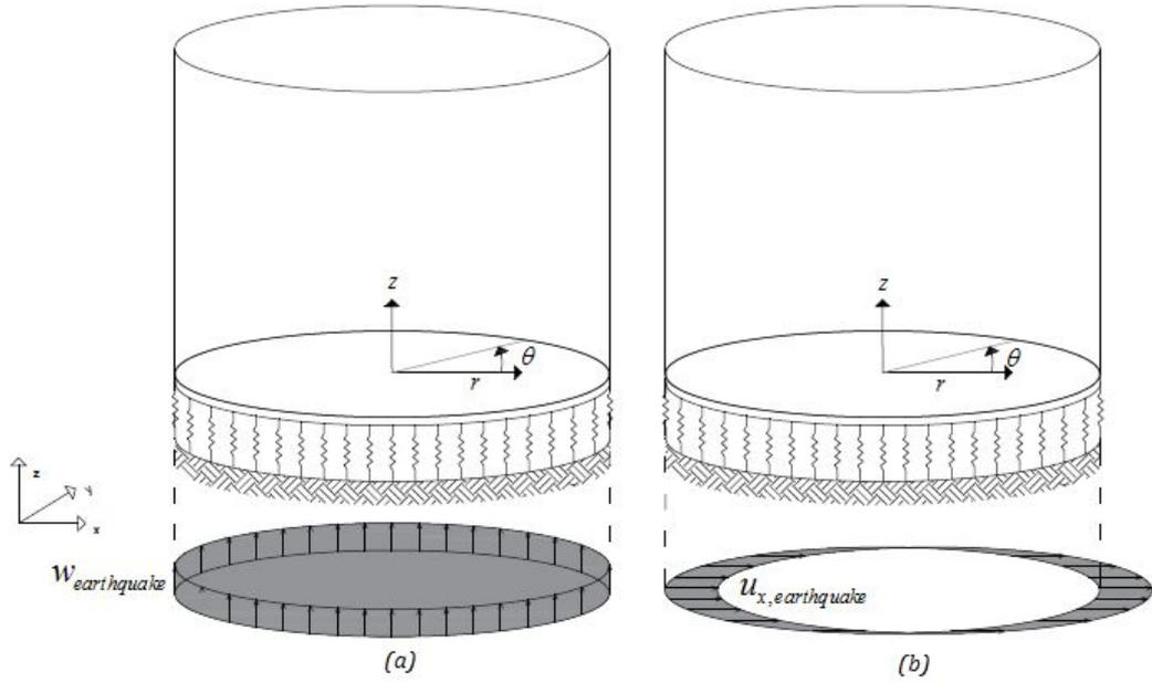
Figure 4.3: The earthquake loading in cylindrical tank. (a) Vertical seismic loading; (b) Horizontal Seismic loading
