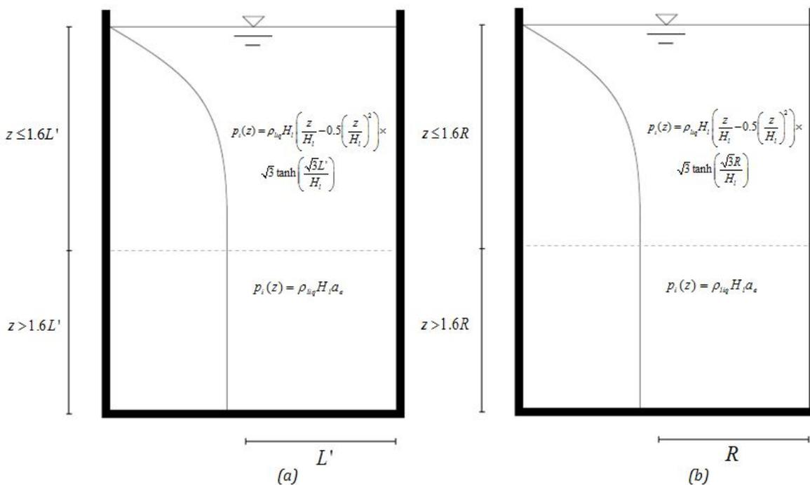
Figure 2.23: Housner correction for tanks with tank geometry ratio  $H/R > 1.6$  or  $H/L' > 1.6$ . (a) Rectangular tank; (b) Cylindrical tank. (Source : The dynamic behaviour of Water Tanks, George W, Housner[7])
