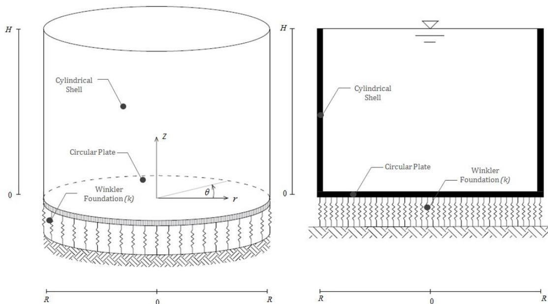
Figure 4.1: The three-dimensional Model, The three dimensional preview (*left*) and cross sectional preview (*right*)
