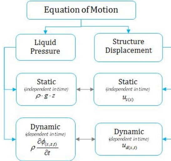
Figure 3.8: Separate analyzing between dynamic and static conditions
