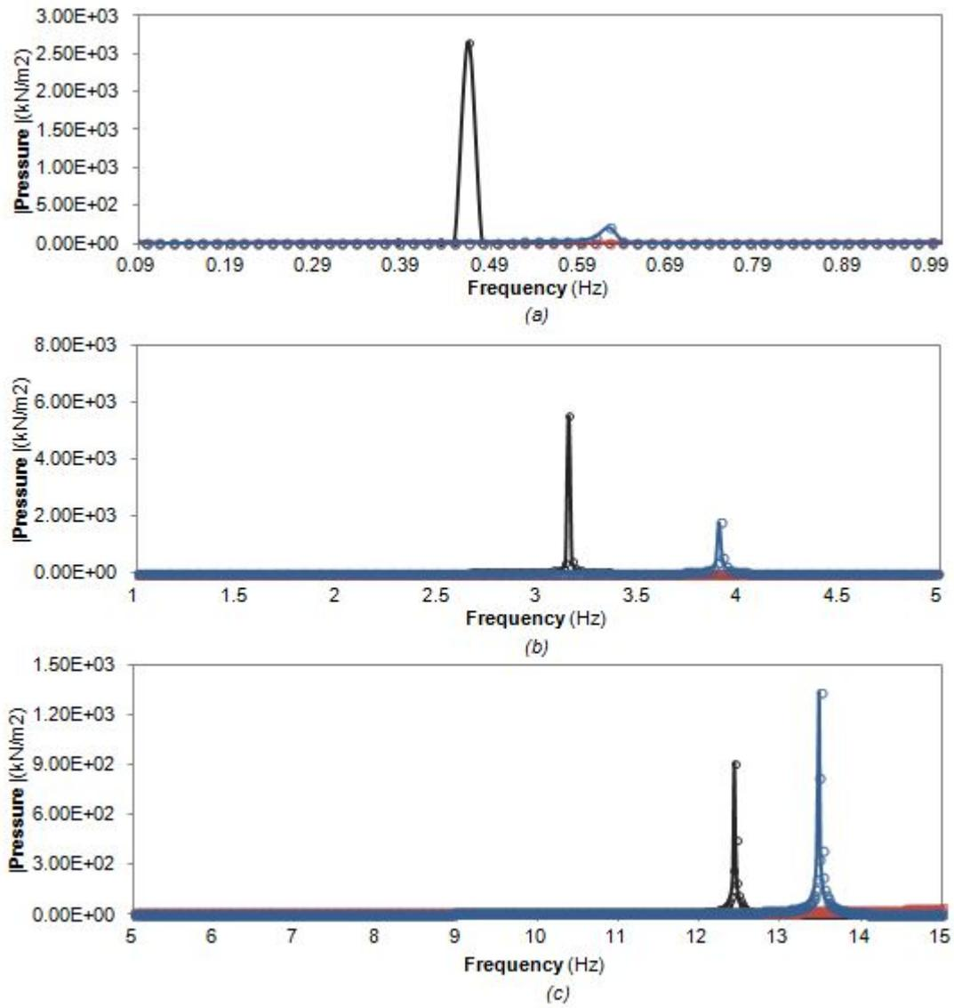
Figure 3.32: Frequency response in term of pressure for different liquid volume under seismic loading in vertical direction: (a) low frequency range;(b) medium frequency range ;(c) high frequency range
