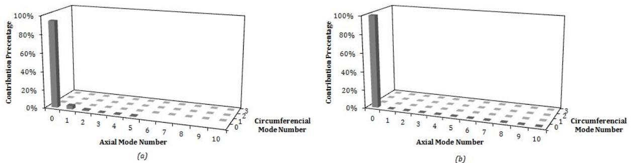
Figure 5.36: Mode contribution under vertical loading before the first resonance peak at (0.4 Hz):
