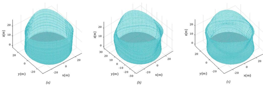
Figure 5.19: Model B mode shape with *circumferential* mode number( $m$ ) = 3 from Matlab, (a) axis mode number 1 ;(b) axis mode number 2 ;(c) axis mode number 3
