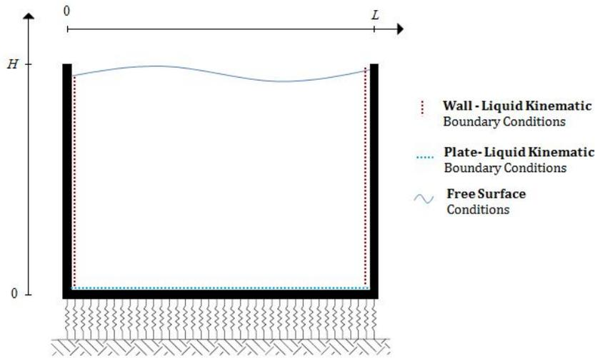
Figure 3.7: Kinematic boundary conditions of the structure with the liquid
