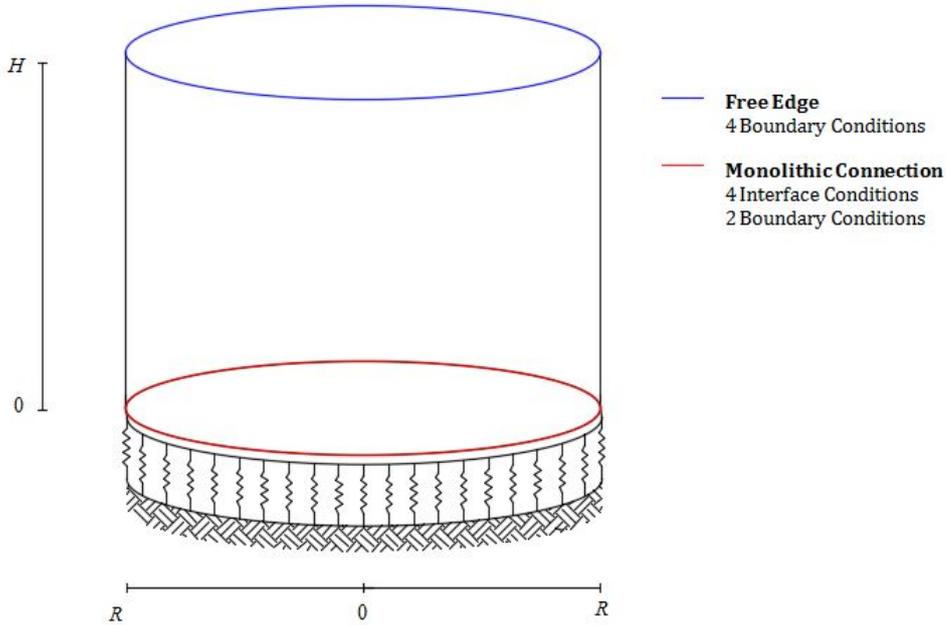
Figure 4.9: Boundary and interface conditions of the cylindrical tank
