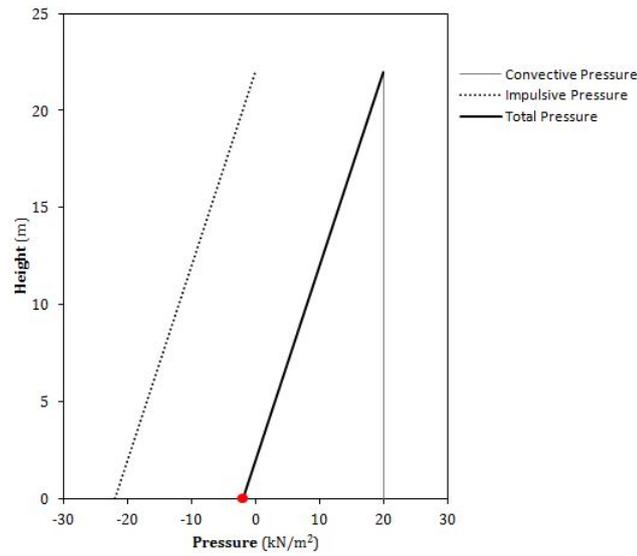
Figure 5.35: Impulsive, convective and total pressure under vertical loading at 1 Hz
