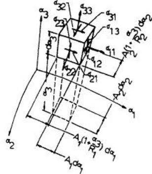
Figure B.3: Stress Acting in the Element
