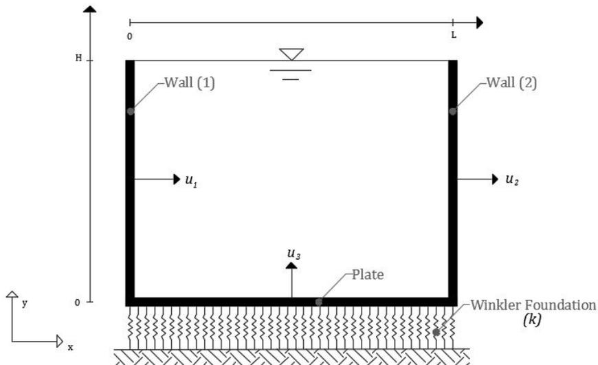
Figure 3.1: Two dimensional Model of the tank
