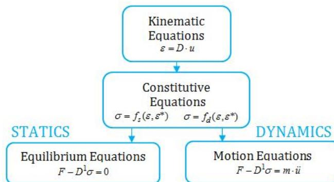
Figure 2.8: The Basic Equation of Statistics and Dynamics
