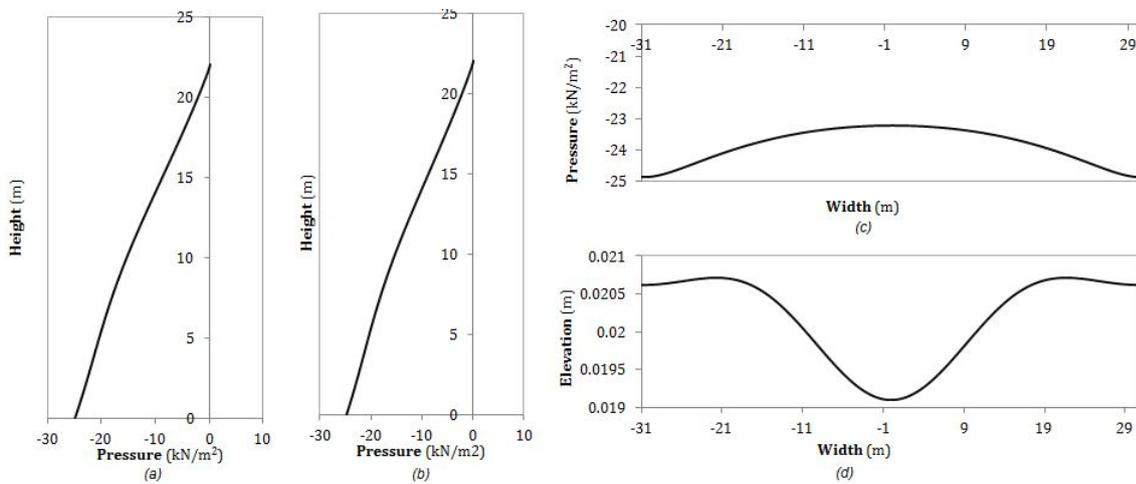
Figure 5.33: Pressure and free surface elevation seismic loading in vertical direction at **1.20 Hz** for Model B: (a) wall Pressure at  $\theta = 0$ ; (b) wall pressure at  $\theta = 2\pi$ ; (c) plate pressure; (d) free surface elevation
