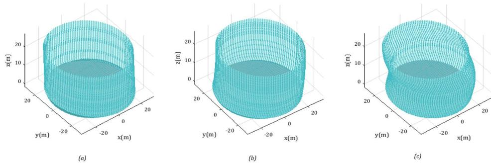
Figure 5.17: Model B mode shape with *circumferential* mode number( $m$ ) = 1 from Matlab, (a) axis mode number 1 ;(b) axis mode number 2 ;(c) axis mode number 3
