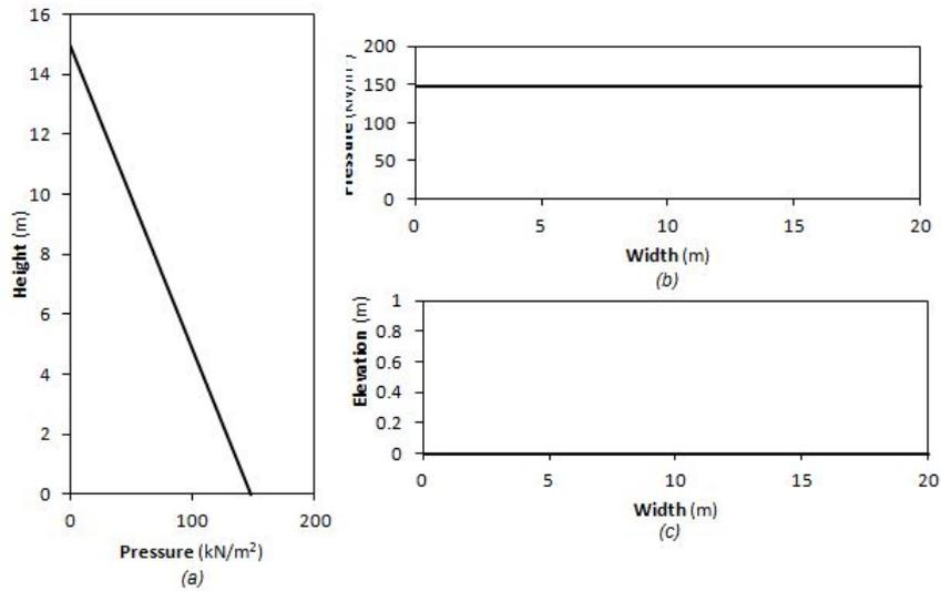
Figure 3.15: Static pressure: (a) wall static pressure; (b) static pressure at  $z=0$ ; (c) free surface elevation at  $z=H$
