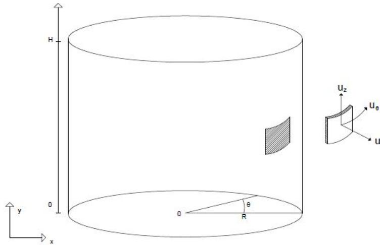
Figure 4.7: Cylindrical Shell axis and degree of freedom
