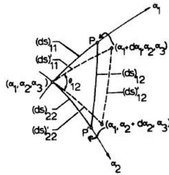
Figure B.4: Shear deformation in plane of the reference surface
