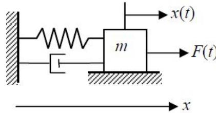
Figure 2.9: Spring and dashpot system
