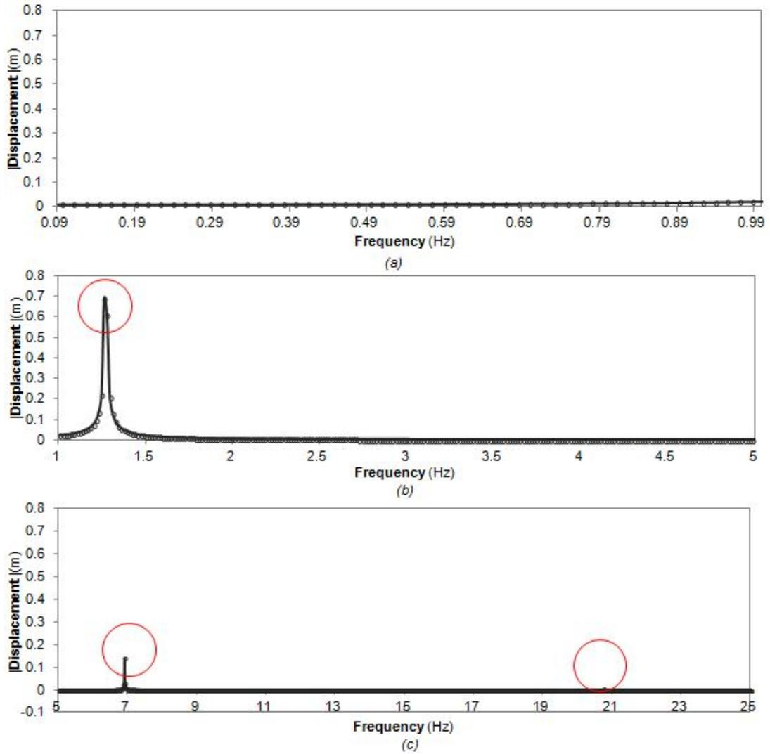
Figure 3.13: Frequency response in term of deformation for empty tank under seismic loading in horizontal direction:
