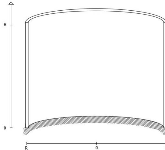
Figure 5.6: The clamped-free cylindrical shell
