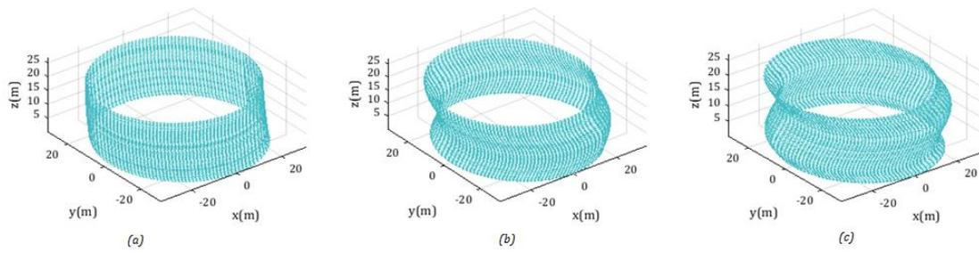
Figure 5.12: Mode shape with *circumferential* mode number( $m$ ) = 1 from Matlab, (a) axis mode number 1 ;(b) axis mode number 2 ;(c) axis mode number 3
