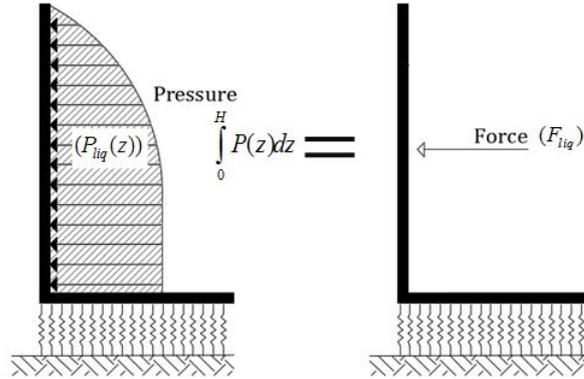
Figure 3.40: Conversion from liquid pressure to force
