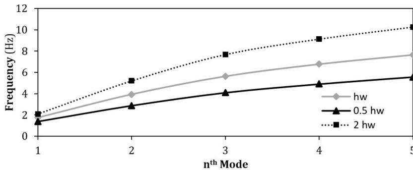
Figure 5.43: Difference natural frequency in for different wall thickness under horizontal loading
