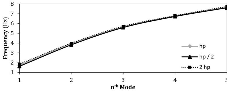
Figure 5.47: Difference natural frequency for different plate thickness under horizontal loading
