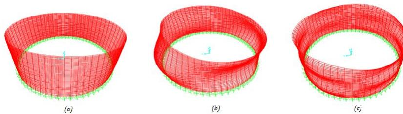
Figure 5.9: Mode shape with *circumferential* mode number( $m$ ) = 2 from SAP 2000, (a) axis mode number 1 ;(b) axis mode number 2 ;(c) axis mode number 3
