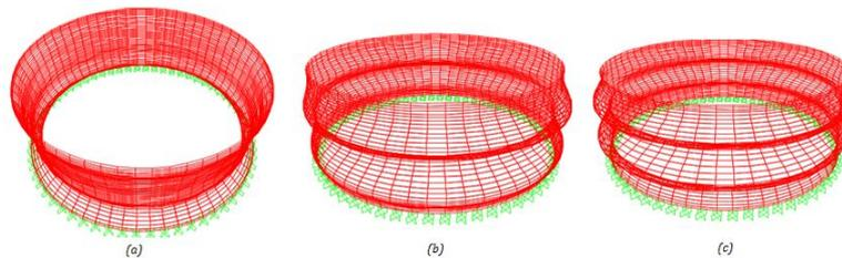
Figure 5.7: Mode shape with *circumferential* mode number ( $m$ ) = 0 from SAP 2000, (a) axis mode number 1 ;(b) axis mode number 2 ;(c) axis mode number 3
