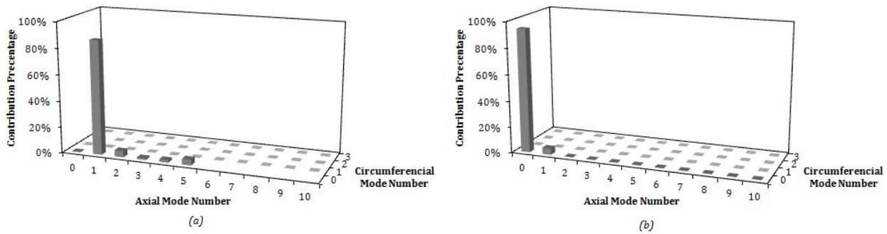
Figure 5.37: Mode contribution under vertical loading at the first resonance peak at (2.55 Hz):
