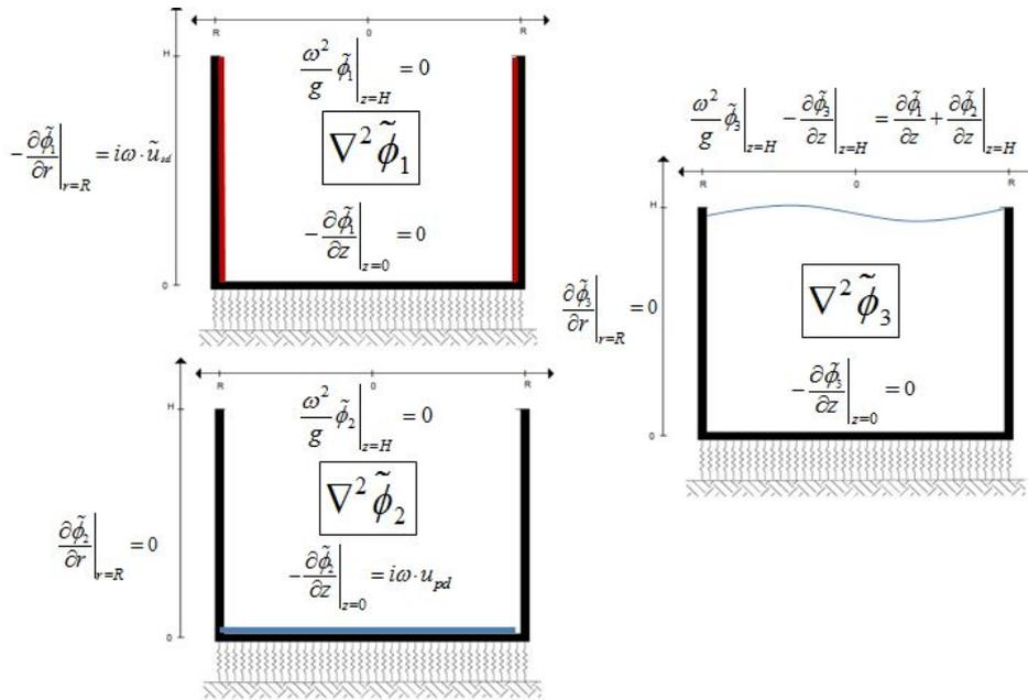
Figure 3.10: Alternative superposition of the fluid potentials
