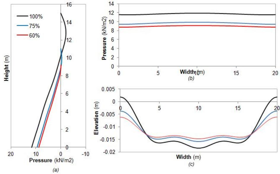
Figure 3.30: Wall Pressure for Liquid Volume Percentage Seismic Loading in z Direction at frequency 1.43 Hz:
