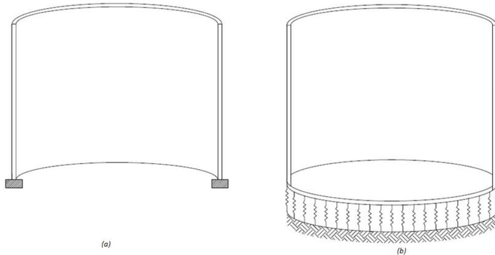
Figure 5.15: The two model that will be used (a) Model A: Clamped Cylindrical Shell; (b) Model B: Cylindrical Shell with Plate
