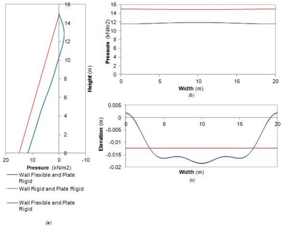
Figure 3.34: Pressure and free surface elevation for different Flexibility Seismic Loading in z Direction at frequency 1.43 Hz:
