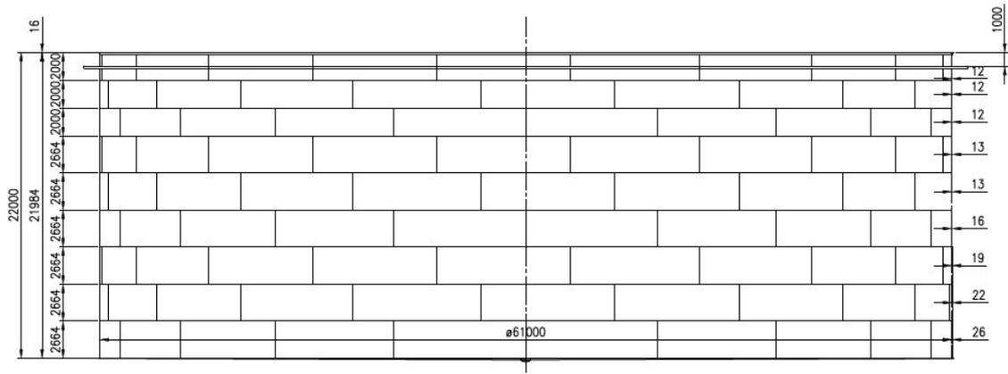
Figure 5.1: Cylindrical shell cross section
