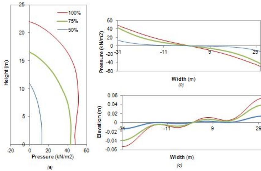
Figure 5.41: Pressure and free surface elevation at 1.97 Hz under horizontal loading: (a) wall pressure at  $\theta = 0$ ; (b) plate pressure; (c) free surface elevation
