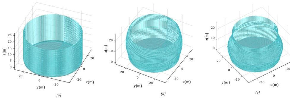
Figure 5.16: Model B mode shape with *circumferential* mode number( $m$ ) = 0 from Matlab, (a) axis mode number 1 ;(b) axis mode number 2 ;(c) axis mode number 3
