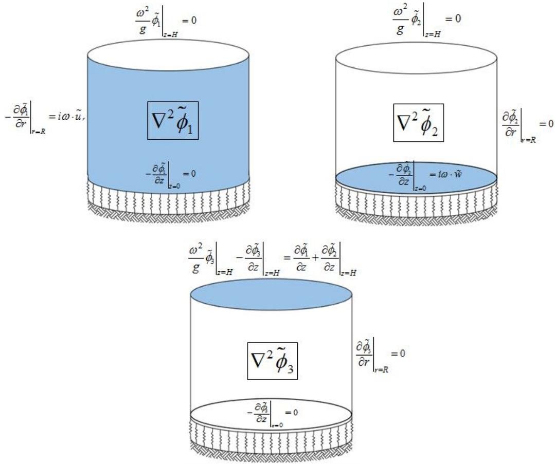
Figure 4.15: Superposition of Liquid in 3D model
