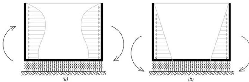
Figure 3.24: Overturning Pressure (a) Horizontal Loading (b) Vertical Loading
