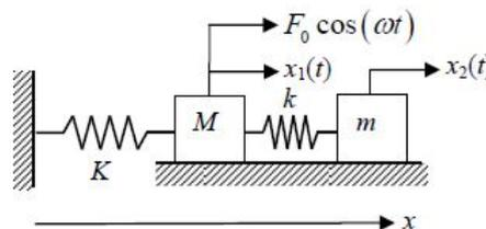
Figure 2.11: The example of multi degree of freedom system
