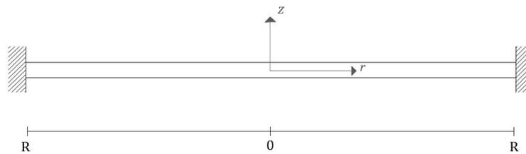
Figure 5.3: Circular plate clamped in the edges
