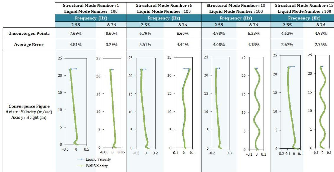
Figure 5.55: The effect of different vacuo-shell mode number to the convergence
