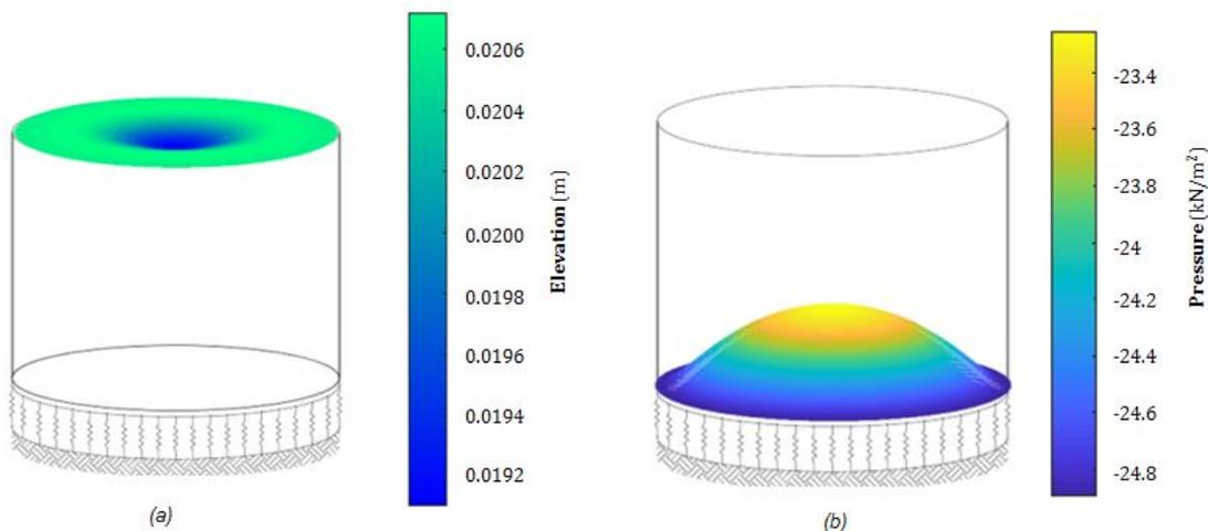
Figure 5.34: Plate pressure and free surface Elevation Seismic loading in vertical direction at **0.700 Hz** in 3D cross section for Model B: (a) free surface elevation; (b) plate pressure
