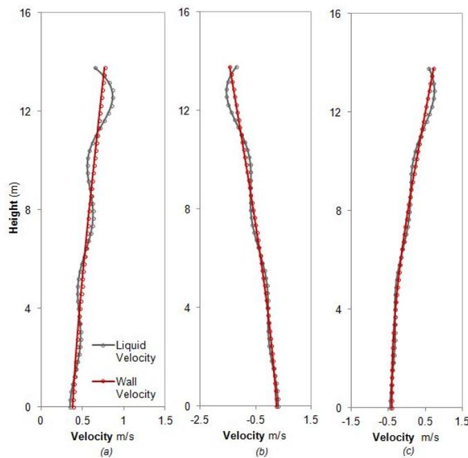
Figure 3.37: Convergence between Wall and liquid velocity for (a) frequency 0.32 Hz ; (b) frequency 0.64 Hz; (c) frequency 1.28 Hz
