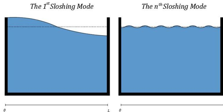
Figure 5.38: The asymmetric sloshing modes : the first sloshing mode (left) and the  $n$  sloshing mode (right)
