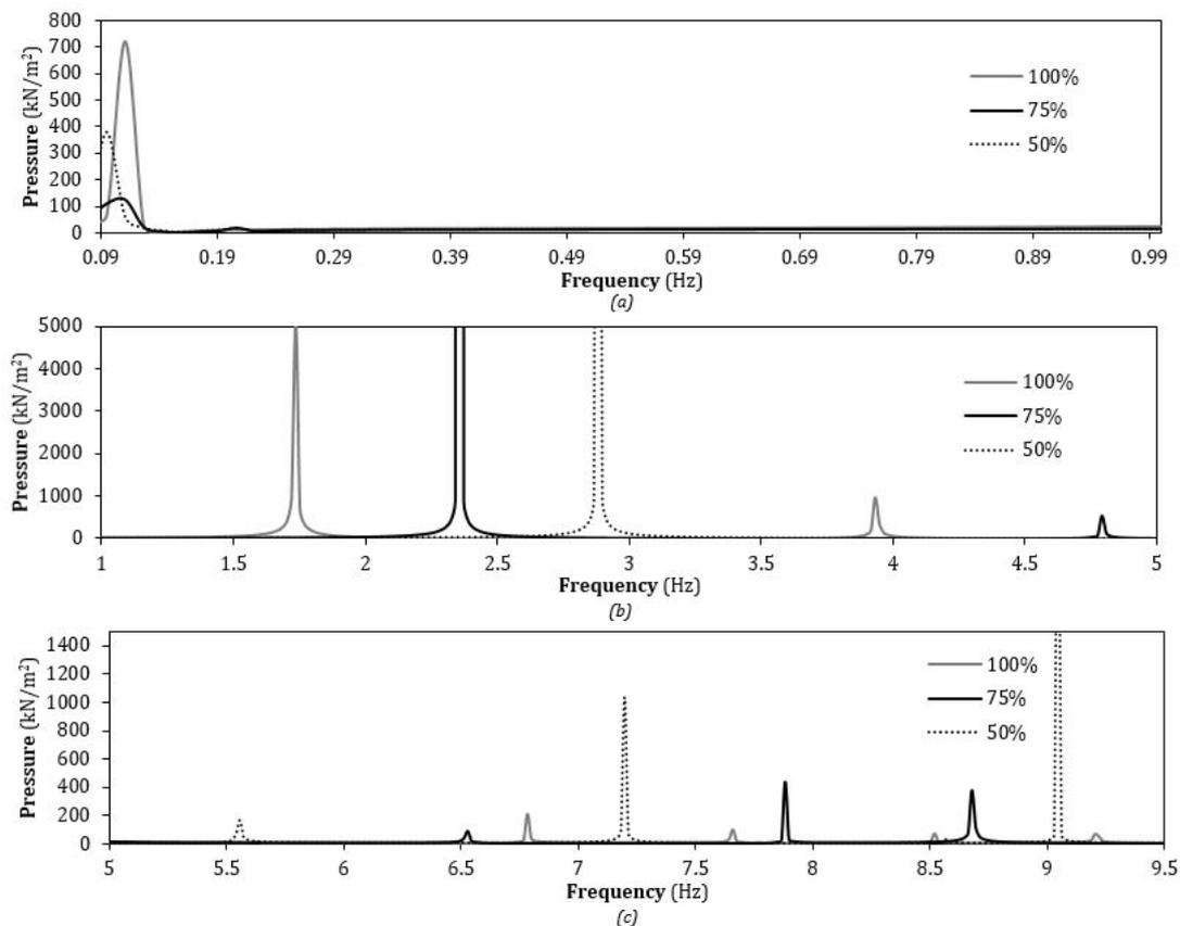
Figure 5.39: Frequency response of the wall pressure for different liquid volume under horizontal loading: (a) low frequency range; (b) medium frequency range; (c) high frequency range
