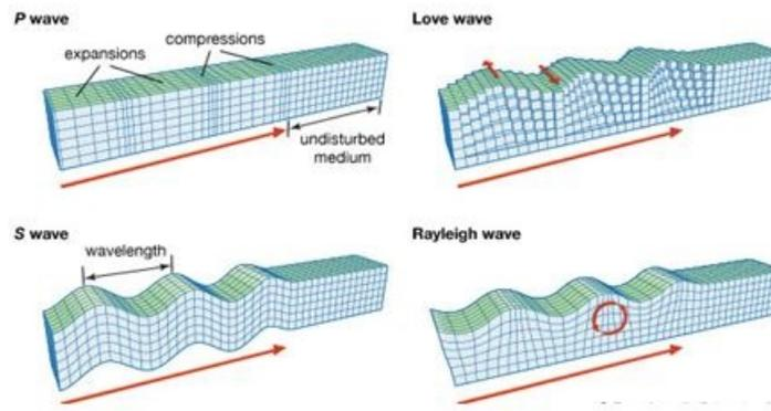
Figure 2.5: Type of wave propagation
