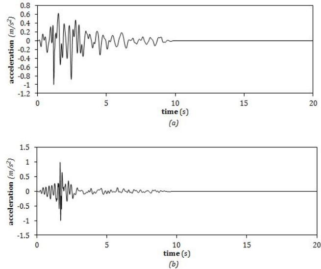
Figure 5.49: Sample of Groningen earthquake acceleration:(a) earthquake acceleration in the horizontal direction (b) earthquake acceleration in the vertical direction
