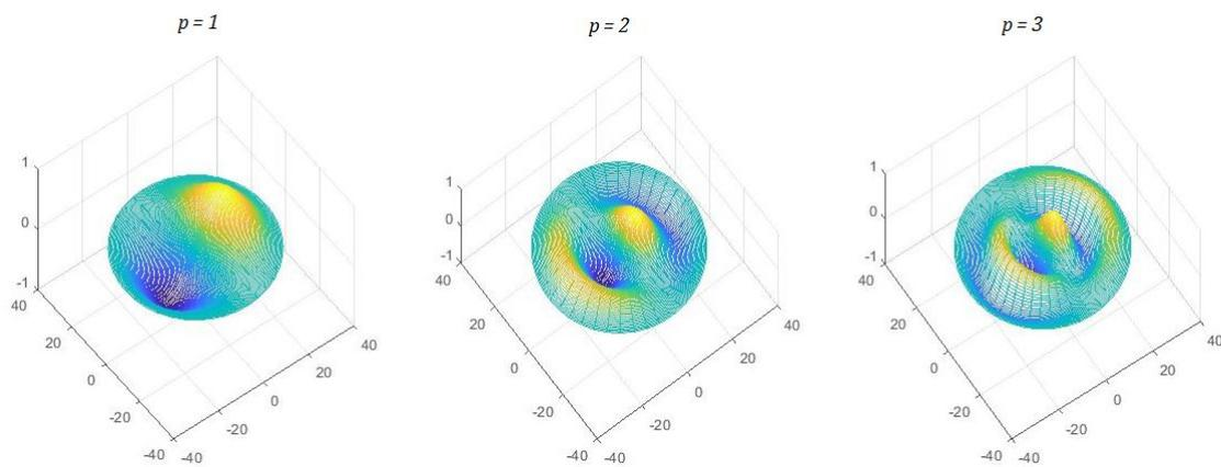
Figure 5.5: Asymmetric mode shape with diametrical mode number ( $p$ ) = 1
