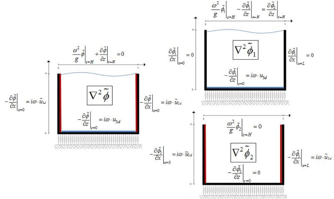
Figure 3.9: Superposition of the fluid potentials
