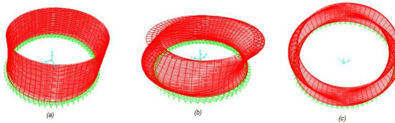
Figure 5.8: Mode shape with *circumferential* mode number( $m$ ) = 1 from SAP 2000, (a) axis mode number 1 ;(b) axis mode number 2 ;(c) axis mode number 3
