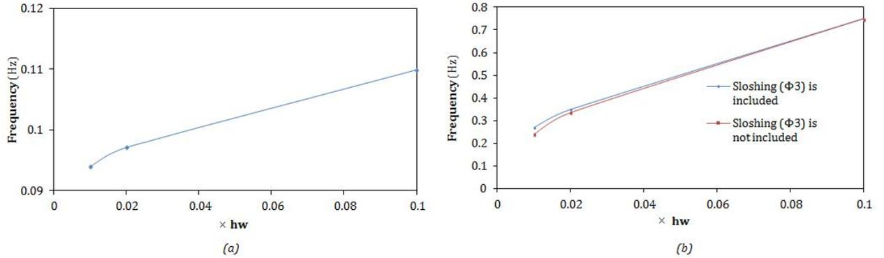
Figure 5.45: Interdependent sloshing and impulsive frequency in a very flexible structure : (a) sloshing frequencies, (b) impulsive frequencies (with and without the sloshing component)
