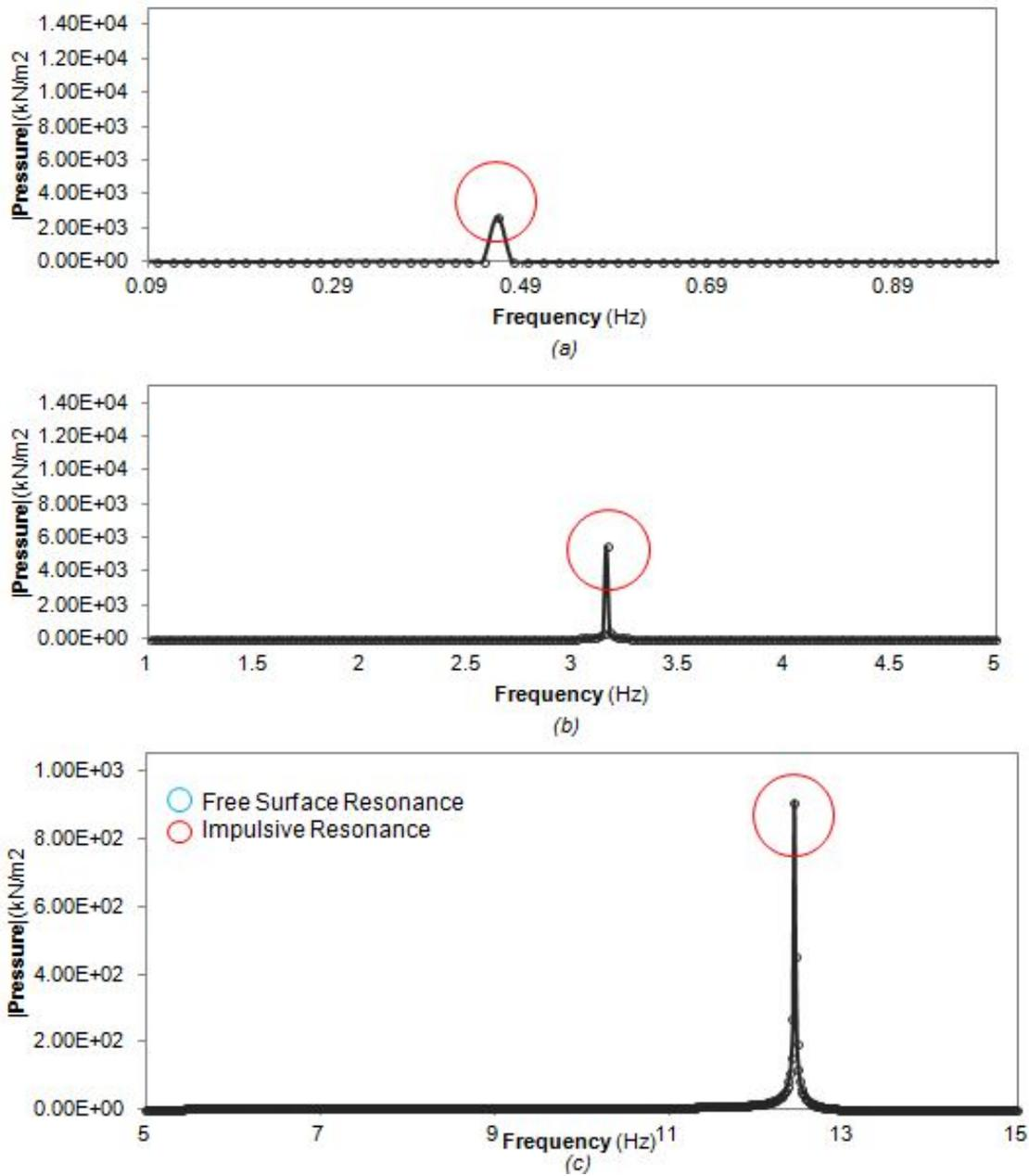
Figure 3.18: Frequency response in term of pressure under seismic loading in vertical direction: (a) low frequency range;(b) medium frequency range ;(c) high frequency range
