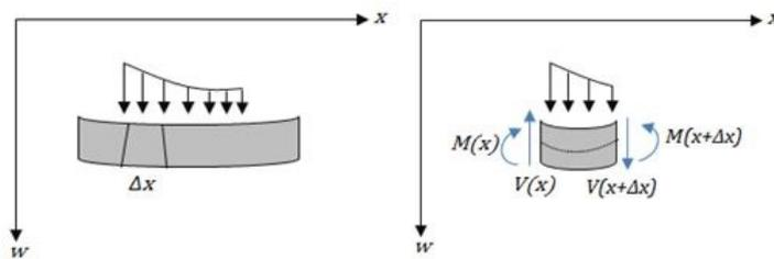
Figure A.1: Beam undergoing transverse motion (*left*) differential element of the beam subject to the shear force bending moment and external load (*right*)
