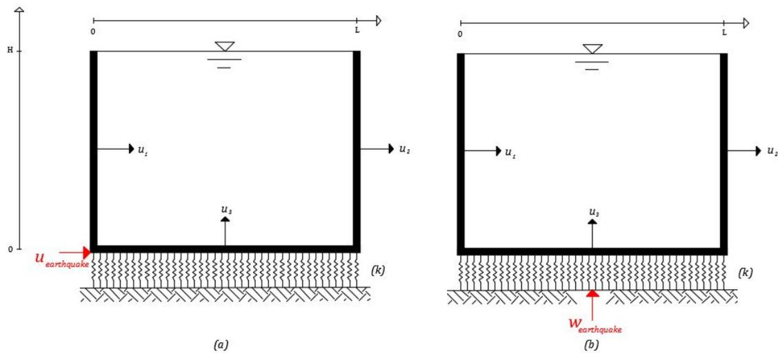
Figure 3.4: Seismic application in the structure. (a) Horizontal seismic loading. (b) Vertical seismic loading
