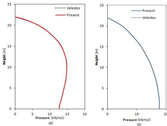
Figure 5.56: Hydrodynamic wall pressure ( $\theta = 0$ ) comparison with Velestos [18] under horizontal loading at the first resonance peak: (a) flexible pressure; (b) rigid pressure
