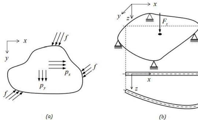
Figure 2.16: In-plane and out of plane loading of a plate: (a) in-plane loading; (b) out of plane loading
