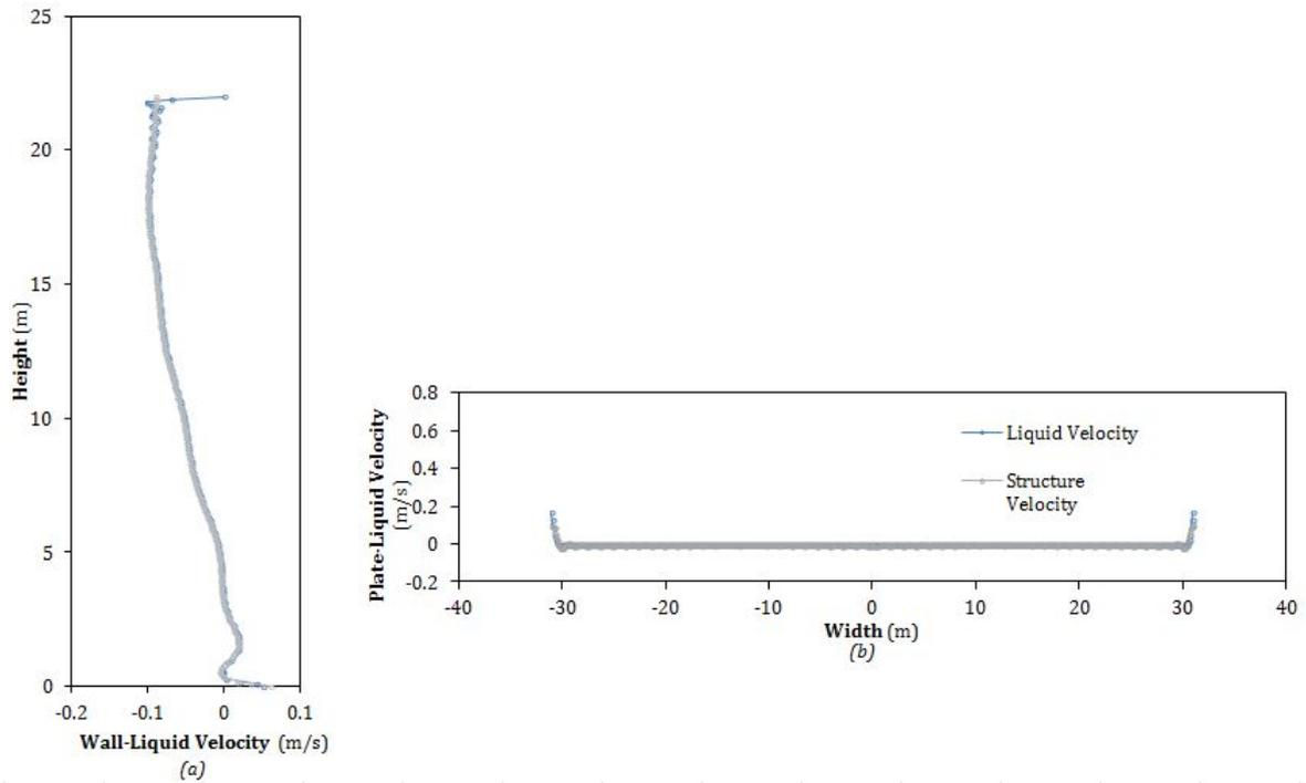
Figure 5.53: Convergence check under horizontal loading at 2.55 Hz : (a) wall convergence at  $\theta = 0$ ; (b) bottom plate convergence
