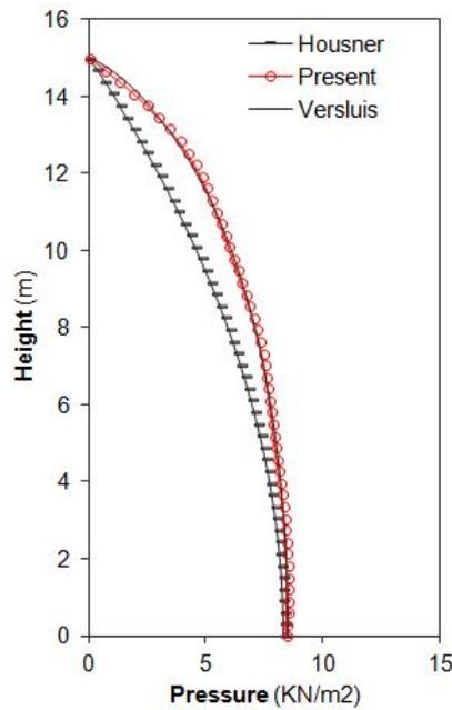
Figure 3.38: Comparison of rigid wall pressure with Housner and Versluis
