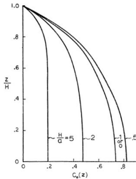
Figure 2.25: Impulsive pressure distribution in rigid tanks
