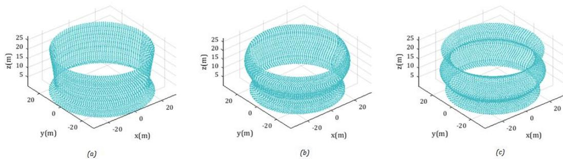
Figure 5.11: Mode shape with *circumferential* mode number( $m$ ) = 0 from Matlab, (a) axis mode number 1 ;(b) axis mode number 2 ;(c) axis mode number 3
