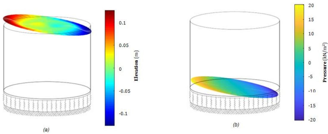
Figure 5.27: Plate pressure and free surface Elevation Seismic loading in horizontal direction at **0.700 Hz** in 3D cross section for Model B: (a) free surface elevation; (b) plate pressure
