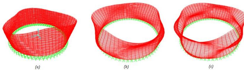
Figure 5.10: Mode shape with *circumferential* mode number( $m$ ) = 3 from SAP 2000, (a) axis mode number 1 ;(b) axis mode number 2 ;(c) axis mode number 3
