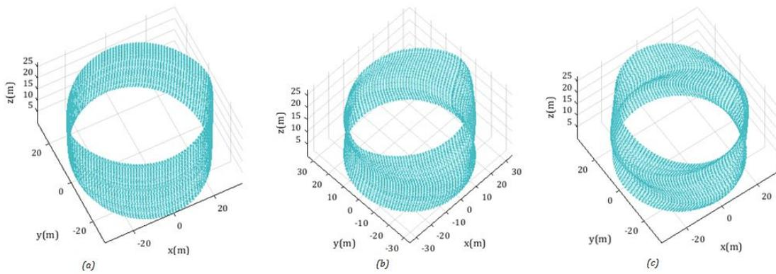
Figure 5.13: Mode shape with *circumferential* mode number( $m$ ) = 2 from Matlab, (a) axis mode number 1 ;(b) axis mode number 2 ;(c) axis mode number 3
