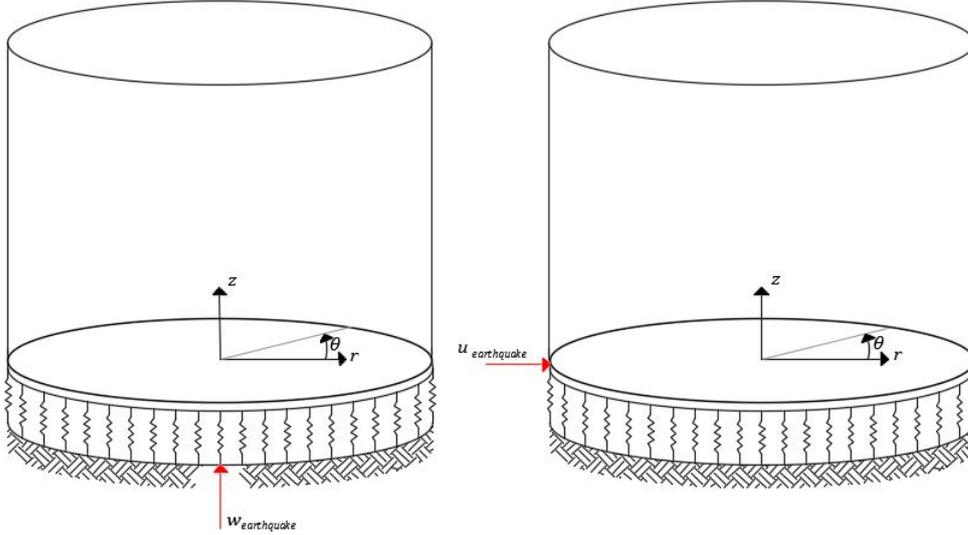
Figure 4.5: The application of seismic loading : vertical seismic loading (left) and horizontal seismic loading (right)
