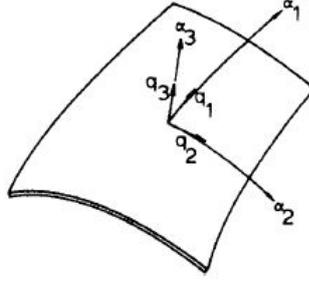
Figure B.7: Distributed loading on the reference surface
