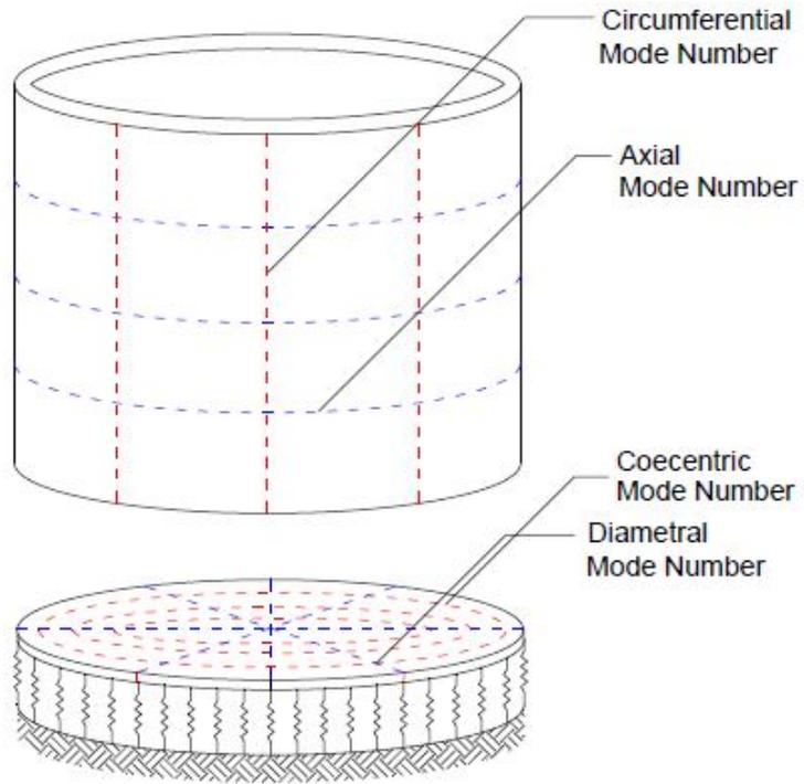
Figure 4.12: Cylindrical Shell and Circular Plate mode number
