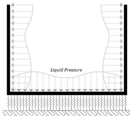
Figure 3.5: The positive direction of the liquid pressure
