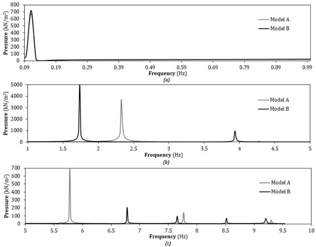
Figure 5.21: Frequency response of Model A and Model B wall pressure in term of pressure under horizontal loading: (a) low frequency range; (b) medium frequency range; (c) high frequency range
