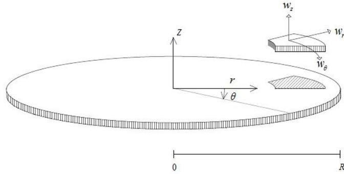
Figure 2.17: Circular slab coordinate
