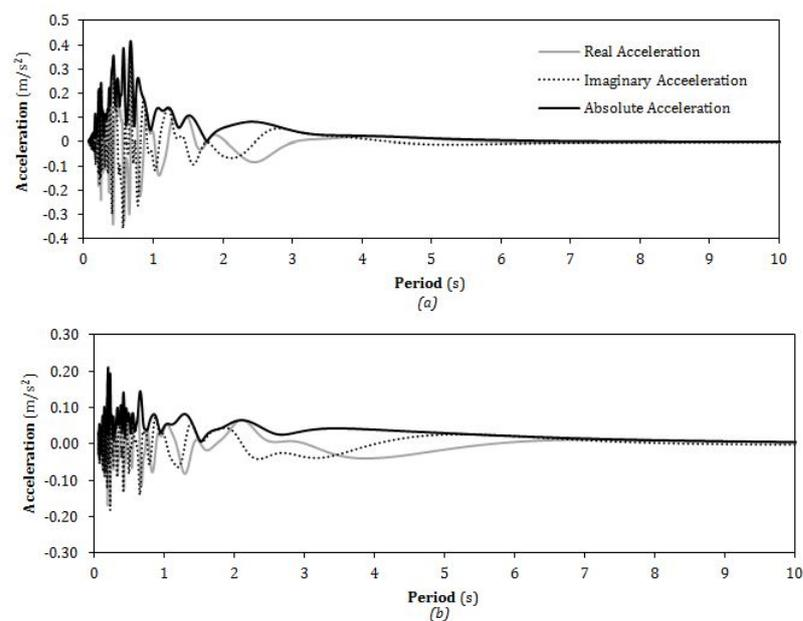
Figure 5.50: Groningen earthquake acceleration in frequency domain
