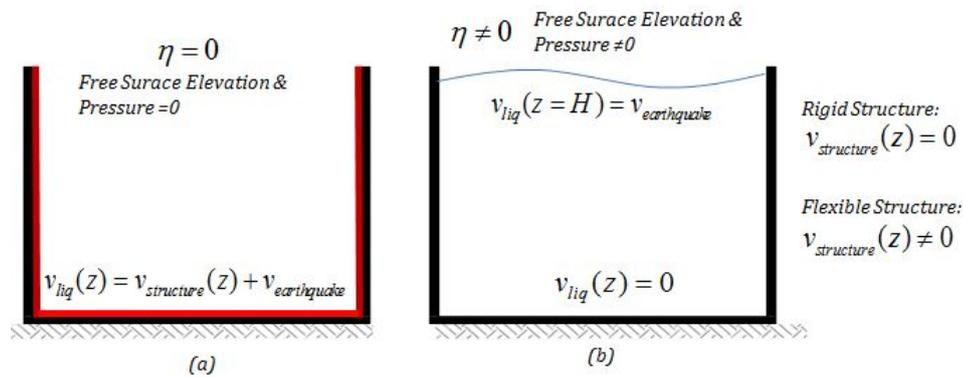
Figure 2.19: The boundary conditions of the impulsive response (a); the boundary conditions of the convective responses (b).
