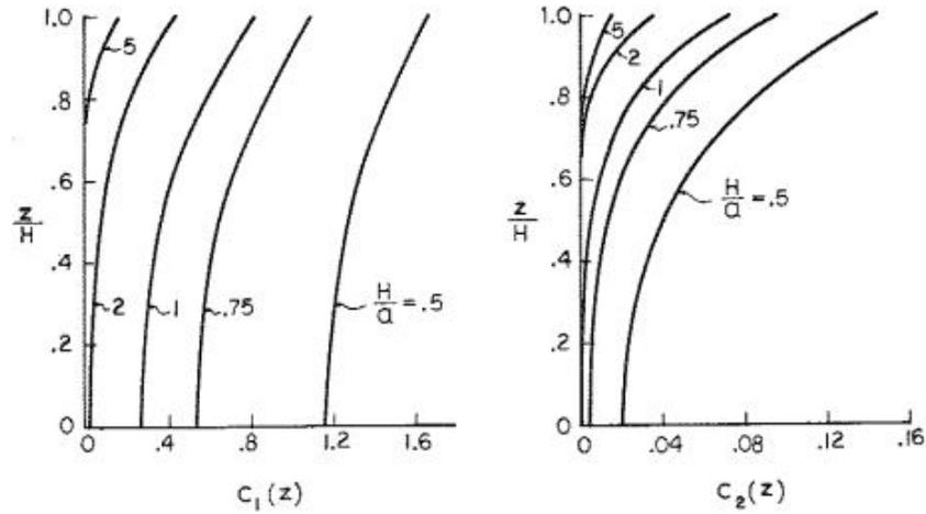
Figure 2.26: Coefficient  $c_k(z)$  for convective pressure in rigid Tanks
