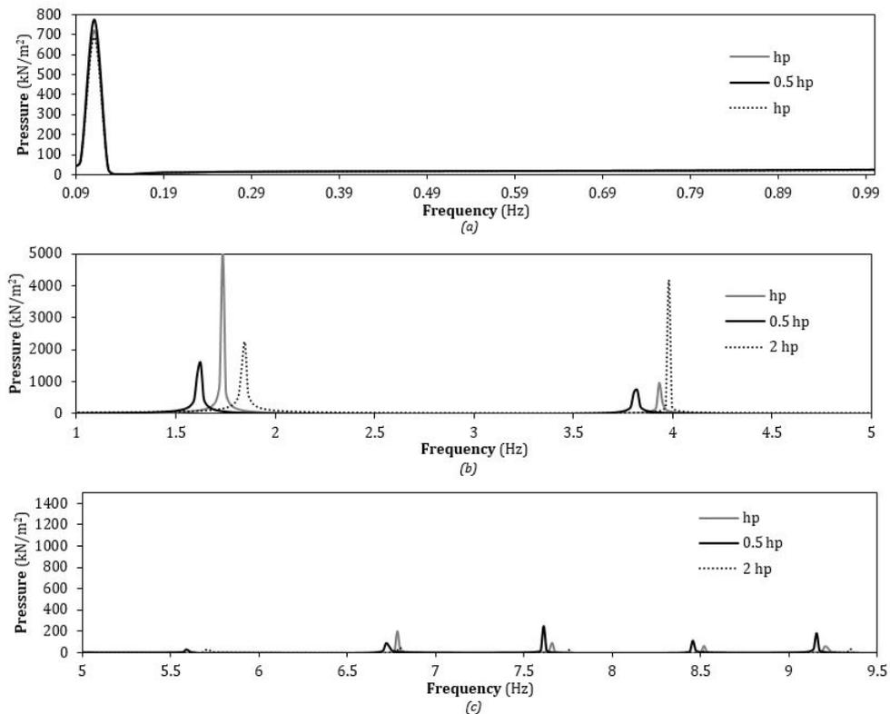
Figure 5.46: Frequency response of pressure for different plate thickness under horizontal loading: (a) low frequency range; (b) medium frequency range; (c) high frequency range
