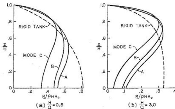
Figure 2.27: Flexible and Rigid Tanks pressure
