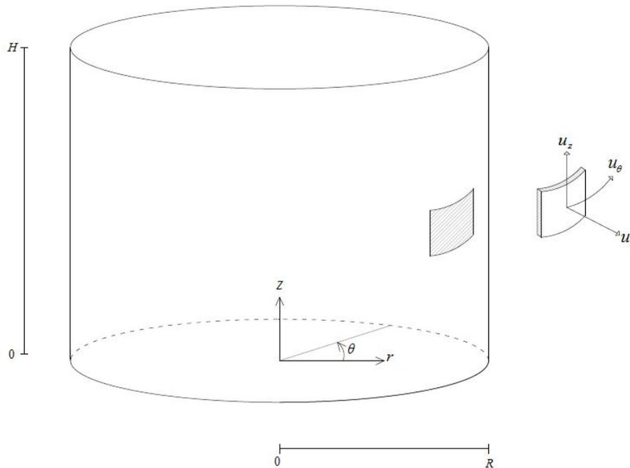
Figure 2.18: Cylindrical shell coordinate
