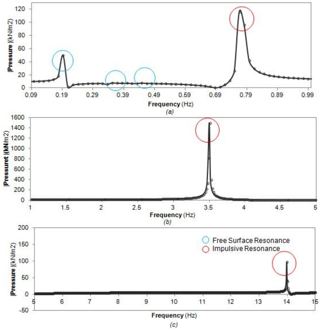
Figure 3.17: Frequency response in term of pressure under seismic loading in horizontal direction:
