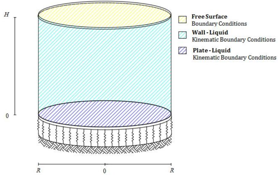
Figure 4.11: Structure and Liquid boundary conditions
