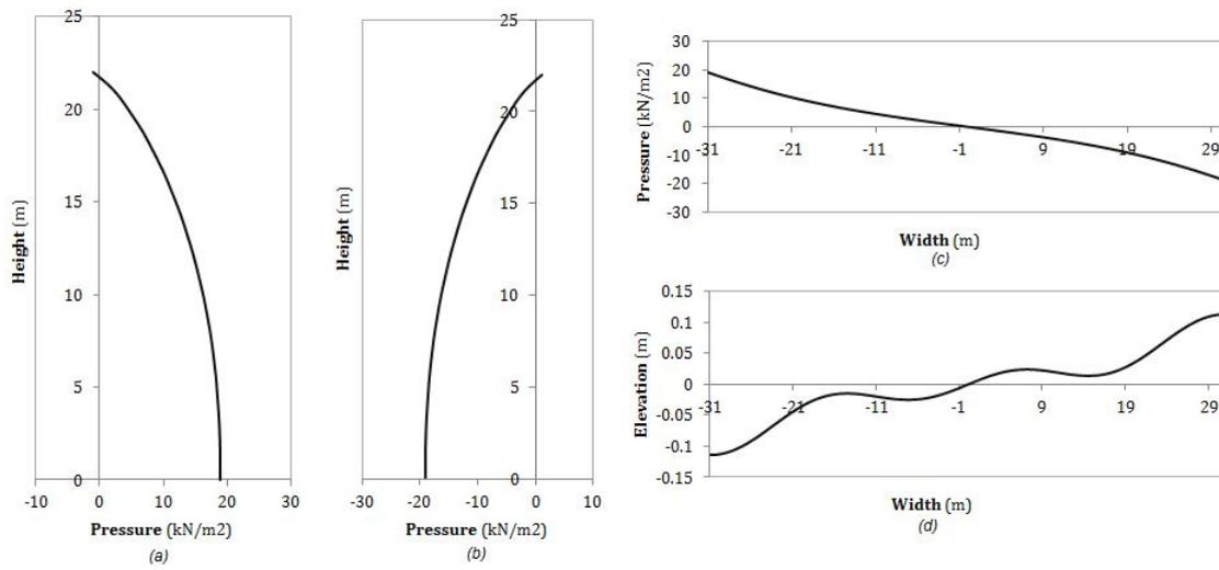
Figure 5.26: Pressure and free surface elevation seismic loading in horizontal direction at **0.700 Hz** for Model B: (a) wall pressure at  $\theta = 0$ ; (b) wall pressure at  $\theta = \pi$ ; (c) plate pressure; (d) free surface elevation
