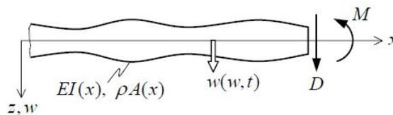
Figure 2.12: The bending beam system
