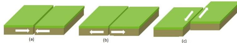
Figure 2.2: Tectonic plate motion: (a) convergent boundaries; (b) divergent boundaries; (c) transform boundaries
