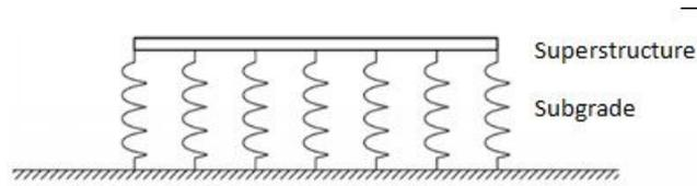
Figure 2.7: Visualization of a structural Winkler Model
