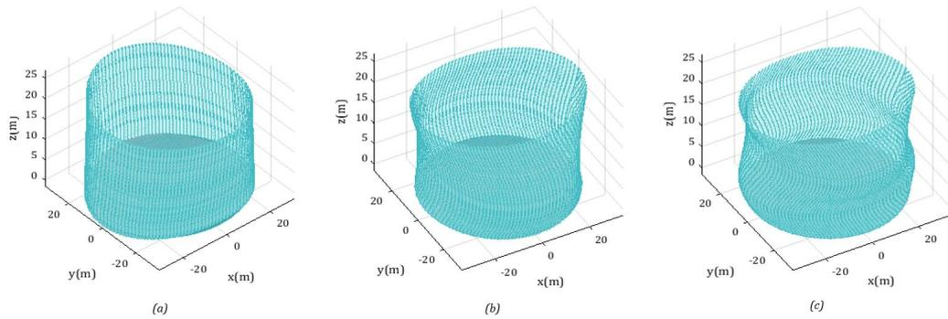
Figure 5.18: Model B mode shape with *circumferential* mode number( $m$ ) = 2 from Matlab, (a) axis mode number 1 ;(b) axis mode number 2 ;(c) axis mode number 3
