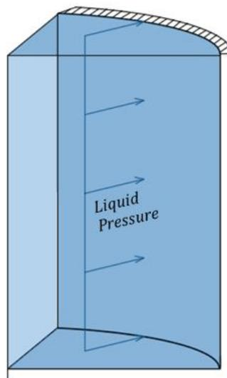
Figure 4.8: Liquid Pressure in the cylindrical container
