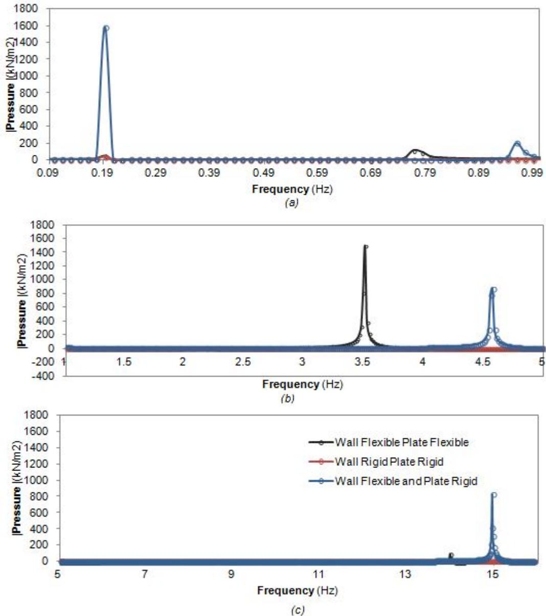
Figure 3.31: Frequency response in term of pressure for different flexibility under seismic loading in horizontal direction: (a) low frequency range;(b) medium frequency range ;(c) high frequency range
