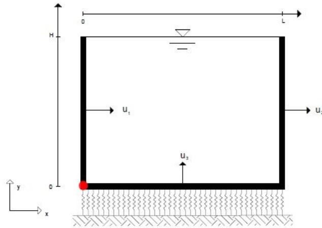
Figure 3.16: Location of the referred point for response pressure plotting
