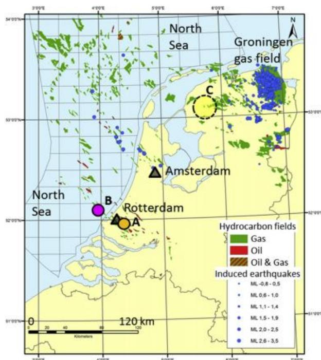
Figure 2.3: The Netherlands earthquake and gas extraction
