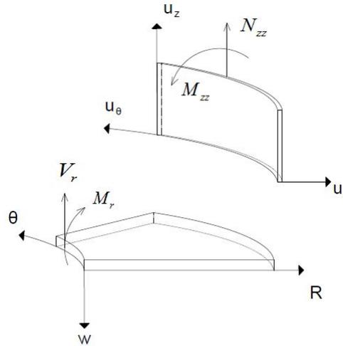
Figure 4.10: Infinitesimal connection between plate and shell with respect to normal/shear force and bending moment
