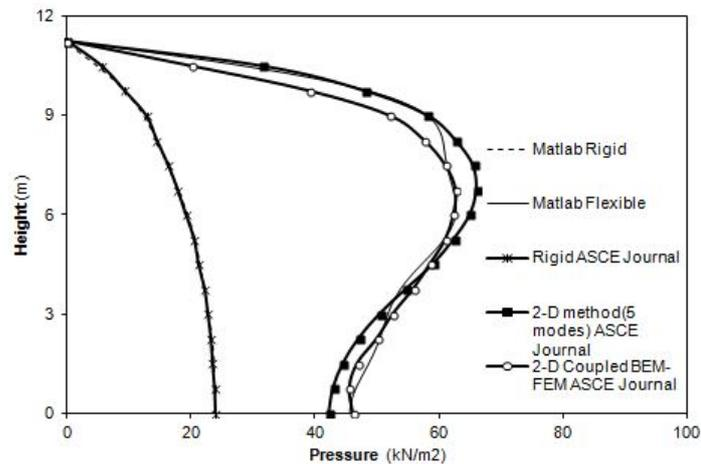
Figure 3.39: Pressure Comparison with other journals (a) Seismic Pressure at 0.3184 Hz, and (b) 0.614 Hz
