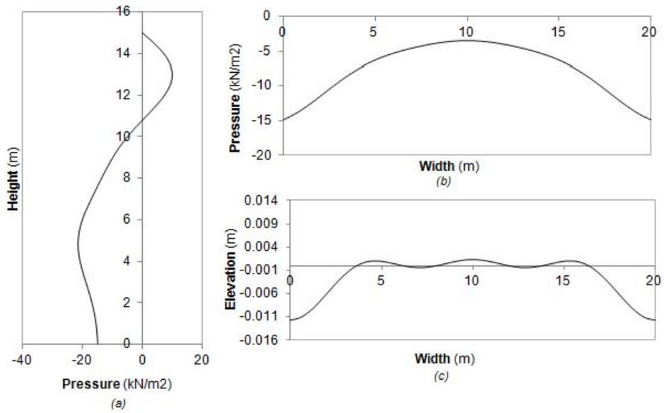
Figure 3.23: Pressure and free surface elevation seismic loading in z direction at 3.425 Hz:
