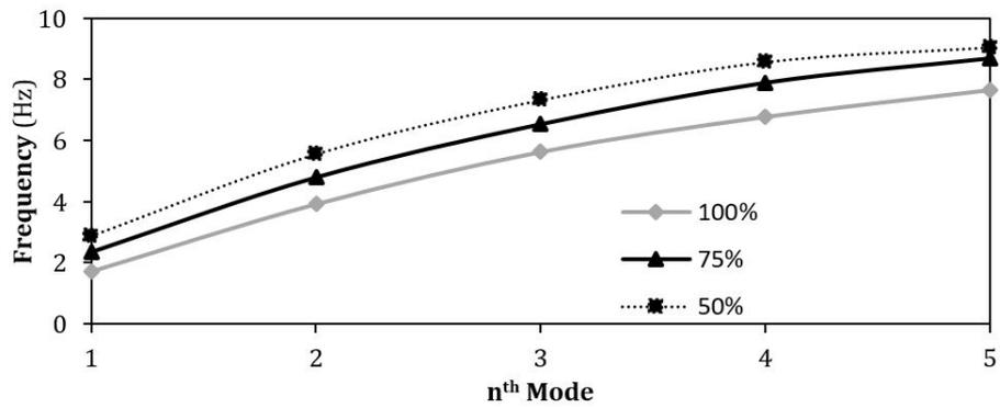
Figure 5.40: Frequency difference for different liquid volume frequency under horizontal loading
