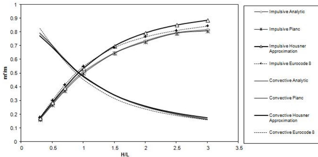
Figure 3.41: Impulsive and Convective Mass ratio for Rigid Tank
