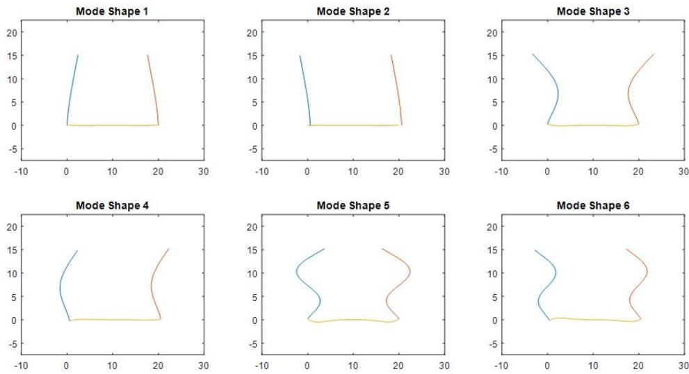
Figure 3.11: The mode shape of the empty tank
