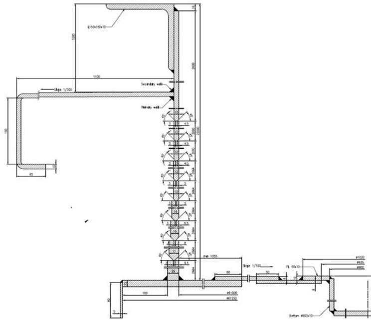
Figure 5.2: Dimension of the wall and bottom plate
