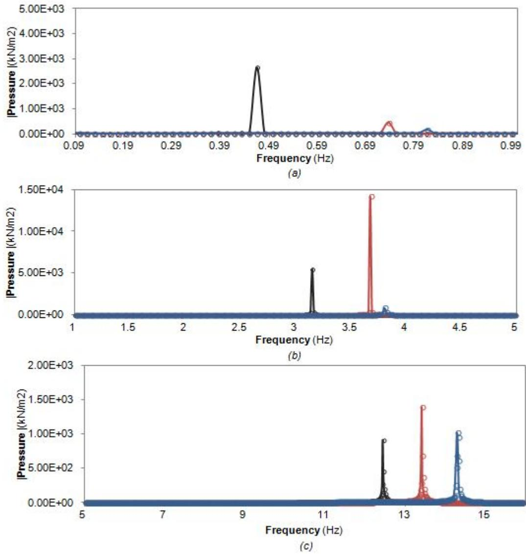
Figure 3.26: Frequency response in term of pressure for different liquid volume under seismic loading in vertical direction:
