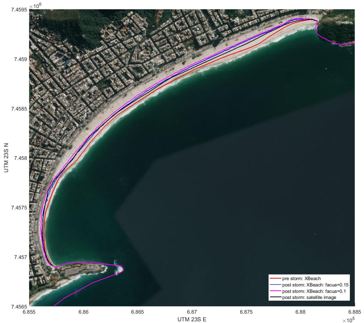
Figure 54: The post storm coastline position resulting from the XBeach model for facua=0.1 and facua=0.15 .
