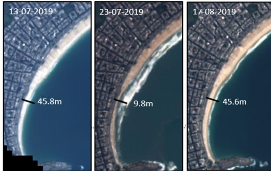
Figure 20: Sentinel 2 satellite images before, directly after and 4 weeks after the July 2019 extreme wave event showing the beach width at the Southern part of the beach.
