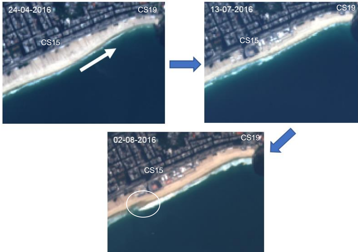
Figure 18: Three satellite images showing an alongshore redistribution of sediment in the Northern part of the beach. The transport direction is denoted with the white arrow.
