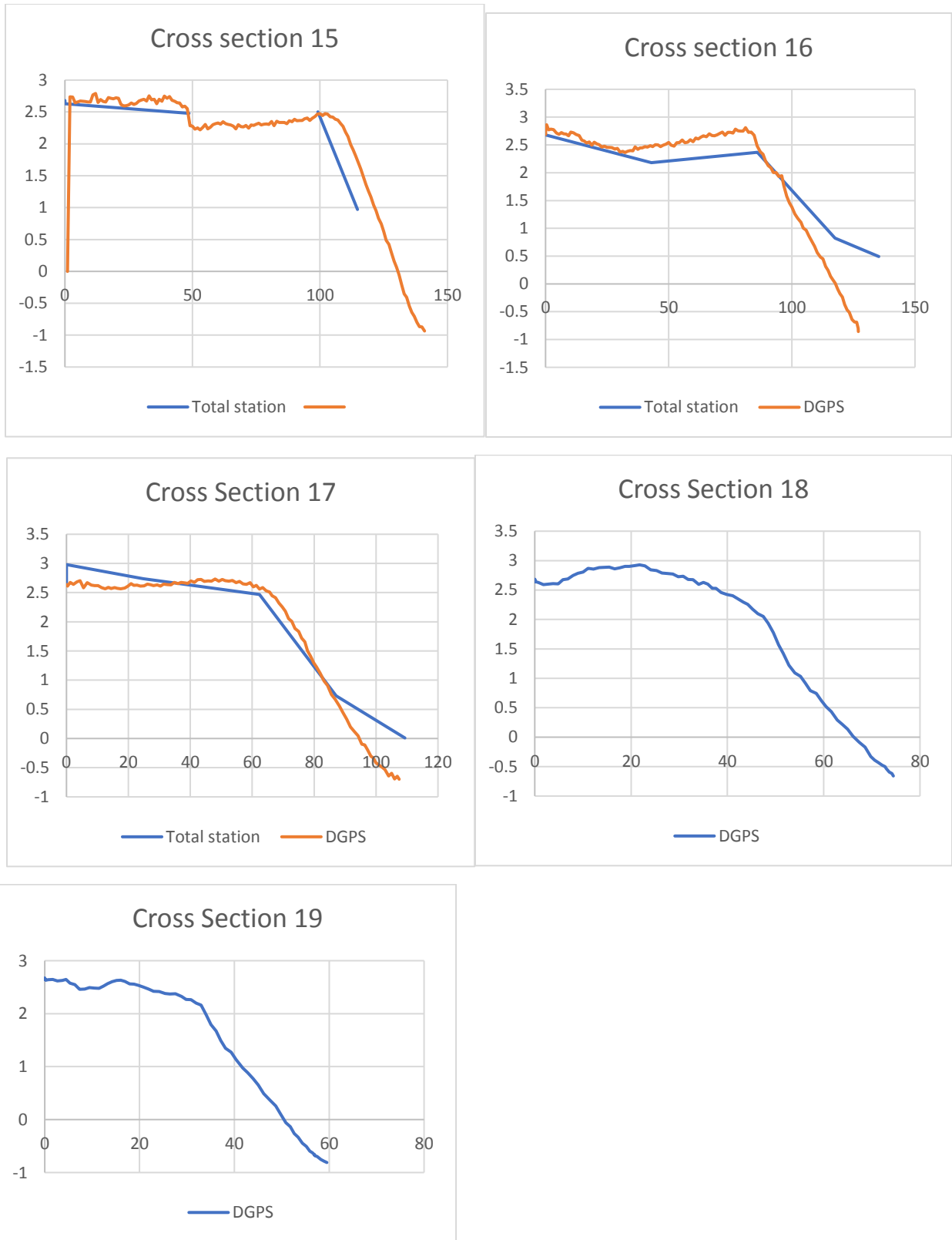
Figure 98: 19 different cross section measurements performed with a total station on 18-12-2019 and with a DGPS device on 04-12-2019. Mean Sea Level is at 0 meters on the vertical axis.
