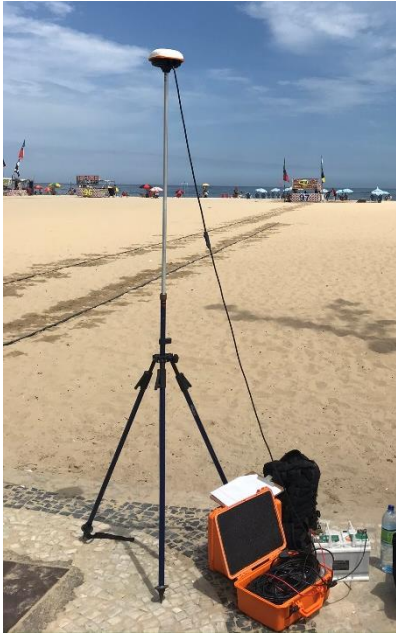
Figure 96: DGPS instrument used for the profile measurements.
