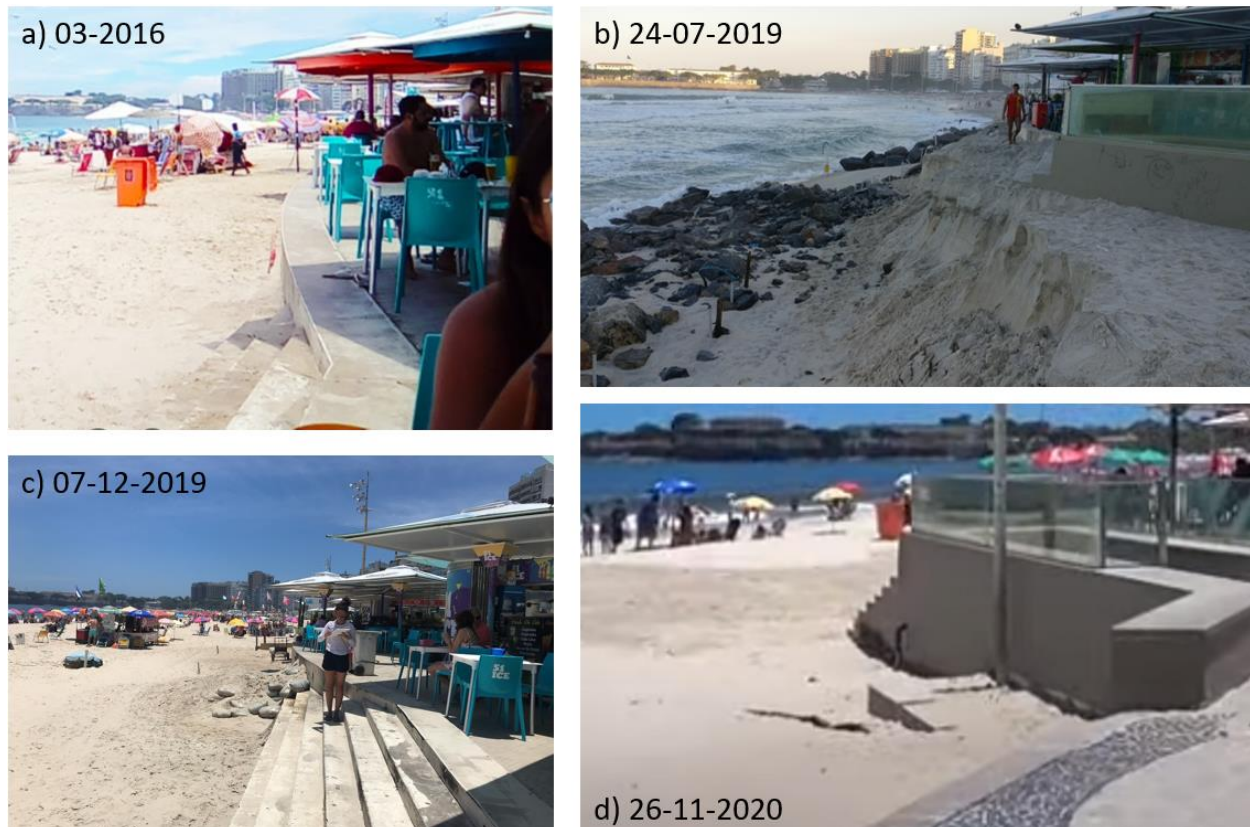
Figure 34: The set of pictures are taken of the same beach kiosk along Copacabana beach showing variations in backbeach elevation. Number of steps visible above the vertical beach level for every image: a) 2.5, b) 2, c) 7 and d) 6/7. Courtesy of Google maps and Han Winterwerp.
