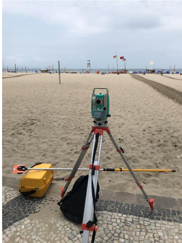
Figure 97: Total station used to perform cross section measurements on the beach.
