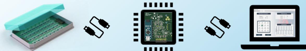
Fig 4. a) 3D model of the array of EHT platforms in the multi-well plate format; b) custom-made bipolar pulse generator; c) user interface of the app for control of the stimulation
