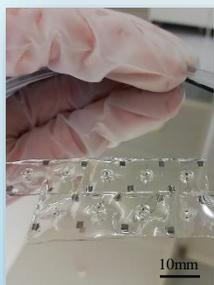
Fig 5. Fabricated EHT platforms with electrodes
