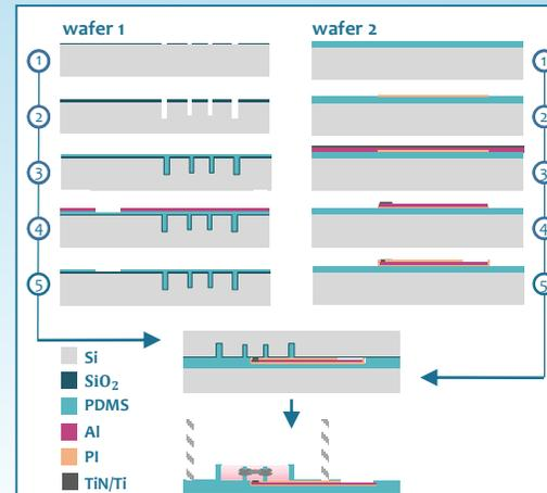
Fig 3. Process flow of the microfabrication
