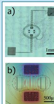
Fig 2. a) Top view of the EHT platform with TiN electrodes; b) FEM simulation of the electric field distribution
