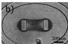
Fig 1. a) 3D model of the EHT platform with integrated electrodes; b) top view of the tissue formed in the EHT platform
