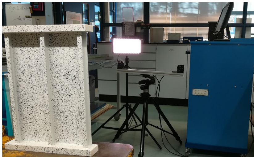
Figure 3: DIC measurement setup.
