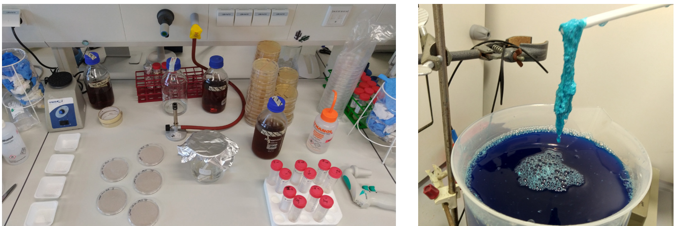
figure 27: Overview of an experimental set-up (left) and the isolation of P.G.A. using \text{CuSO}_4 (blue) on the right.
