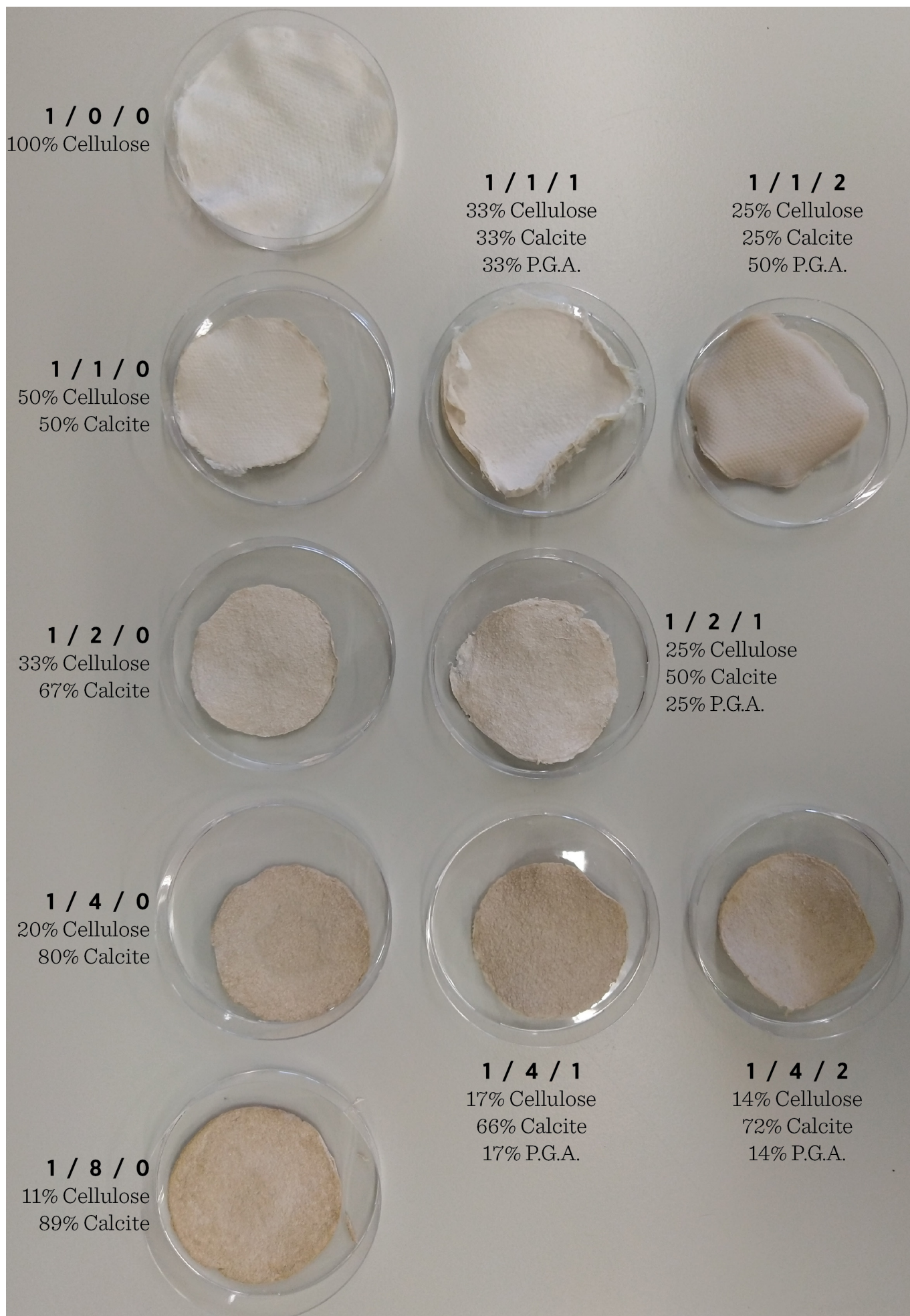
figure 28: Samples with varying ingredient ratios, not that the percentages are an approximation.
