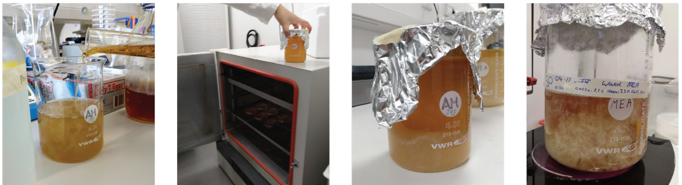
Figure 20: Overview of the calcification procedure by the Sporosarcina Pasteurii .
