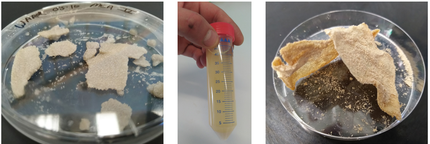
Figure 24: Different materials combined with Bacterial Calcite, from left; Sand, Chitosan, Unblended cellulose mat
