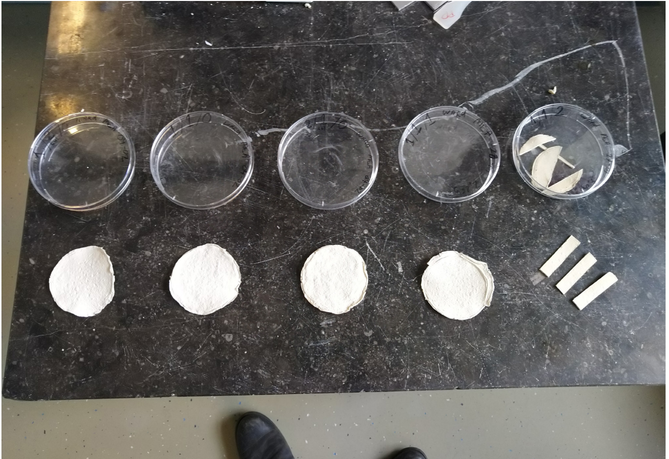
figure 38: The material samples used for the 3P bending test
