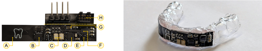
Fig. 4. Densor implementation. Left image—fabricated PCB before insertion into aligner: Ⓐ PCB antenna, Ⓑ STMicroelectronics ST25DV64K NFC tag [123], Ⓒ Seiko CPH3225A chip capacitor bank [112], Ⓓ Abracon AB1805 RTC [2], Ⓔ STMicroelectronics LIS2DW12 accelerometer [121], Ⓕ STMicroelectronics STM32L021F4 MCU [120], Ⓖ Vishay VEMD1060X01 photodiode [130], Ⓗ programming port (which is cut off before embedding in a dental aligner). Right image—example of a fully assembled Densor, i.e. fitted into a dental aligner.
