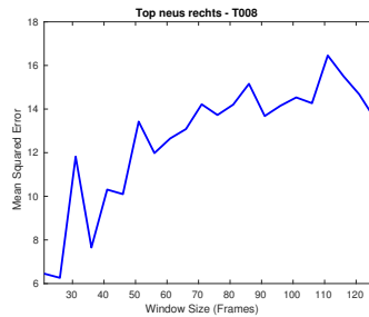
Figure 3.12: MSE vs Window size - T008 'Top neus rechts'. If a large motion is estimated by the Eulerian approach, the MSE increases with the window size.
