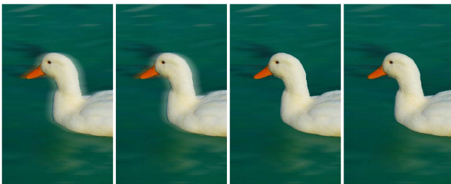
Fig. 20. Comparison with Photoshop tools for the background motion blur. From left to right, Photoshop results using Motion Blur, Path Blur, Content Aware Fill with layer compositing, and our approach. (Image source: pixabay.com).
