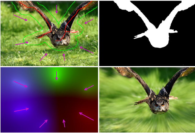
Fig. 6. Multi-directional motion blur. Top row: the input image with user scribbles and multiple motion paths (left) and the segmentation mask (right). Bottom row: the diffusion map M with the colors encoding the direction and length of each motion path (left), and the final result (right). (Image source: pixabay.com).
