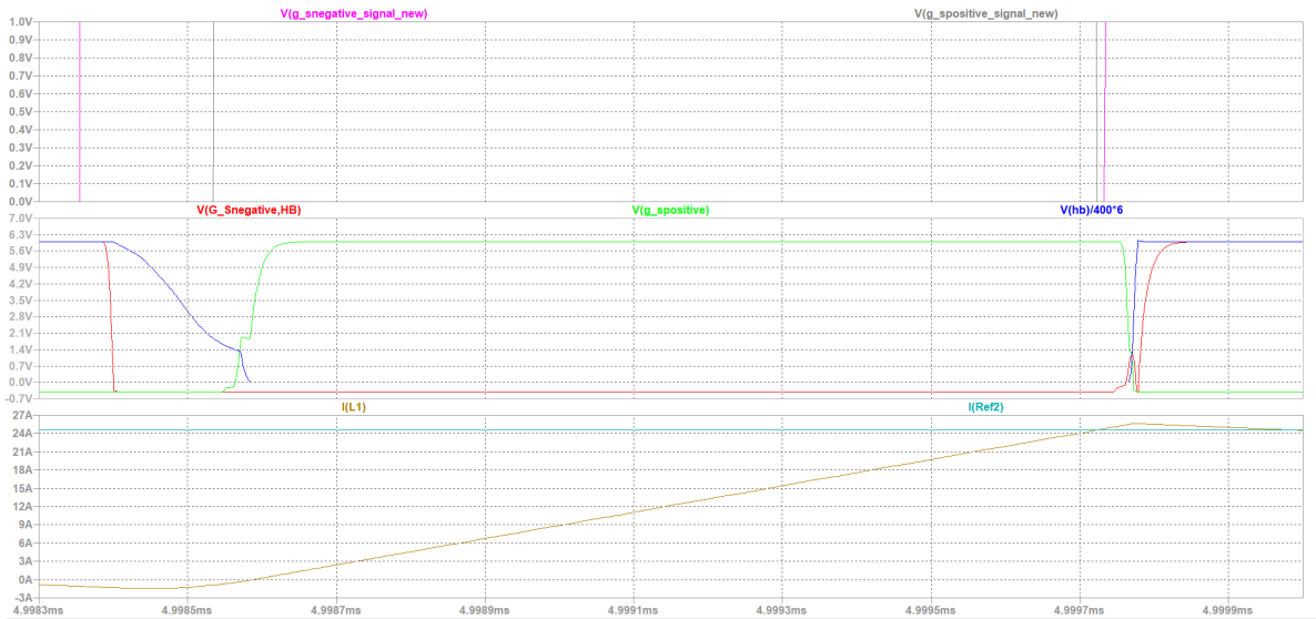
Figure 4.19: Details @5ms, for model with gate driver, 15μH, no margin timing
