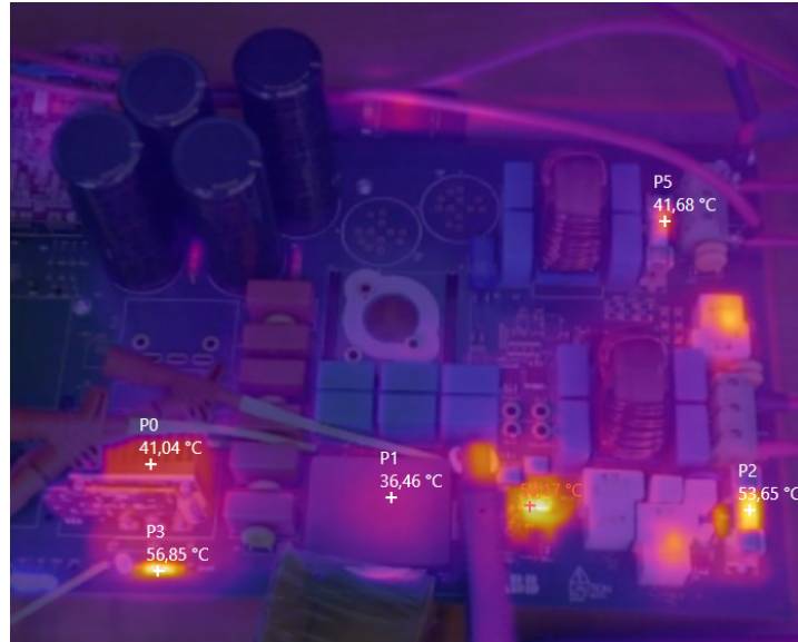
Figure 6.22: Thermal image overall, @ v_{AC} = 300V
