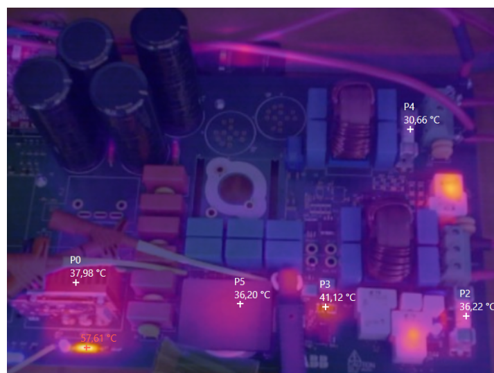
Figure 6.27: Thermal image overall, @ v_{AC} = 200V
