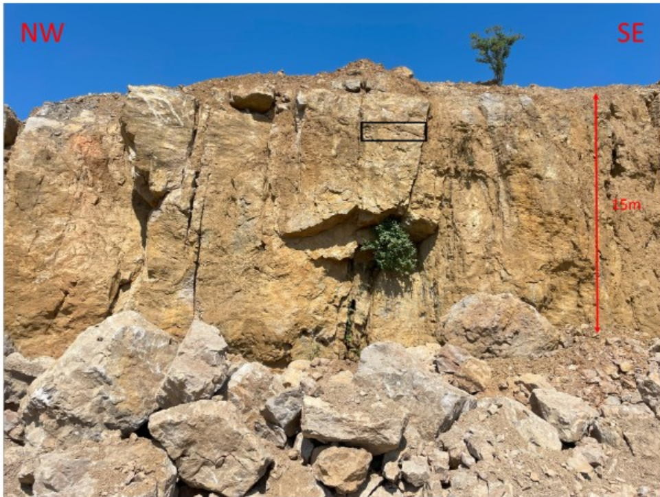
Figure 7.3: Single visible bedding plane (Black box) on a 30 meter wide, 15 meter high outcrop (Bench 2 location without karst).
