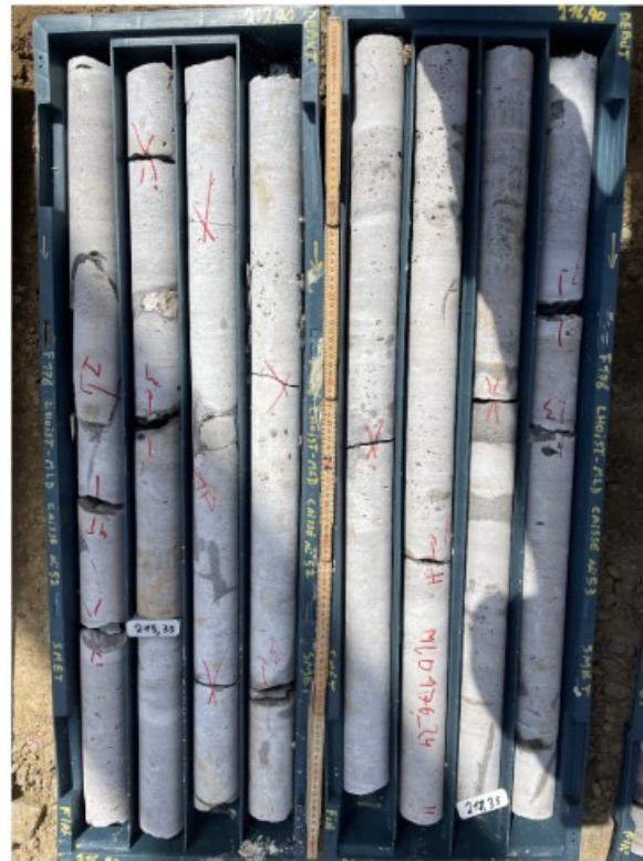
Figure 5.7: Formation C in BH176, bed thickness including all sub-horizontal joints is around 70cm similar to Mathieu (1962) descriptions.
