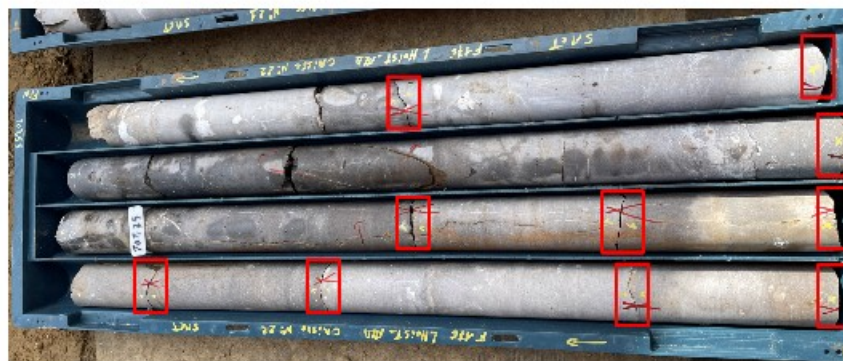
Figure 5.4: Red boxes surround joints originating from hammer blows to retrieve cores from the casing or to fit the rock cores into core boxes. These human induced joints have been marked by the drilling operator.
