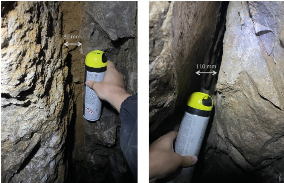
Figure 3.9: Dissolution joints found in the iron shafts near the quarry. Both are found in formation D.
