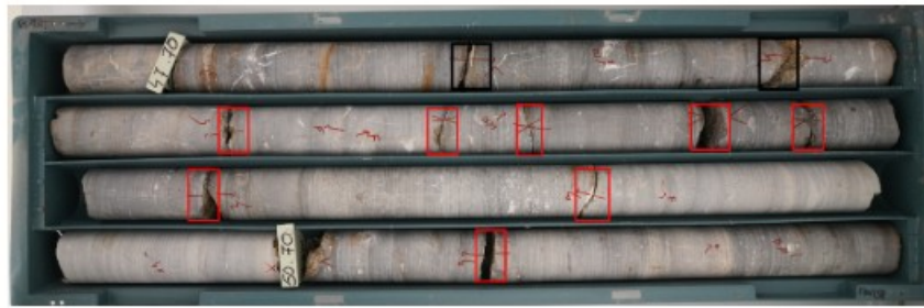
Figure 5.5: Fractures (red boxes) not interpreted on the borehole optic scan in formation E. Some display clear signs of surface staining. Black boxes are joints observed during core descriptions and observed on the optic scan.
