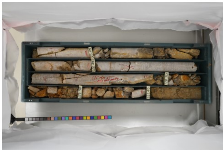
Figure 5.25: Borehole 172 drilled accros karstic voids, between 128.7 and 131.7 only 60cm of cores are recovered on a borehole section 3m long.
