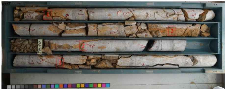
Figure 5.22: 1) joint with no wall contact when sheared, clay infill. 2) Rough planar and rough undulating joints with thin coating of dolomitic sand
