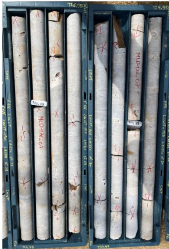
Figure 5.6: Rock core samples indicate bedding thickness at least 1 meter thick for formation D.
