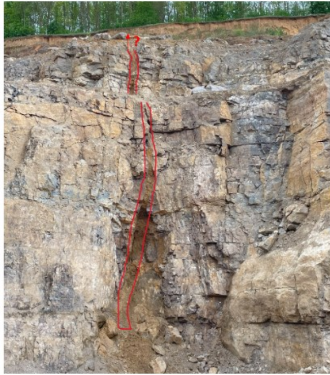
Figure 5.12: Joint at least 30 meters in height on bench 1 and 2. The joint is not observed on bench 0 (bench with overburden removal)
