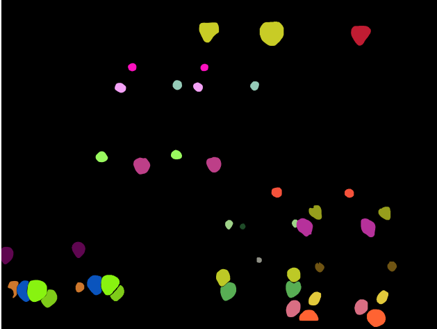
Figure 10. Example of matching of the images of Figure 2. Strawberries appear twice since both the strawberry segments from the RGB and the OCN camera are shown. Segments shown with the same color were matched by our algorithm. When manually evaluating, the matching performance is good on strawberries that are relevant for our size measurements. Proper matching allows us to calculate disparity, depth, and finally the size of a strawberry.
