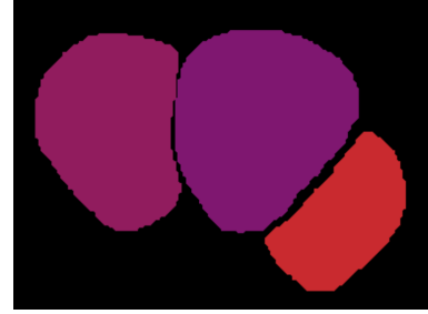
Figure 12. Close up of three strawberry segments on the bottom left of Figure 11. The depth estimation algorithm seems to put occluded segments further away, which indicates good performance locally.
