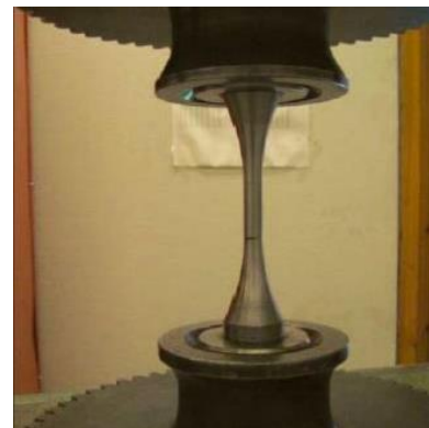
Figure 8: Small scale test specimen during fatigue testing
