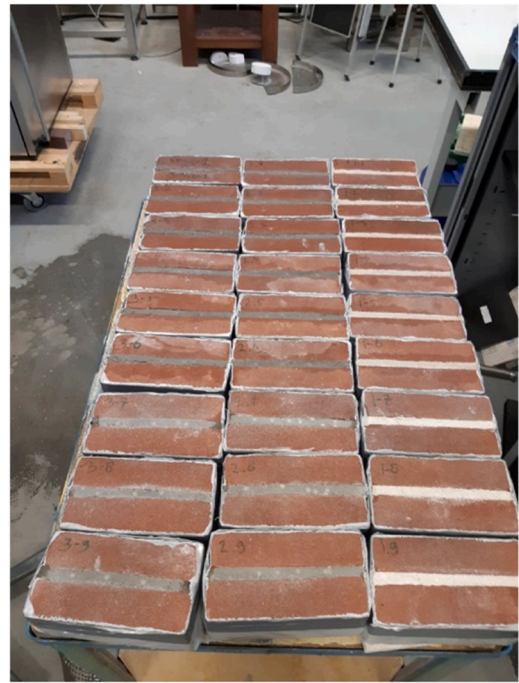
Fig. 1. Example of sealed and pointed test specimens.
