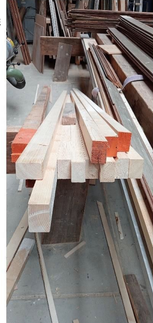
BUNNDLE OF LAMELLA READY FOR LAMINATING
