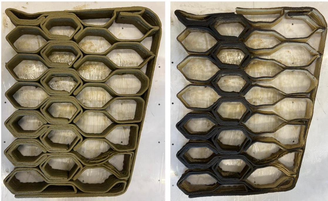
Figure 14. Printed prototype before (left) and after (right) drying.
