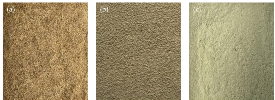
Figure 1. Bamboo material employed for research: (a) bamboo fibers; (b) bamboo powder B; (c) bamboo powder G.
