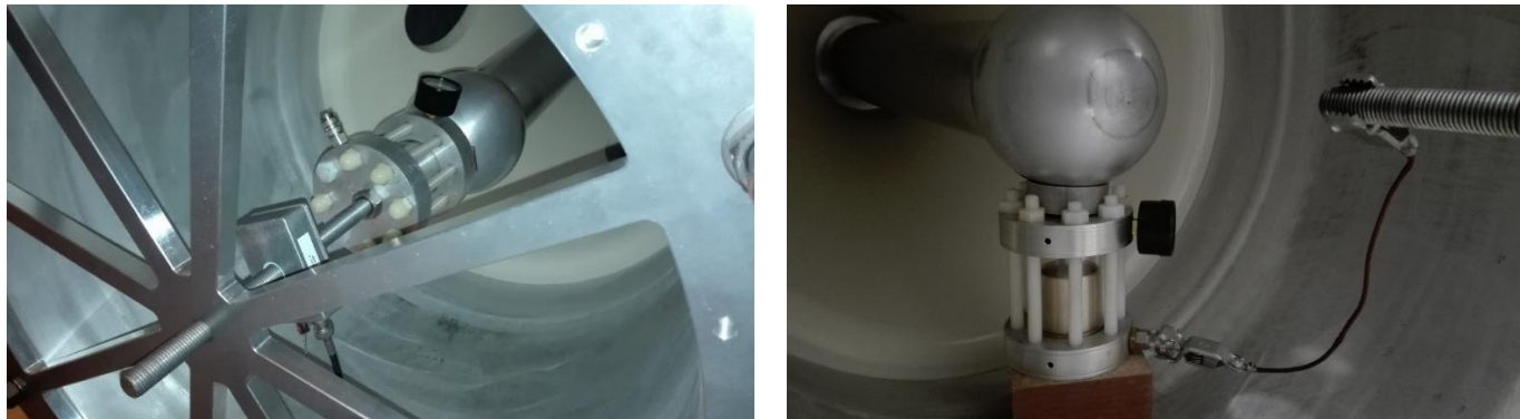
Figure 52. Installation of the test cell in the GIS
