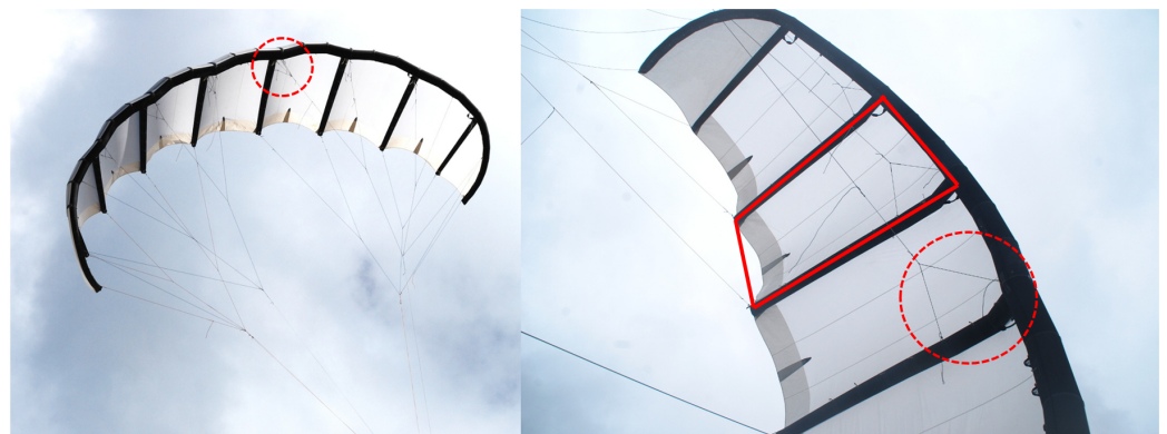
Figure 2. Two photos of the LEI V3 kite in flight: the red quadrilateral indicates the structural model of one of the wing segments, and the red circles indicate Y-splits of the bridle close to the tubes to distribute the transmitted load [25].
