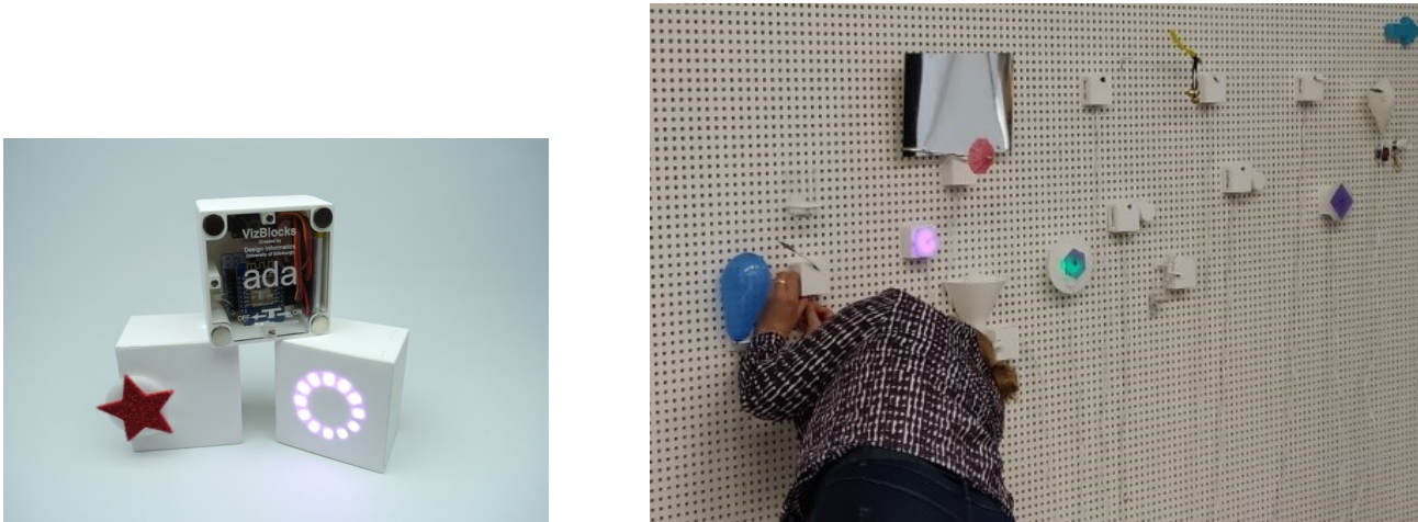
Figure 2: (left) individual VizBlocks blocks, clockwise, including the back of a modular block showcasing its internal electronics, an LED ring block, and a servo-motor block with a craft material star attached. (Right) VizBlocks physicalisations mounted on a paneled wall in the design studio.
