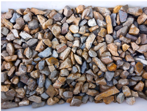
c Clean ballast particles in the reservoir: AREMA
