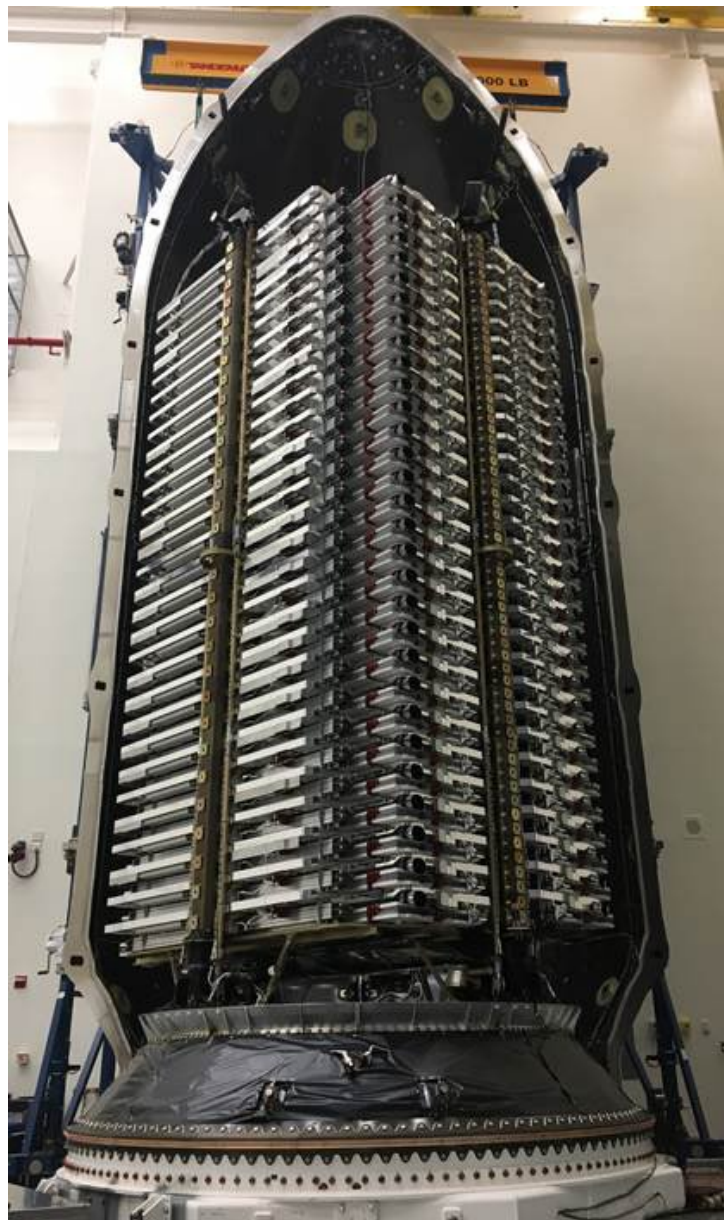
Figure 3.4: Starlink satellites loaded in a Falcon 9 3
