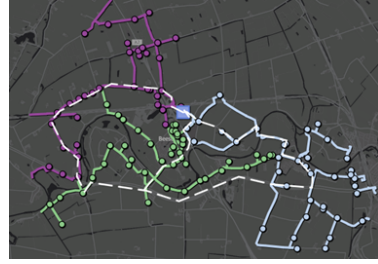
Figure 6: Current grid topology of Beesd (colored lines) and sketch of existing grid expansion plan (white dotted lines).
