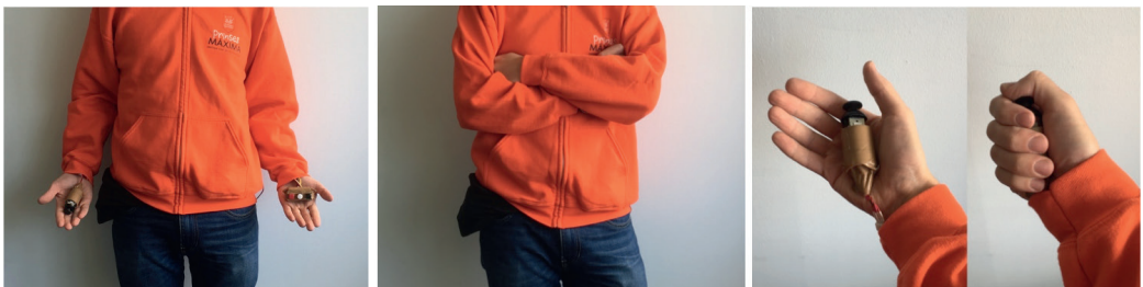
Figure 7 During the fieldwork, Fizzy was controlled with a joystick and buttons that were concealed in the hands and by standing with the arms crossed or behind the back.
