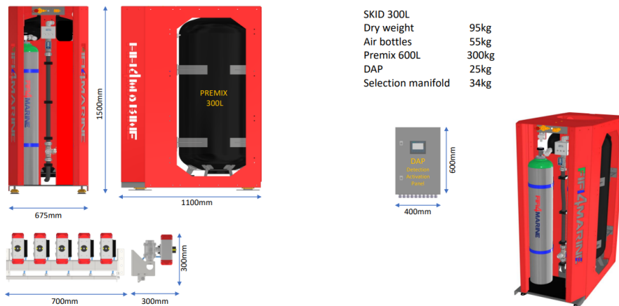
Figure A.2: 300 l firefighting skid from FiFi4Marine (Fifi4Marine, 2022).
