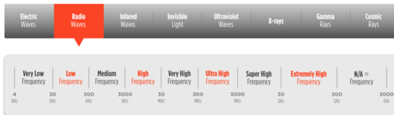
Figure 2.3: Electromagnetic spectrum with radio waves indicated [3]
