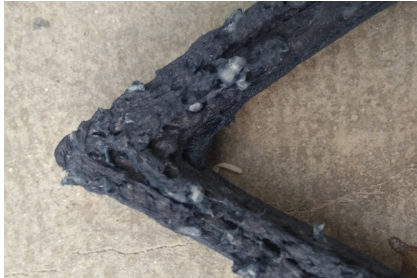
Figure 4.11: Insufficient molten pellets
