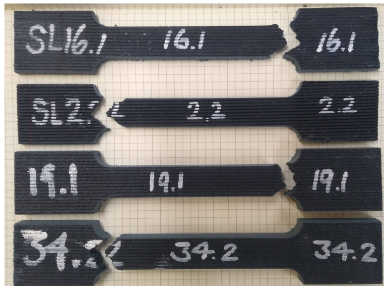
Figure 5.2: Cracked tensile specimens.
