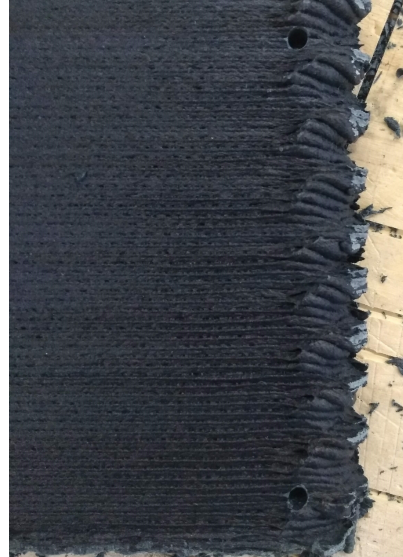
Figure 4.5: Distortion within the printed plate due to the corner.
