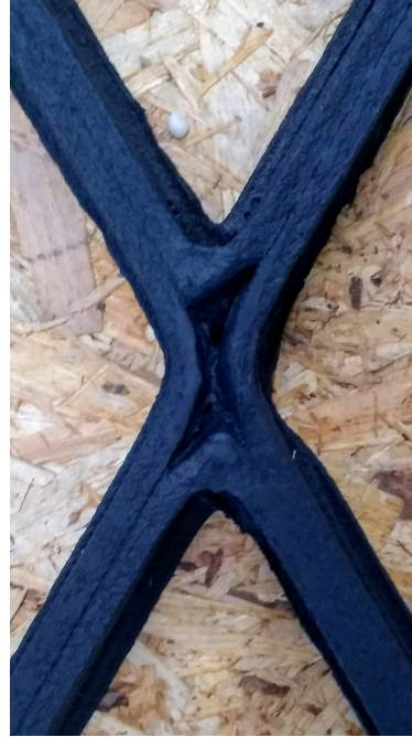
Figure 2.5: Insufficient volumetric flow rate at the joint
