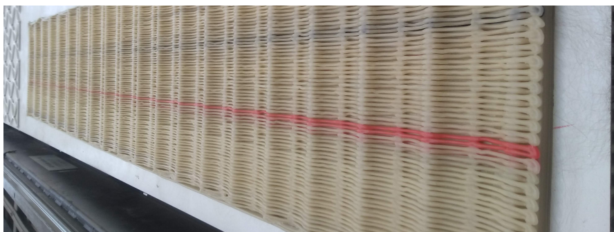
Figure 4.6: The distribution of a single pellet with red colouring agent along the print path of a panel with a surface area of 2.45 x 0.40 m 2 .
