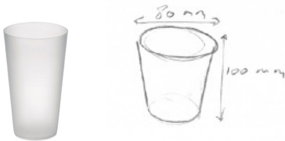
Figure 27: the reusable festival cup as analysed in this paragraph (left) with its measurements (right).
